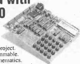
The AES-10... a complete learning system, a complete embedded control system. Extensive manuals guide you through your 8051 development project. Assembly, BASIC, and C programmable. All hardware details, complete schematics. Learn to program the LCD, keypad, digital and analog I/Os. The entire board is software reconfigurable for your applications. Everything you need, nothing extra required.
