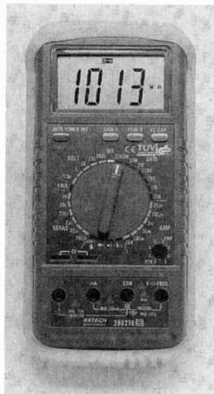
The *Rangemaster II* features 45 ranges and 11 functions that include voltage, current, resistance, frequency, capacitance, and logic, with very wide ranges and high resolution. The range for DC voltage is 200 mV to 1000 volts (0.6% basic accuracy); AC voltage is 200 mV to 750 volts (1.2%); DC/AC current is 20  $\mu$ A to 20 amps (0.8% and 1.2%, respectively); resistance is 200 ohms to 200 megohms (0.8%); capacitance is 2 nF to 200  $\mu$ F (3%); and frequency counter is 2 kHz to 20 MHz (1%).
