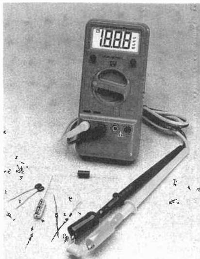
resolution in the 20-ohm range. The meter features a capacitance zero-adjust button to compensate for test-lead and stray capacitance. The 20-ohm range, typically found only in expensive, bench-quality meters, also features the zero-adjust button to compensate for test-lead resistance. The CR50 also includes a beeper for fast and convenient continuity measurement, and a diode test.
