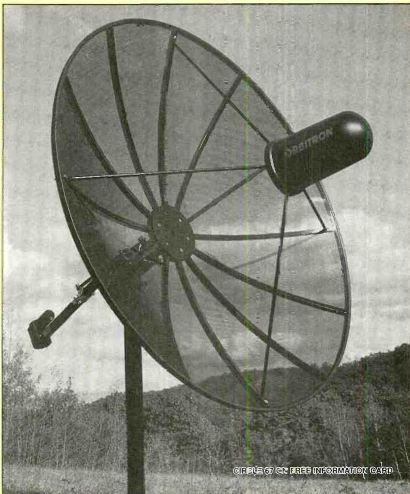
the wind. When we installed the feedhorn, only minor adjustments were required to get the feed to the 31¾-inch focal point of the dish.
