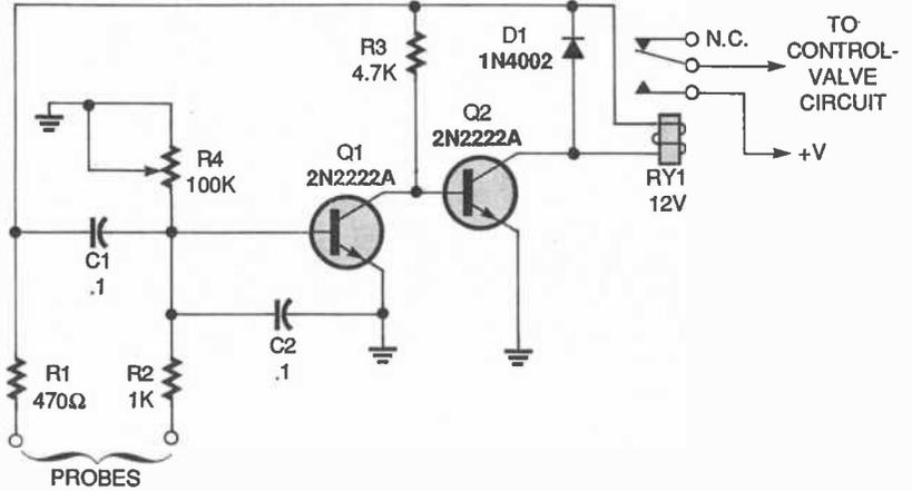
Fig. 3. This circuit builds upon the principles used in the circuit of Fig. 1 to provide automatic operation of a watering system when a dry-soil condition is detected.
