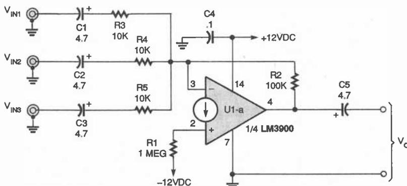
Fig. 10. This CDA-based audio mixer will take the signals from up to three channels and combine them into one channel. Once again, it is built around the LM3900.
