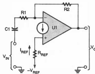
Fig. 4. Here a CDA is used much like an op-amp in an inverting follower circuit.
