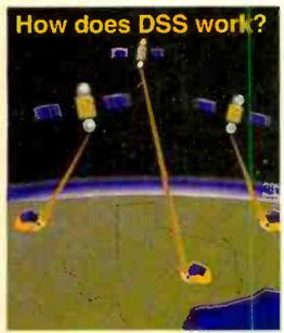
**Three satellites.** There are three satellites located 22,300 miles above Texas. The satellites receive program information from two uplink centers that then beam the signals down to your RCA DSS dish!
