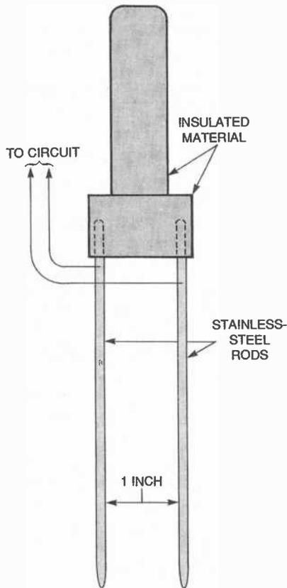
Fig. 2. This probe assembly can be used with the circuit in Fig. 1, as well as other circuits in this month's column. While some dimensions are specified, they are not critical so feel free to use whatever is handy.
