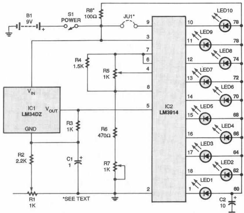
*Fig. 1. Here's the schematic for the LED Thermometer. An LM34DZ temperature sensor, IC1, outputs a voltage that changes with temperature. The circuit interprets that output and displays the temperature in two-degree steps using LED1 through LED10.*
