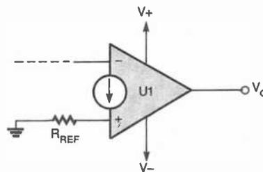
Fig. 7. Though intended for use in single-ended-supply applications, the CDA can be configured for use with a bipolar supply.
