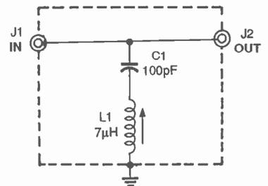
Fig. 4. If your receiver is "desensitized" by the converter's local oscillator, this 6.000-MHz wavetraps could help minimize the problem.
