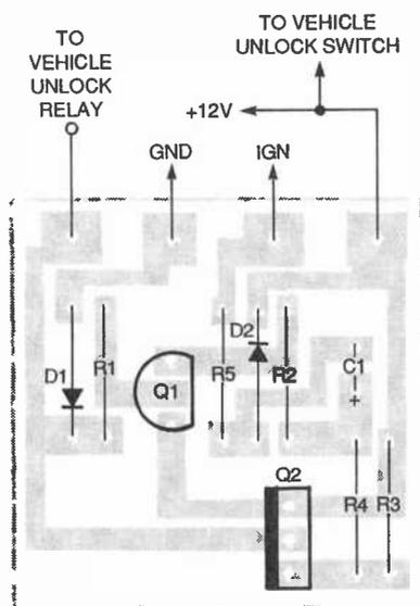
Fig. 3. When building the Unlock-Too on a PC board, use this parts-placement diagram as a guide.
