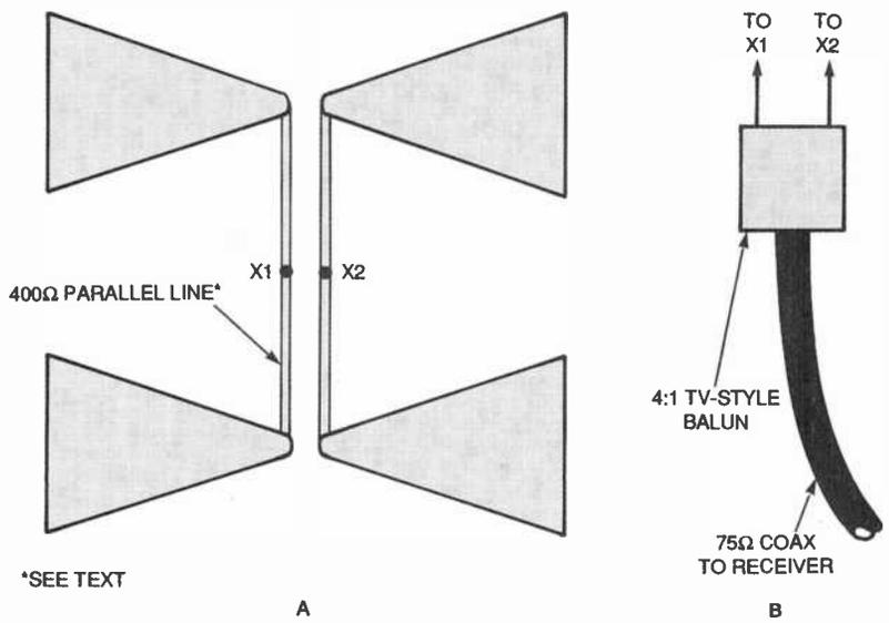
Fig. 9. The two bow-tie dipoles are connected together by a 400-ohm transmission-line harness (A). To use coax to connect to your rig, again use a 4:1 BALUN transformer.
