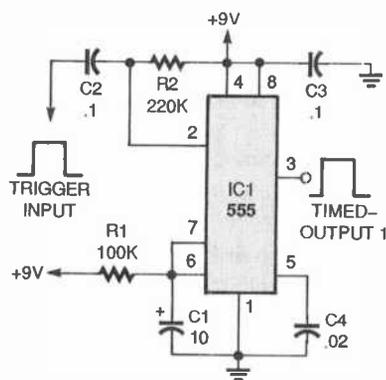
Fig. 1. This simple timer is based on a 555, which is the most well-known IC suitable for this application.
