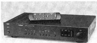
By pressing the LLC button on either the remote control or front panel, the LLC circuit corrects all channels when volume markings fall below 12 o'clock on the level. The LLC circuit adjusts each channel progressively in both amplitude and frequency, so there is no loss of the Dolby sound field when volume is reduced.
