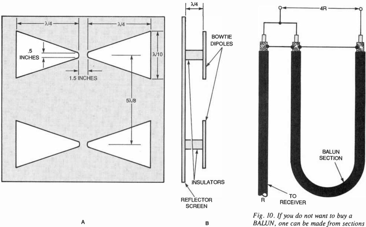
Fig. 8. The "Bow-Tie" reflector antenna, so popular for use in receiving UHF TV signals, can also be used to receive UHF radio signals. A front view of the antenna is shown in A, and a side view in B.
