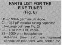
Inductor L2 gives a DC-signal return path for D1's output. The inductance of L2 is too large to affect the circuit's tuning function. This is a very fine crystal radio receiver. Build it, fine tune it, and you'll agree.
