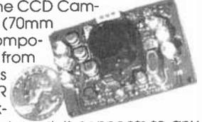
**Power Supply Regulating Kit for CA-H34** This simple kit is designed to fit onto the back of the CA-H34 CCD camera. It resolves the problem of hooking up the camera to an UNREGULATED supply (which damages the camera) by providing safe regulated power from any 12V-14V DC supply. It also provides regulated 12V DC from a 12V AC source.
