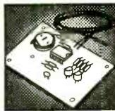
Ever lost frozen food because your freezer stopped? The TC-2 kit would have saved you money. An alarm activates when the temperature reaches a critical point. Turn ceiling fans on automatically when it gets too hot. This kit gives you 100mA of output. SIZE: 2" x 1.4" Power requirement 6 to 15V DC.
