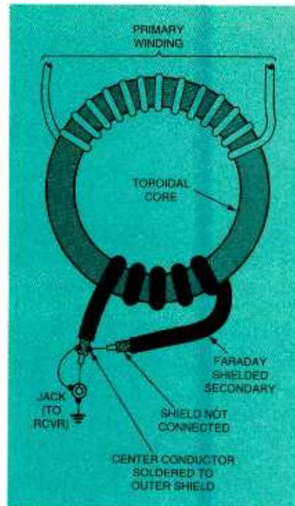
Fig. 7. Use of coaxial cable to form a Faraday-shielded transformer.
