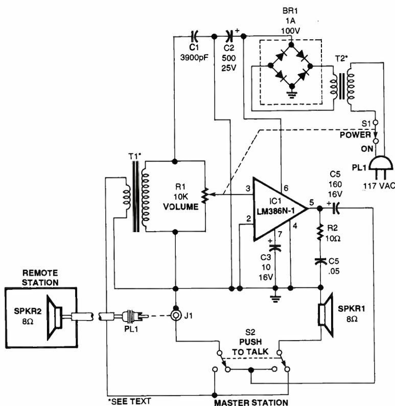
Fig. 1. This simple intercom system can be used in a number of household functions when you want to monitor, or converse with, another location.
