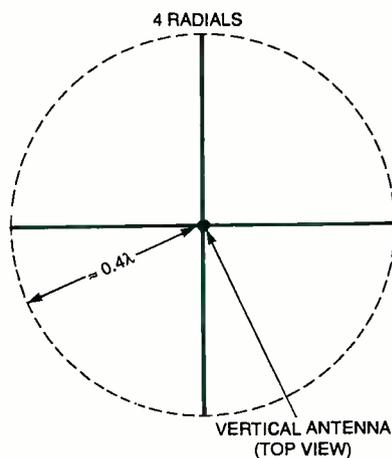
Fig. 3. Four-radial system.
