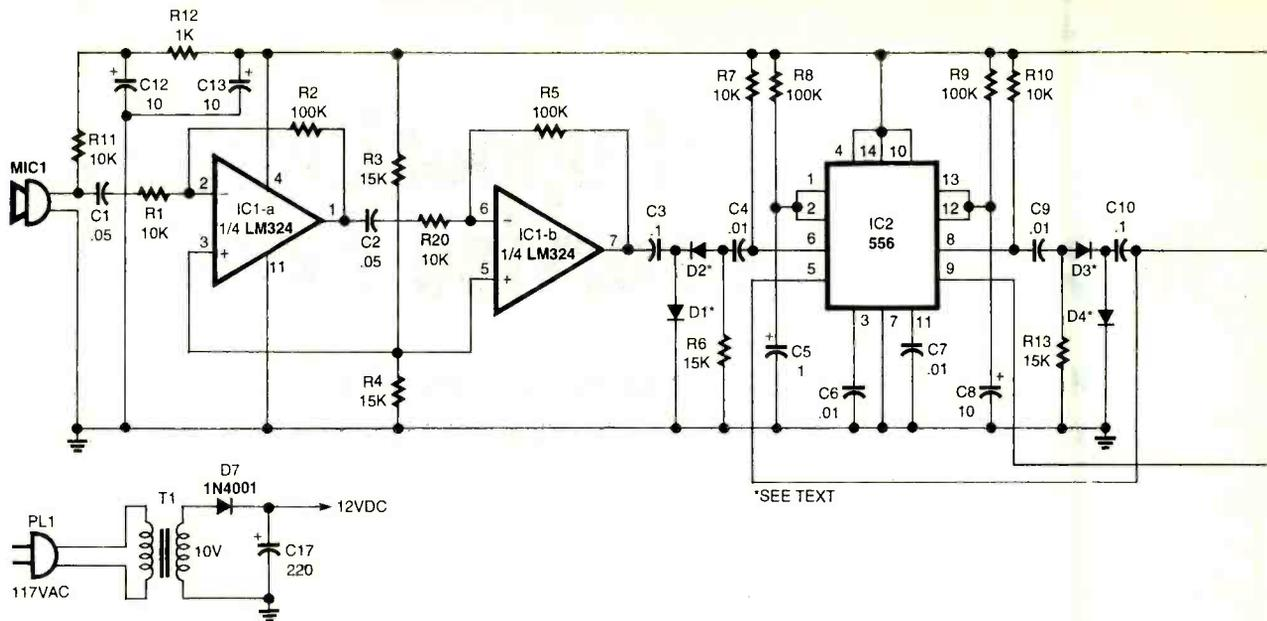
Fig. 3. Here's another amazing circuit. The two output relays can control a number of electronic devices. Just a clap of your hands twice, or almost any other quick double sound within a one second interval will activate operation.
