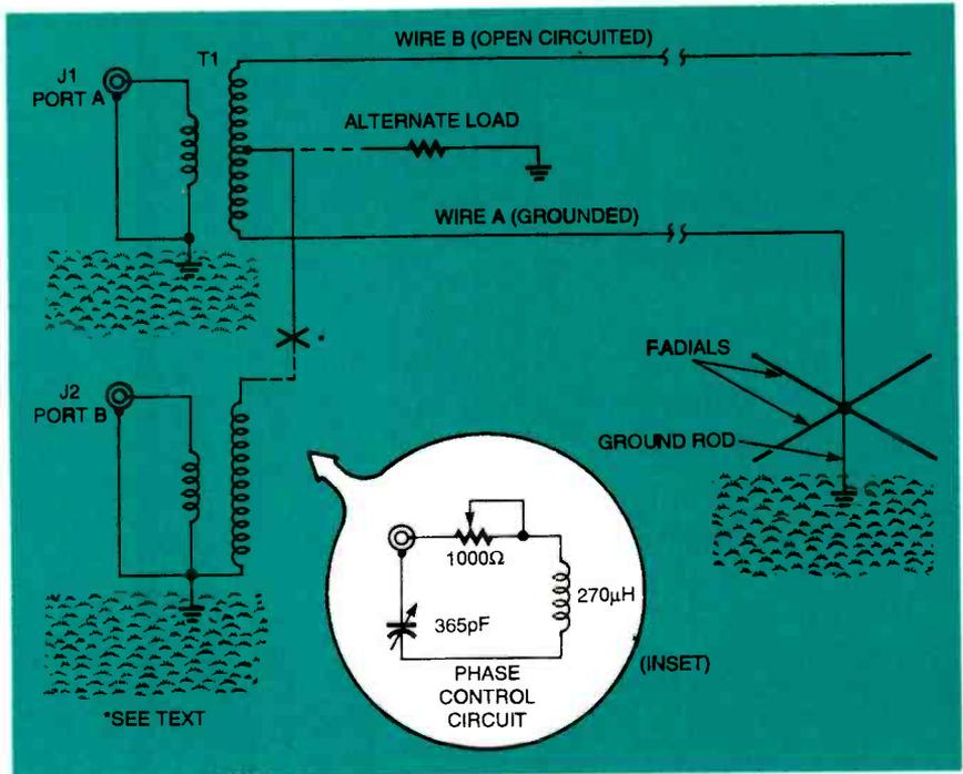
Fig. 10. Steerable-notch Beverage antenna.
