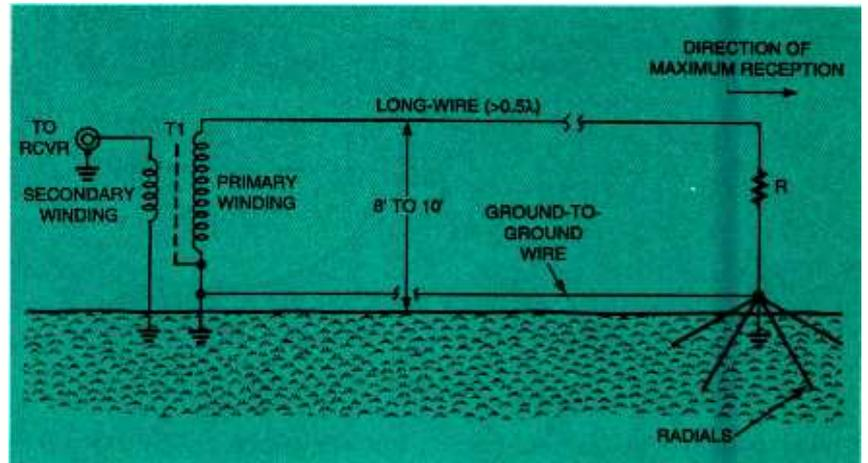
Fig. 4. Use of a ground-to-ground wire and radials to improve Beverage performance.
