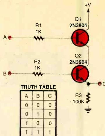
Fig. 3. Two or more switching circuits can be combined to form basic logic building blocks. Here a pair of switching transistors (setup in a buffer configuration) is used to form an AND gate.
