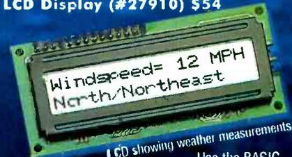
Use the BASIC Stamp's SEROUT instruction (recurses one I/O line, ground and power) to communicate with the Serial LCD display.
