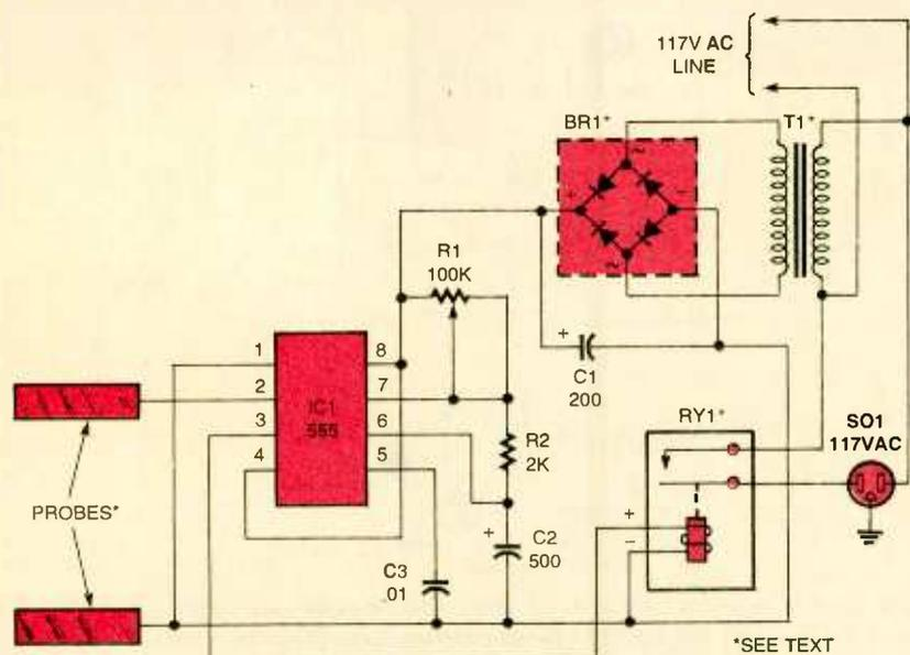
Fig. 4. This neat circuit is used as an AC controller for a water pump inserted into power outlet SO1; however, any device, which depends upon probes in a conducting medium to work, can be used in its place.
