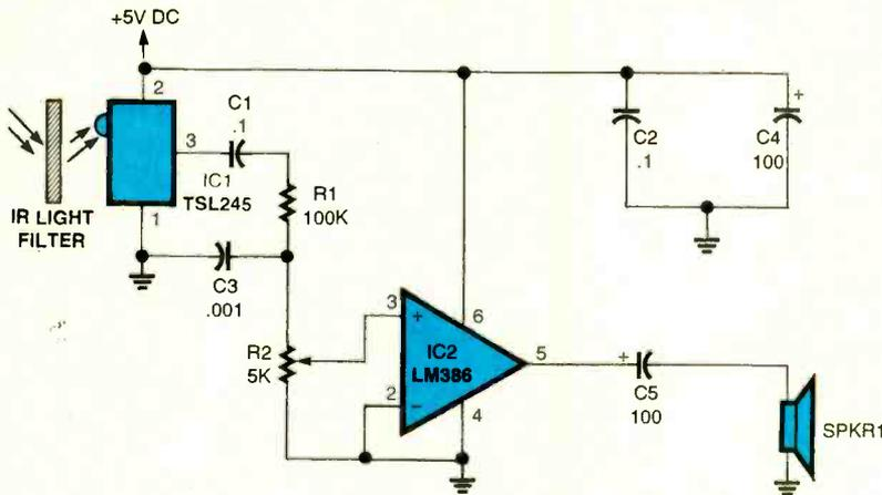
Fig. 3. This fun-circuit produces an audio output whose pitch is proportional to the light falling upon IC1.
