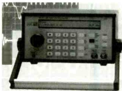
skipped points. It provides function, arbitrary waveform, and pulse-generation capabilities.
