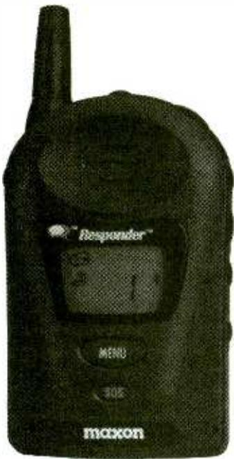
groups of users, directly from the handset. As many as 25 voice messages and/or memos can be stored in the Responder. The device is also capable of placing a live telephone call to an emergency service number or to a limited list of key personal numbers.
