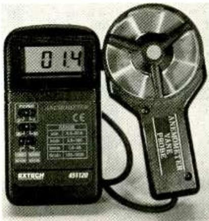
Measurements range from 160 to 5900 ft./min, 1.6 to 58 knots, 0.8 to 30 m/sec, and 2.8 to 108 km/hr. The low-friction, ball-bearing, twisted-arm vane structure ensures precise low and high readings.
