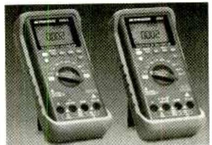
The meters provide two user-selectable operating resolutions (4000/40,000 counts), voltage to 1000 VDC/750 VAC, current to 10A, a dual-display offering frequency to 200 kHz with AC signal measurement, resistance to 40 megohms, capacitance to 9999 µF, and diode check and continuity. These instruments feature data hold, relative mode, and MAX/MIN/AVG of inputs with an elapsed timer counting the time to the event.
