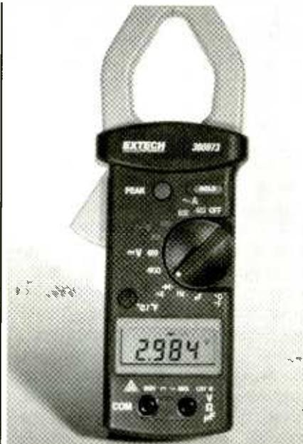
Peak (Maximum) Hold, and there are indications for over range and low battery. Measurements are displayed on a 3 1/2-digit (3999 count) LCD. The unit, whose jaws open to 1.6 inches, measures 9 x 3 x 1.5 inches. It comes complete with test leads, a bead wire temperature probe, nine-volt battery, and case.
