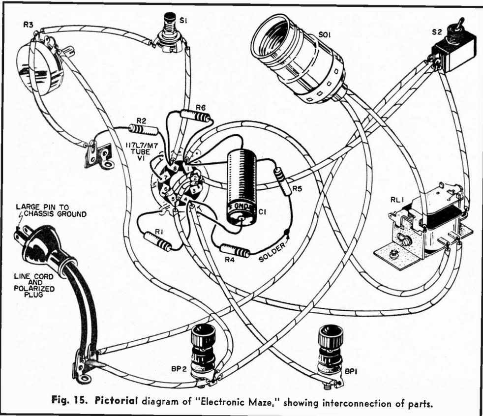
Fig. 15. Pictorial diagram of "Electronic Maze," showing interconnection of parts.
