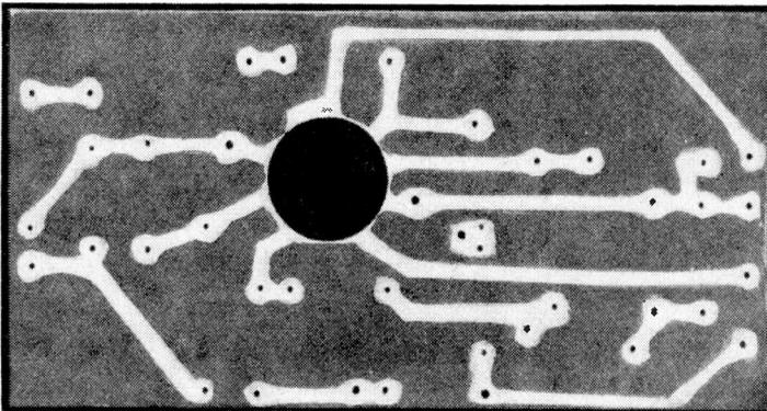
Fig. 2. The etched board, drilled and cleaned, and ready for mounting socket and component parts. Mounting holes for the electrolytic capacitors may have to be enlarged somewhat.
