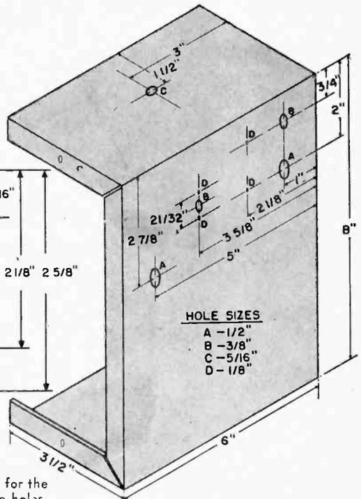
Fig. 2. Cover of the "Minibox" used for the transmitter showing the position of the holes.
