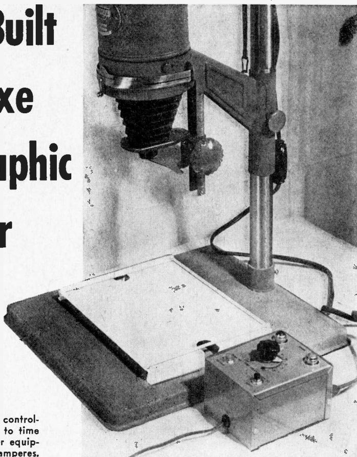
**Fig. 1.** The timer, shown here controlling an enlarger, can be used to time "on" or "off" intervals of other equipment drawing as much as five amperes.
