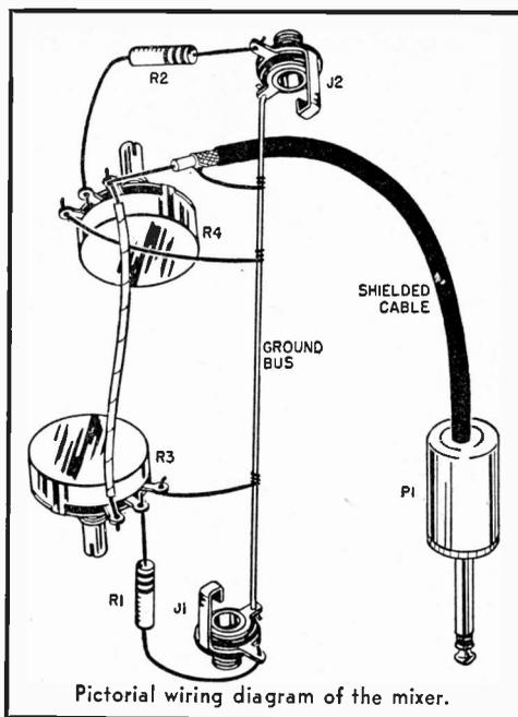
**Underchassis view** of mixer (above, left). Exact position of the two potentiometers is not critical. The author's potentiometers are equally spaced along one side with the input jacks at the ends. The cable to the recorder passes through a grommet in the side of the box. Use the proper plug for the tape recorder or amplifier at the end of this cable.
