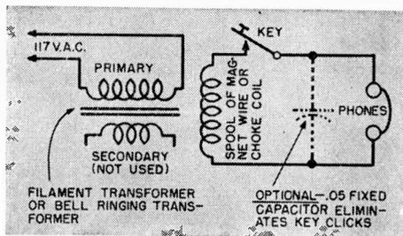
The simple code practice oscillator which can be built from surplus or junk box parts.
