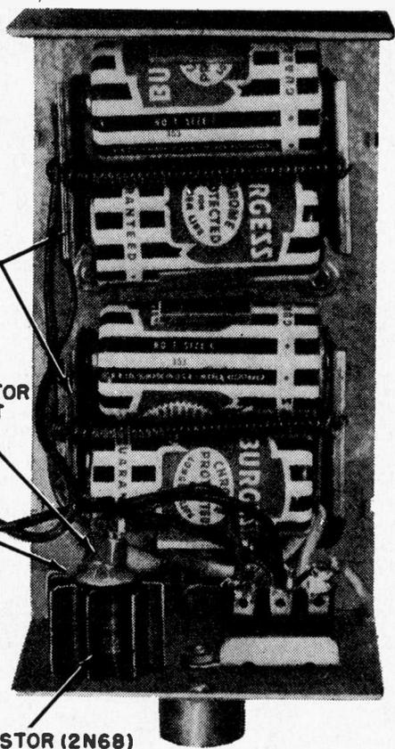
2N68. If desired, *n-p-n* junction type 2N102 may be used in place of the 2N68, *provided the battery polarity is reversed* as well as the leads to capacitor C1.
