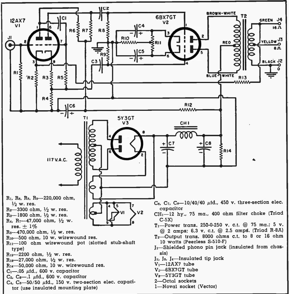
**Fig. 3. Complete schematic** of the 4-watt amplifier. It may be operated from most tuners and preamplifiers and provides adequate output for ordinary home listening.
