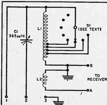
$C_1$ —365- $\mu$ fd. broadcast-type variable capacitor
