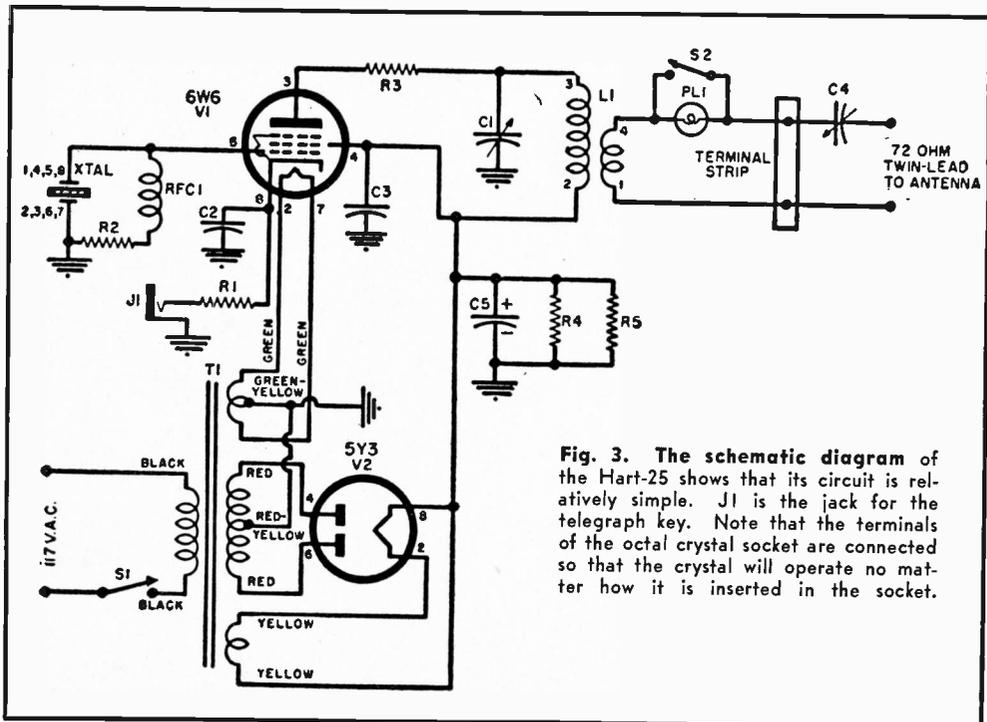
Fig. 3. The schematic diagram of the Hart-25 shows that its circuit is relatively simple. *J1* is the jack for the telegraph key. Note that the terminals of the octal crystal socket are connected so that the crystal will operate no matter how it is inserted in the socket.
