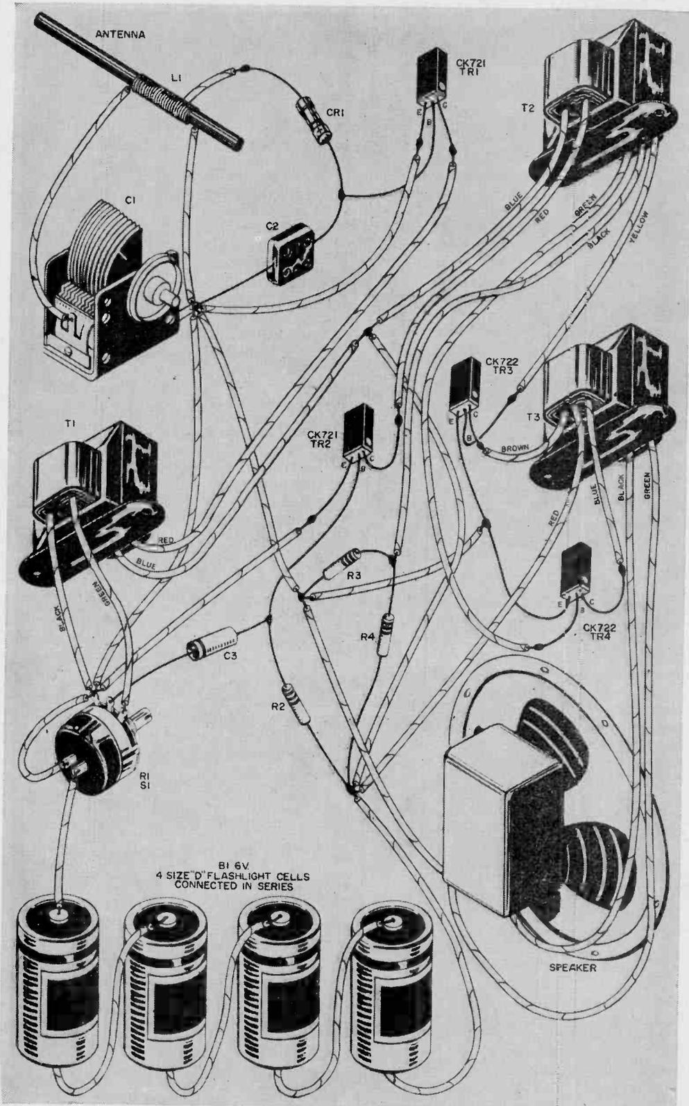
Pictorial diagram (on opposite page) and parts list (below) for the complete transistorized receiver.
