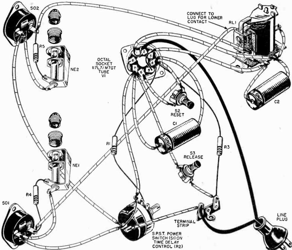
**Fig. 6.** The timer is shown here with the wiring and assembly completed, but before the two parts of the cabinet are assembled. Note the position of the sub-chassis and parts layout. The layout is not critical but it is best to keep it neat and compact.
