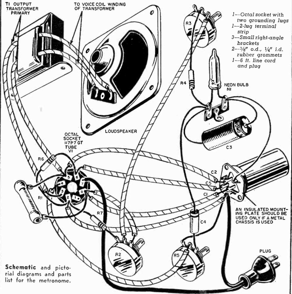
**Schematic** and pictorial diagrams and parts list for the metronome.
