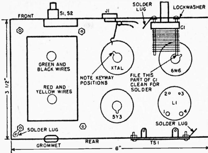
Fig. 1. This bottom view of the chassis shows the placement and orientation of the most important parts of the transmitter.
