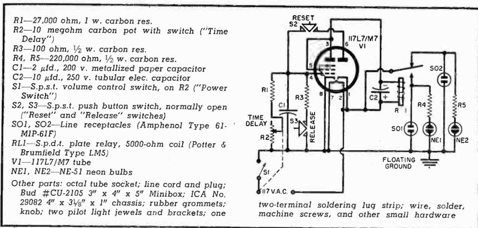
Fig. 4. Here are the schematic diagram and parts list for the home-built timer.
