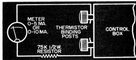
Fig. 5. Hookup for initial adjustments.
