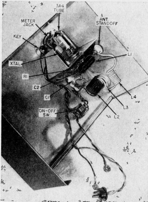
**Back view** of the transmitter without the batteries, showing location of the various parts.
