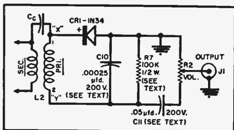
Fig. 2. Partial schematic of non-powered unit.
