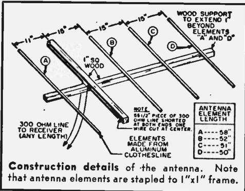
**Construction details** of the antenna. Note that antenna elements are stapled to 1"x1" frame.
