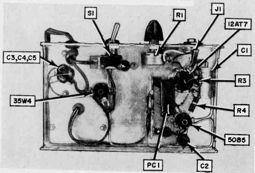
Fig. 3. Below-chassis view of the wired unit. Parts are identified.
