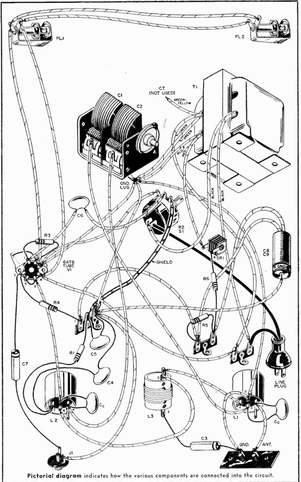
Pictorial diagram indicates how the various components are connected into the circuit.
