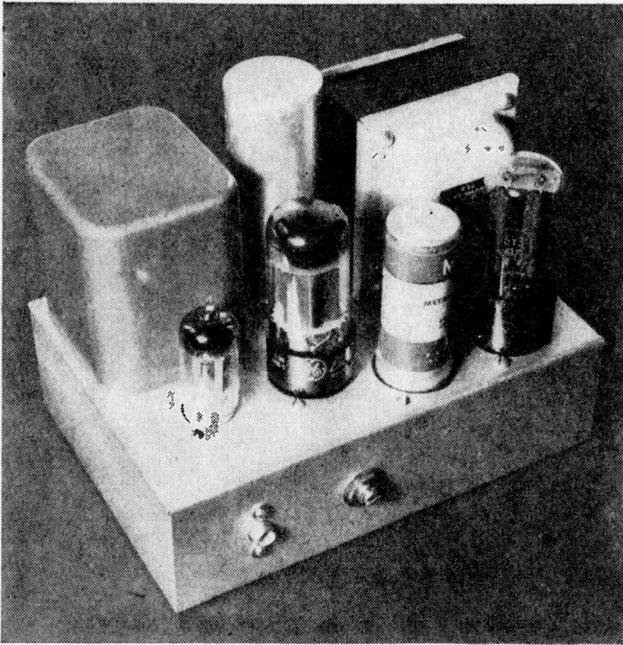
Fig. 1. Home-built amplifier measuring 5" x 7" x 2".
