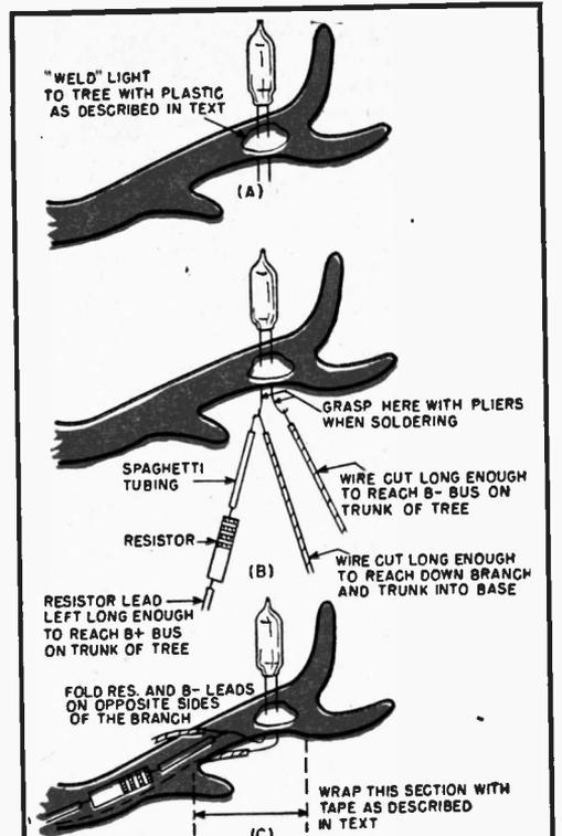
Fig. 2. Method of mounting and wiring neon lamps on individual branches. (A) Using plastic to "weld" light to branch. (B) Fastening resistors and leads to base of lamp. (C) Placement and taping of the wiring used in construction.
