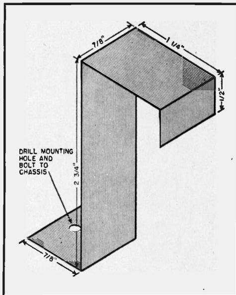
**Fig. 3.** Bracket for holding the B battery. This part may be made from copper, brass or aluminum.
