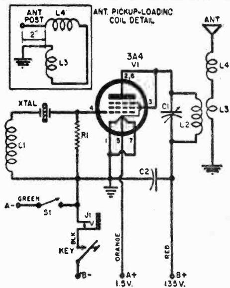
**Fig. 3. Schematic diagram** and parts list for the complete R/C transmitter. The pictorial diagram below shows the way the antenna pickup and loading coils are positioned.
