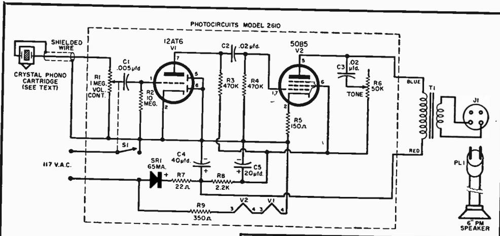
C1\*—0.005- $\mu$ fd. disc ceramic capacitor
