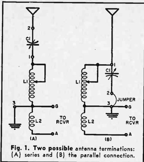
**Fig. 1. Two possible antenna terminations:**
