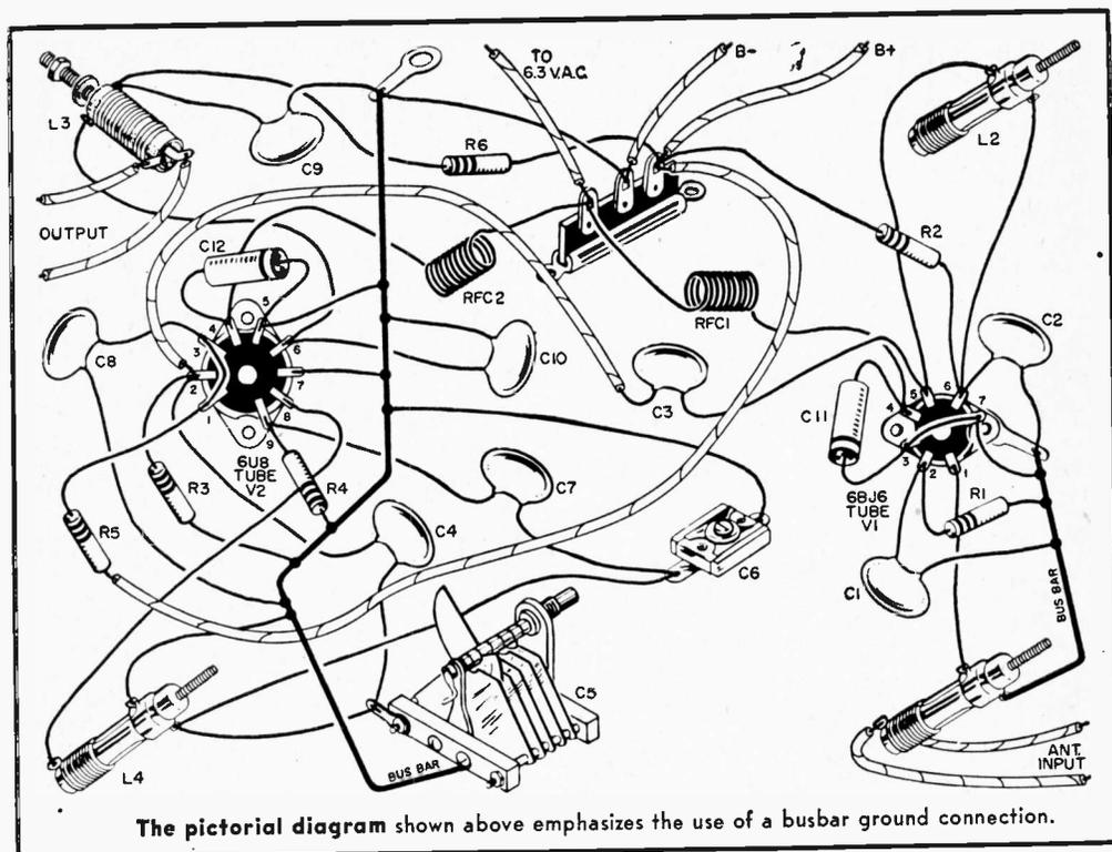
and  $L3$  to 4000 kc. Apply voltage to the tuner and check with the grid dip oscillator to see that the oscillator circuit is oscillating at 45 mc. Final tuning can be completed on received signals.
