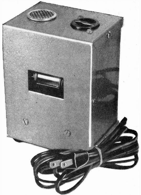
**Y**OU won't have to worry about coming home to a dark house at night if you build an automatic light switch like the one described here. When a table or floor lamp is plugged into its receptacle, it will automatically turn the lamp on at night and off during the day.
