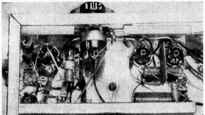
**Fig. 8.** Under chassis view of the completely wired radio. →
