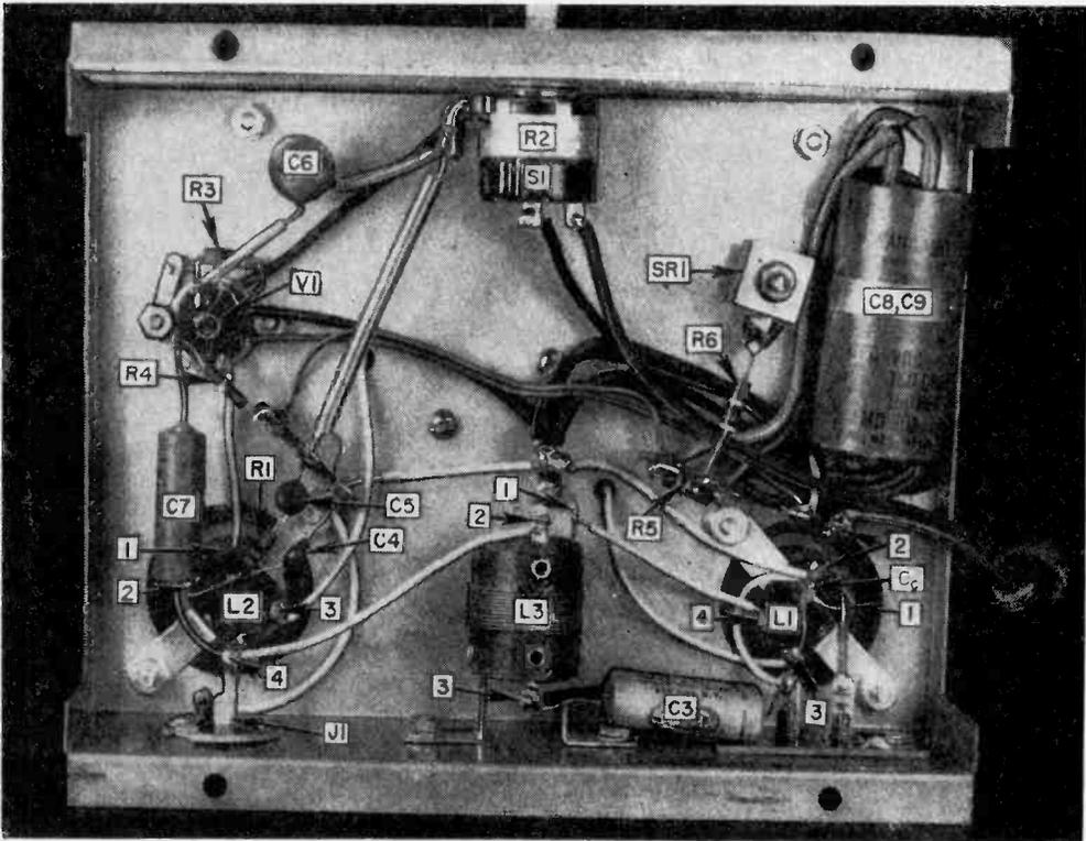
**Fig. 4. Rear view of powered version.** The power transformer *T1* is located above the chassis, while the remainder of the power supply components are mounted below the chassis. See Fig. 3.
