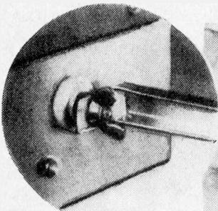
A detail view of mounting of one control antenna to its feed-through insulator.
