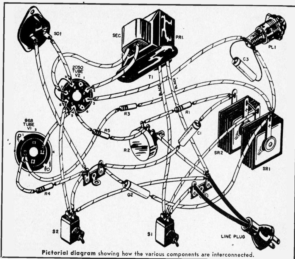
Pictorial diagram showing how the various components are interconnected.
