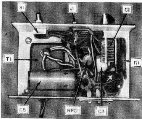
**Fig. 5. Bottom view of the Hart-25 chassis.** Most of the major components are visible, except the socket for V1, the 6W6GT, which is hidden by the variable tuning capacitor, C1.
