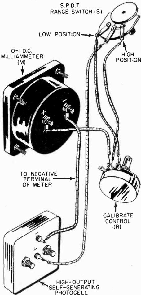
A LIGHT meter is invaluable for measuring illumination levels in the home, office, or factory—and outdoors as well as indoors. It can be used, with proper calibration, as a photographic exposure meter and also in conjunction with enlargers and printing boxes in the darkroom.
