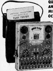
QUICKLY AND EFFICIENTLY TESTS RADIO AND TV TUBES INCLUDING: SEVEN PIN MINIATURES; EIGHT PIN SUBMINARS, OCTALS AND LOCALTS; NINE PIN NOVALS
