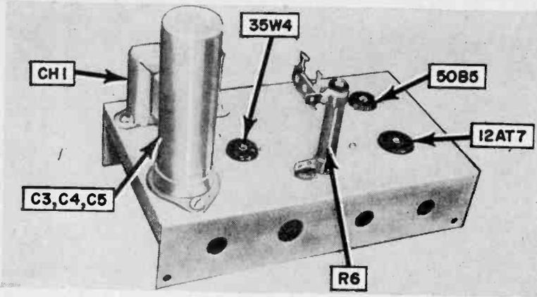
Fig. 2. Above-chassis view of amplifier (at left). Some parts are mounted but not wired.
