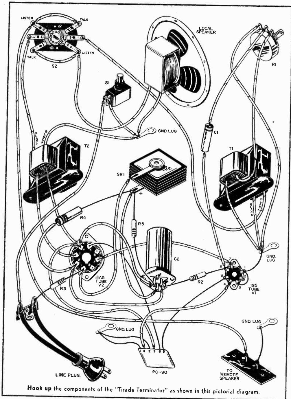
particularly critical. However, delicate filaments combined with high-gain amplifiers are subject to 60-cycle hum unless carefully handled. If the hum is excessive, it usually means one of three things: poor grounds, defective filament filtering capacitor (C2c), or extra long 1A5 grid leads.
