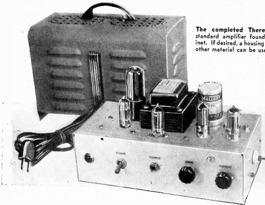
The completed Theremin in a standard amplifier foundation cabinet. If desired, a housing of wood or other material can be used instead.
