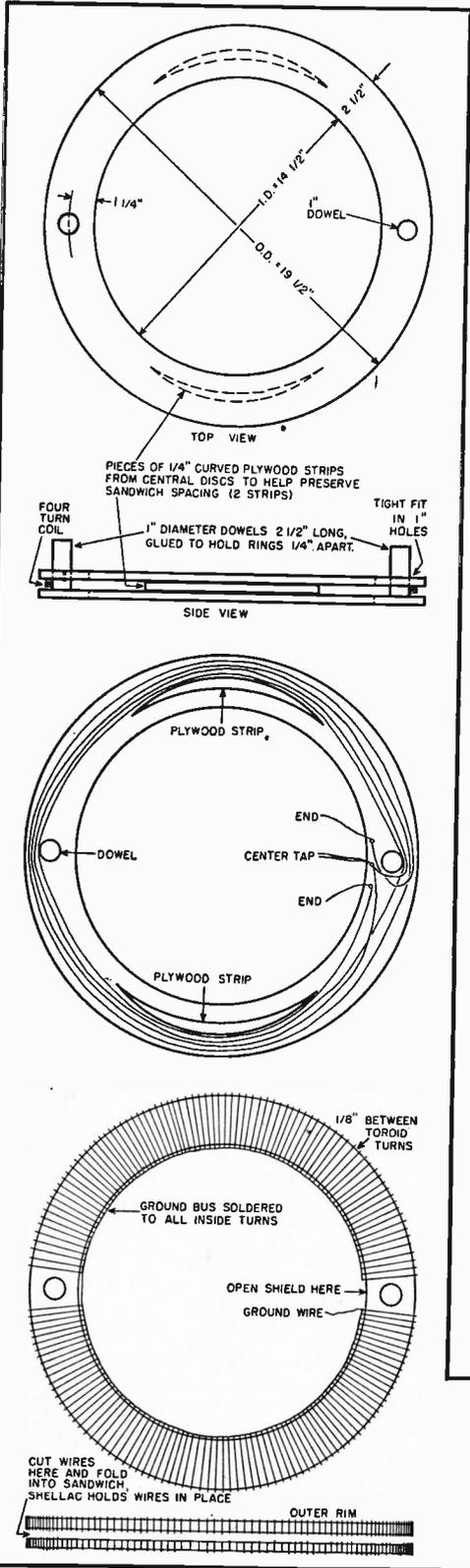
**Construction details** of the loop. Top drawings show top and side views of wooden frame. Center drawing indicates how windings are placed on the frame, and bottom sketches give detailed information on the construction of the Faraday shield.
