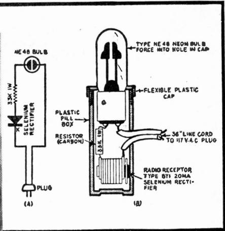
Fig. 4. Proper way to use the 60-cycle stroboscope diagrammed above. Technicians and audiophiles will find this handy for checking the speed of their phonograph turntables.
