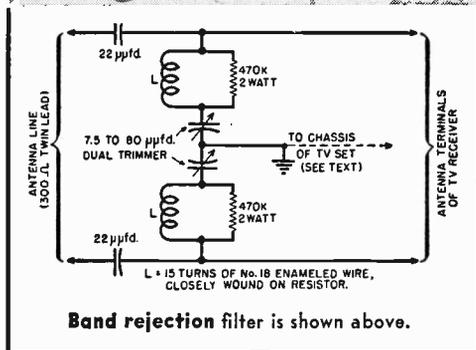
resistors is to serve as simple, inexpensive coil forms. Any style of capacitor can be used, except the paper tubular type. This type has some inductance at the higher TV channel frequencies.
