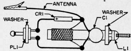
Pictorial diagram of the tuning unit (above). This assembly mounts inside of a plastic tube.
