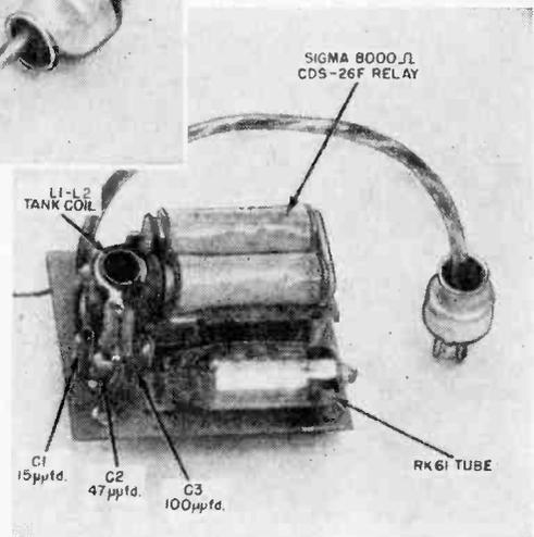
*Sigma 26F* relay. A slightly larger *Sigma* relay, the 10,000-ohm 5F, will also work fine, but due to its larger size and weight, a new chassis layout would have to be made.
