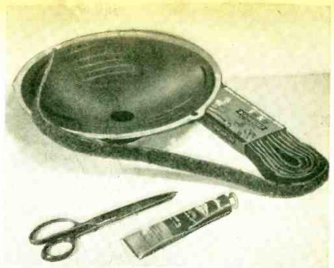
If the woofer doesn't have a cardboard spacer ring, you can cement felt weatherstripping around the rim (see the photograph above) as a substitute.
