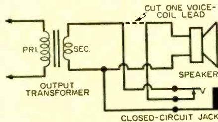
How the pillow speaker jack is wired into the voice-coil circuit of the bedside radio.
