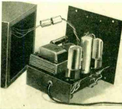
Components are mounted as shown here. Miniature cable connectors which join the four leads that go to strobtron socket on top of case make it simple to remove chassis for inspection or repairs.
