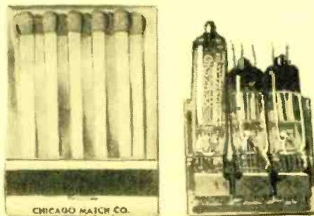
Printed-circuit plate with three sub-miniature tubes installed is smaller in size than book of matches. Unit is a complete three-stage audio amplifier excluding only power supply and volume control.
