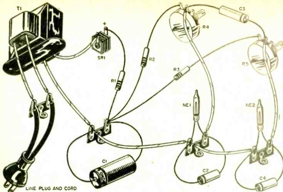
**Pictorial and schematic diagrams** for the darkroom timer. Since the circuit is not critical, other parts may be substituted for those given below in certain cases (see text).
