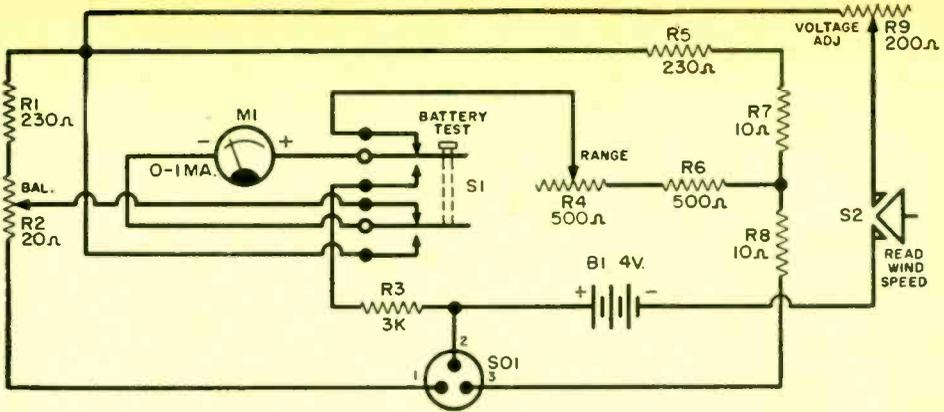
**Diagrams** and parts list for the electronic anemometer. The circuit above is contained in the control box; the thermistors diagrammed on the right are placed on a separate base and located out in the open. A three-wire cable connects the thermistor assembly to the control box containing the meter. Pictorial diagram showing method of connecting parts is at the left.
