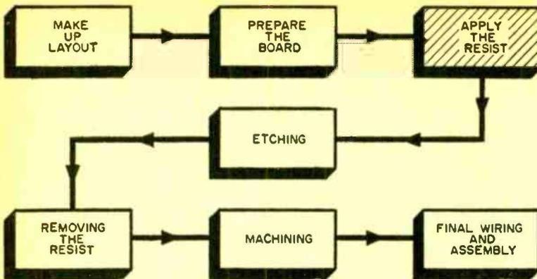
Basic steps in the preparation of an etched circuit. It is in the step labeled "APPLY THE RESIST" that simplified techniques can be used and time saved.
