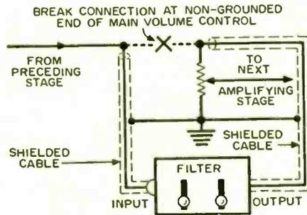
Filter may be used with "single-chassis" amplifier by tapping into amplifier's own circuit as shown in above schematic. Note use of shielded cable for carrying the audio signal.
