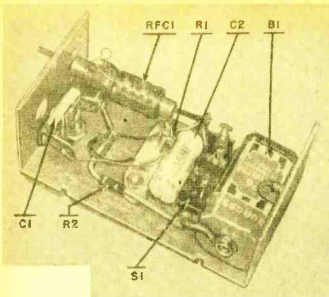
**Open-chassis** view of the transistorized calibrator shows wiring details clearly. Only standard, readily available components are used. The major parts are identified here, but neither the circuit nor chassis layout is critical. Be sure to mount the battery securely.
