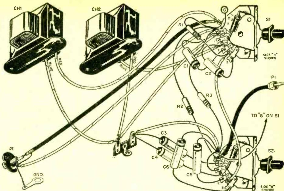
**Pictorial diagram** above details relationship of parts used in the filter. Note that leads on chokes CH1 and CH2 are colored, and must be wired according to instructions. Below are the schematic diagram, table of frequency cutoff action for different switch settings, and parts list. Switches are shown at 100-cps and 4000-cps cutoff points, including shield of output cable, should be returned to connection at ground on J1.
