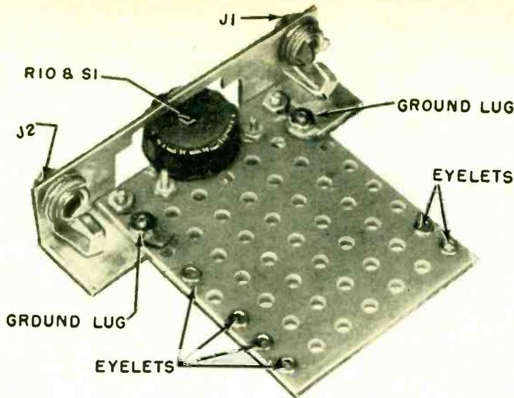
**Preliminary** assembly of the Bakelite mounting board, "frame" for input (J1) and output (J2) jacks, gain control (R10) and the power switch (S1). Small eyelets are installed in board as terminal connections. Use either or both ground lugs shown for grounding the circuit in accordance with Fig. 1. The ground tie point in the pictorial diagram below should be connected to one of these points.
