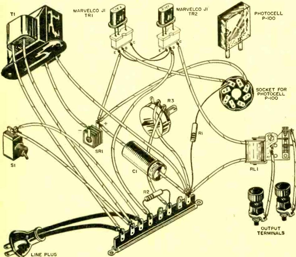
Parts of the photo-relay are interconnected as shown in this pictorial diagram.
