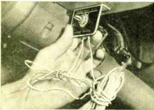
**WIRE SWITCH.** The switch, with 1 triple, 2 double contacts, taps line from transformer to front speaker, with extension line and ground for rear. Solder long "blue" line to triple "both" contact. Hook 2' "white" line to 2-contact "rear" position, "red" to 2-contact "front" post. Mount under dash.
