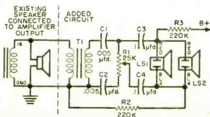
Schematic for the electrostatic tweeter.
