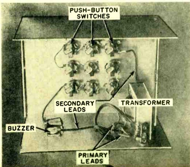
Metal cabinet, doorbell transformer and buzzer, a two-terminal tie-point strip, nine push-button switches, power cord and hookup wire make up the simple parts list for the intelligence tester. Push buttons with s.p.d.t. contacts are employed, and connection is made to normally closed contacts of all switches except the three that will be used to ring the buzzer.
