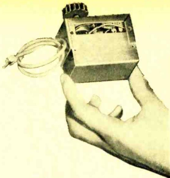
Most "presence controls" in hi-fi components are built right into the circuits of preamplifiers or amplifiers. Yet it is quite simple to add this type of control externally to almost any hi-fi system.
