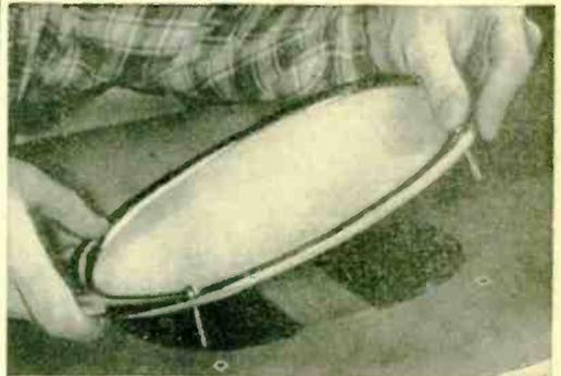
**CUT SHELF.** Using a sharp knife, carefully follow outline (above). Then lay moulding and baffle in place and drop mounting bolts through holes (above, right). Mount speaker from the trunk, using a weight to hold bolts in place (as shown below).
