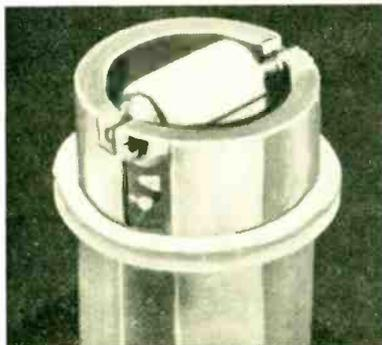
The photos above and at right show both ends of the Atomotron's charging belt. See exploded view of model for construction details. Ionic or corona discharge from the sharpened points of the support rod makes the model spaceship revolve rapidly around hollow aluminum sphere.
