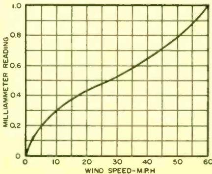
Typical calibration graph used with meter.
