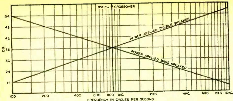
Fig. 1. Assuming 72 db of available sound energy, half of it (36 db) is applied to each speaker at the crossover point. At other frequencies the proportion varies, one speaker getting less while the other gets more, but the sum of 72 db is constant.
