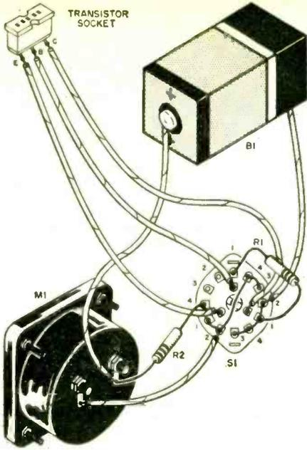
Pictorial and schematic diagrams show how parts are interconnected. See parts list below.
