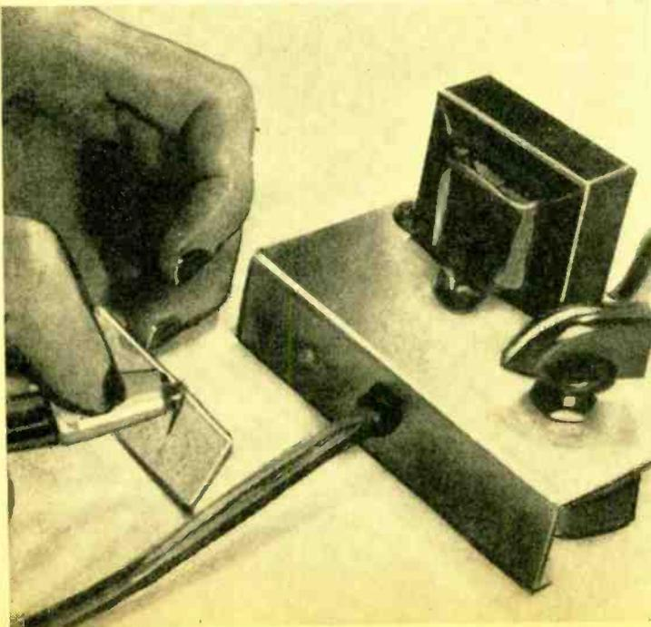
**Note** the construction of the power supply in the aluminum chassis. A rubber grommet is used to protect the power cord. Tool is being used to burn name into piece of plastic. The test leads themselves should not be plastic—the heat might melt them.
