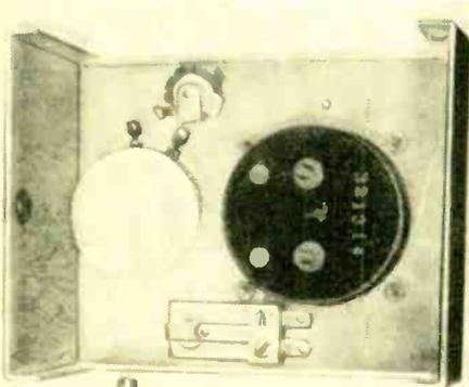
Chassis and subchassis of the control box are at left. The polystyrene subchassis sheet is mounted to rear of meter by the meter terminal screws.
