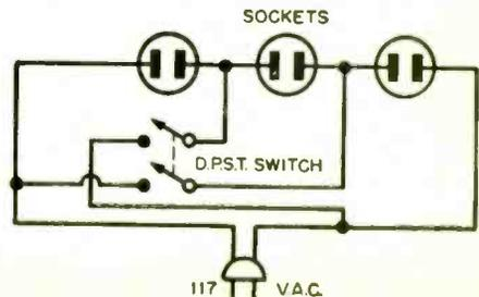
Schematic of dimmer control for photofloods.
