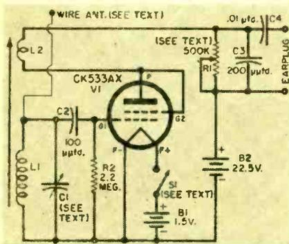
Schematic diagram and receiver parts list.
