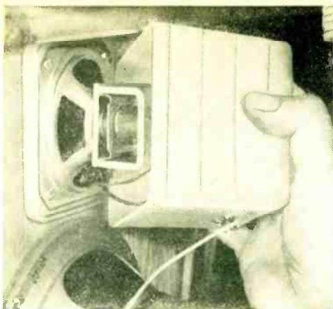
At left is view of plastic freezer container being mounted over the tweeter to isolate the back wave from the woofer. If a horn-type tweeter is used, this precaution is not necessary.
