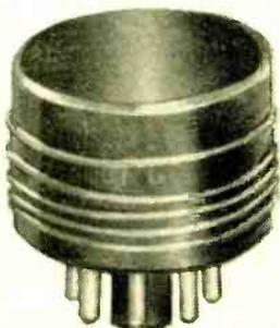
Four plug-in coils, such as the one shown here, cover the basic frequency range. Data for each coil is given in the box above. You can salvage the coil forms from defective octal tubes as described in the text.
