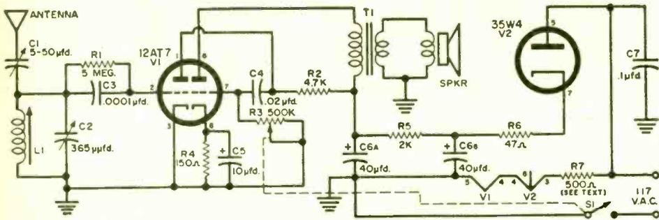
Schematic and pictorial diagrams for junk box receiver. A 12AU7 can be used in place of the 12AT7 if it is more easily obtained.
