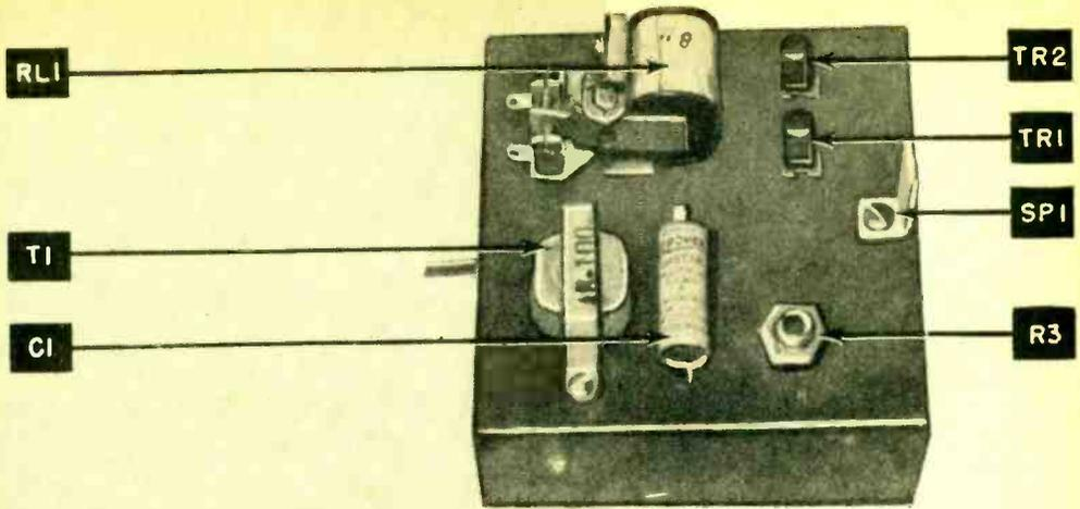
is the point of maximum sensitivity. For applications requiring a lower sensitivity, adjust  $R3$  in the direction of decreasing resistance until the desired sensitivity is obtained.
