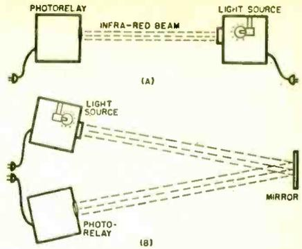
If light source and photo-relay are set up at opposite ends of site, as in (A), you will need two different outlets. They may be set up side by side, however, both a.c. plugs then going to the same duplex outlet, as in (B); a small mirror reflects beam back to relay and the total throw distance is doubled.
