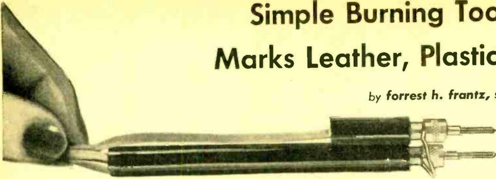
**H**ere's a burning tool you can make in half an hour. You can probably find all the materials in your junk box, or at most, they would cost you \$3 to \$4 at any parts store. The transformer is a 6.3-volt filament transformer capable of delivering 3 or more amps. The 100-ohm, 5-watt rheostat is the temperature control. A short length of Nichrome wire makes up the burning tip, which you can attach to the ends of an ordinary pair of test prods.
