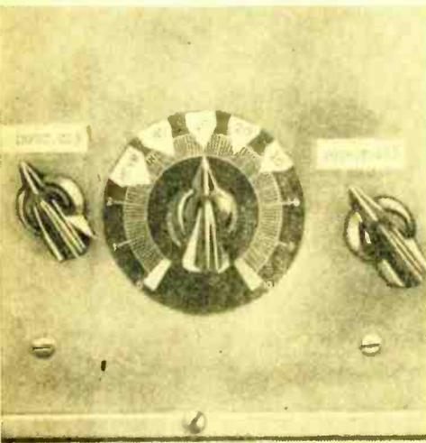
**Front** panel should be marked with proper identification for various bands and for identification of input (C1) and output (C2) capacitors.
