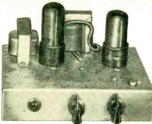
On the front of the amplifier are located the pilot light, the tone control, and the volume control. As shown on the preceding page, amplifier is used in hi-fi system that has been chosen to provide good performance at low cost.
