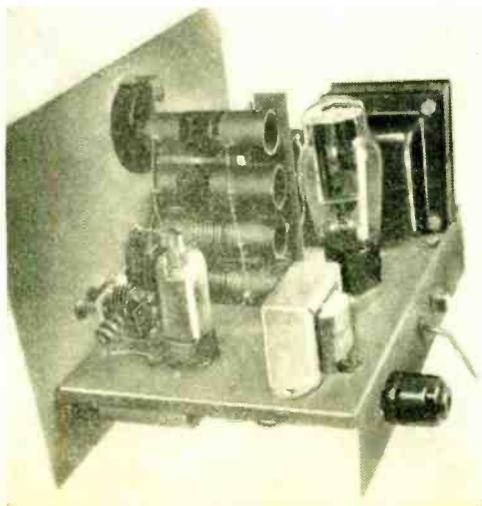
Now make a "parasitic suppressor" by winding six turns of No. 16 or No. 14 wire around a pencil, spacing the turns, so that the coil is about  $\frac{3}{4}$ " long. Slip the winding off the pencil and insert a 100-ohm, 2-watt resistor through it. Solder the ends of the coil to the leads of the resistor close to the resistor body.
