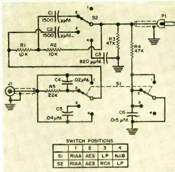
RIAA is only about 5 db, it was possible to construct this unit without any tubes. The total volume loss introduced by the equalizer is just slightly less than 6 db, which simply means that your volume control on the amplifier will have to be set *slightly* higher.
