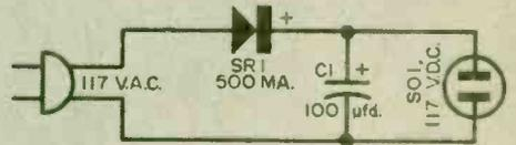
This power supply can be used to increase a motor's speed and prevent excessive heating. Very simple to construct, it is designed primarily for small high-speed motors used on a.c. or d.c., such as the carving motor shown at the top of this page.
