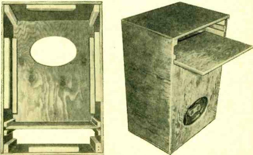
**Rear view of enclosure before speaker is installed (above, left) shows position of bracing blocks. Note how ducted port is installed. The back should be put on with screws for tightest fit. Photo above, right, shows how to tune ducted port—it's best to turn the enclosure upside down.**
