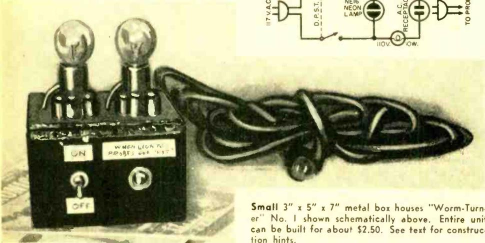
Small 3" x 5" x 7" metal box houses "Worm-Turner" No. 1 shown schematically above. Entire unit can be built for about \$2.50. See text for construction hints.
