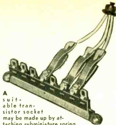
A suit-able transistor socket may be made up by attaching subminiature spring clips to a tie-point strip. Use a 7- or 8-terminal strip; you'll find the extra terminals handy for other components.
