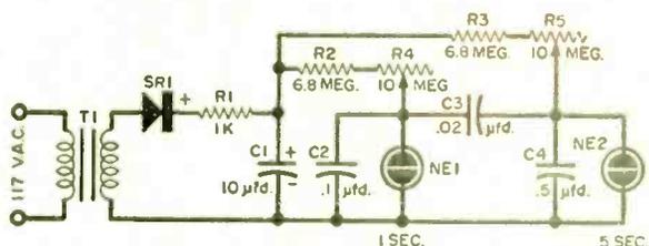
the 1-second and 5-second bulbs. For example, an 11-second interval calls for two blinks of the 5-second bulb, one of the 1-second bulb, and a 23-second interval calls for four blinks of the 5-second bulb, three of the 1-second bulb.
