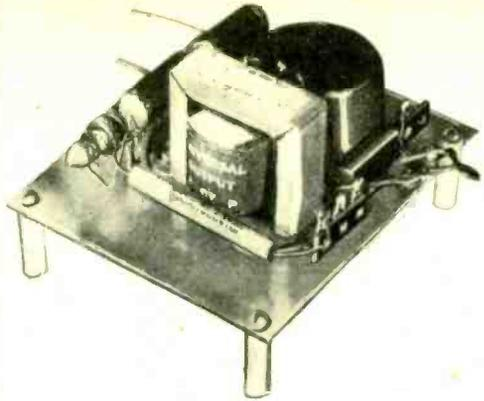
Small enough to be mounted in the same case with a Geiger counter, the power supply weighs one pound.
