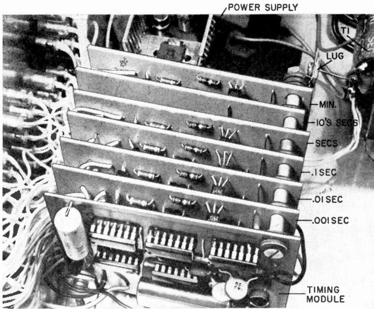
Fig. 9. Timing module and DCU circuit boards should be stacked for space conservation and neatness. Use  $\frac{1}{2}$ "-long insulated spacers (or metal spacers and fiber washers) between each board for adequate separation. Board designations from bottom to top are M2 through M8.
