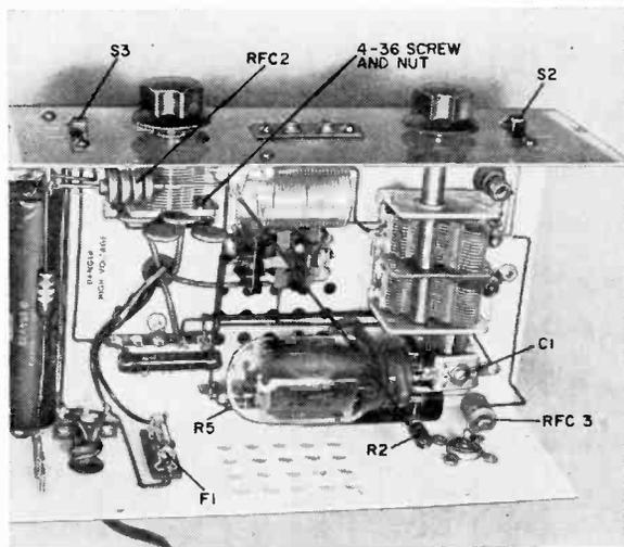
photos and called out in Fig. 2. Otherwise, the considerable amount of heat generated by *V1* will be trapped within the chassis. Four rubber feet, at least ¼" thick, should be fastened to the bottom of the box so that it will clear the operating table sufficiently for air to circulate easily through 25 holes drilled in the bottom directly beneath the tube.
