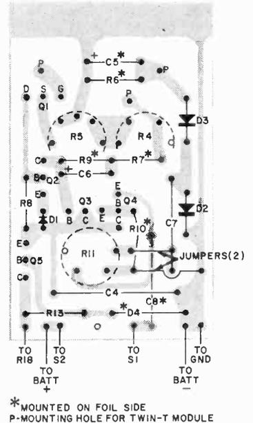
Fig. 4. Note that some of the components are mounted on the foil side of the board to ease construction.
