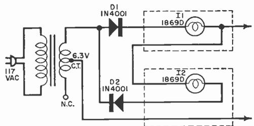
The lamps are connected so that, with equal potential on both probes, both lamps glow very dimly.
