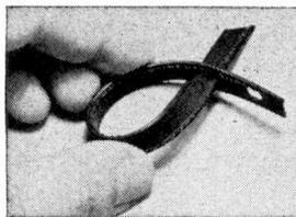
Wrap the fabricated cable tie/hanger around the cables to be bundled together and pass the angled end of the tie through the slot. Pull tight and anchor the tie with a nail or screw where desired. For low voltage, use the twin-lead as is; for high voltage, tear or cut out the conductors.
