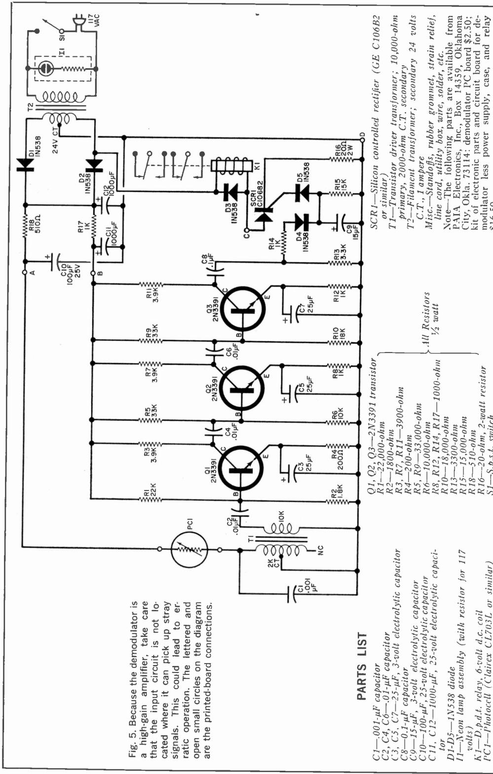
Fig. 5. Because the demodulator is a high-gain amplifier, take care that the input circuit is not located where it can pick up stray signals. This could lead to erratic operation. The lettered and open small circles on the diagram are the printed-board connections.
