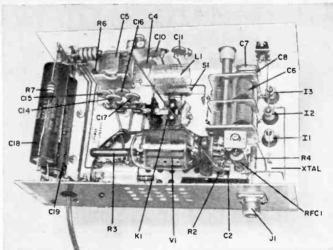
Fig. 3 (left and below). Views of the interior of the transmitter. Mounting details of certain components are shown enlarged on pages 82 and 83. Once the other half of the box is secured in place, the entire transmitter is shielded, and all high voltages are safe from accidental contact.
