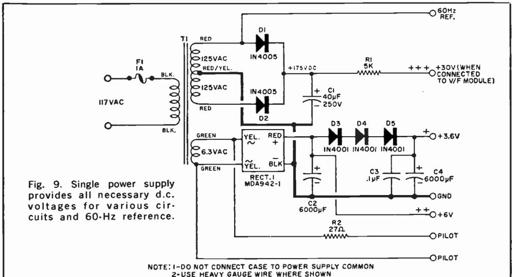
Fig. 9. Single power supply provides all necessary d.c. voltages for various circuits and 60-Hz reference.
