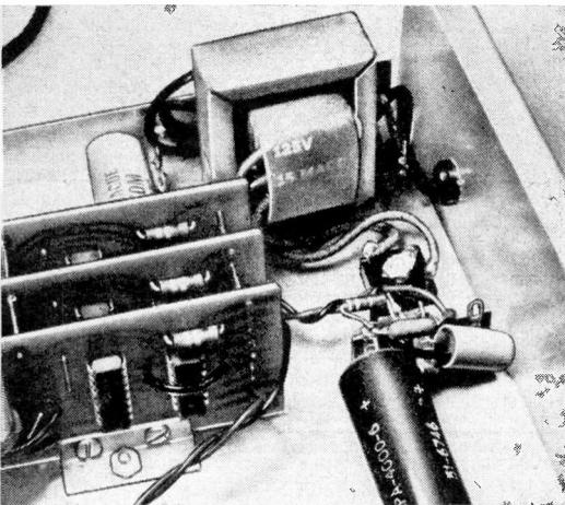
Fig. 5. Terminal strips and point-to-point wiring should be employed when assembling power supply.
