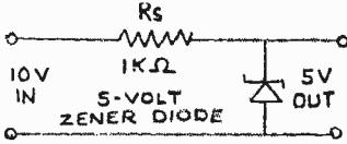
As before with the two 1000-ohm resistors in the circuit, the voltage divides exactly in half so that 5 volts appears at the output. What happens when the input potential is raised to 15 volts? Oddly enough, the output remains at 5 volts as a result of the regulatory ability of the zener diode.
