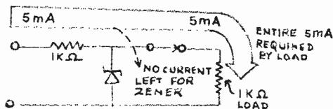
With no current available for the zener diode, it ceases to conduct, and the voltage across the load begins to decrease with further decreases in load resistance.
