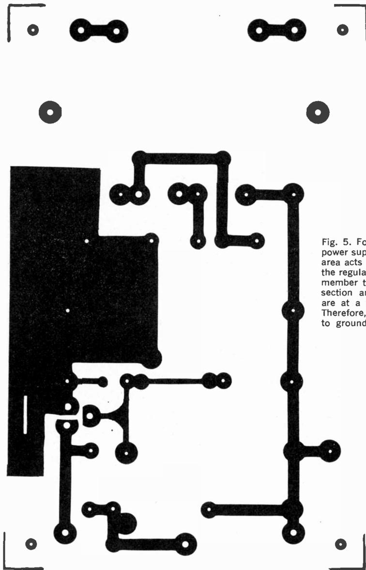
Fig. 5. Foil pattern for the power supply. The large foil area acts as a heat sink for the regulator transistor. Remember that both this foil section and the heat sink are at a full 24-volt level. Therefore, don't short them to ground for any reason.
