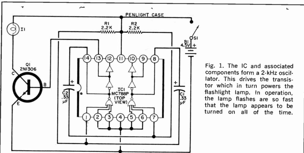
Fig. 1. The IC and associated components form a 2-kHz oscillator. This drives the transistor which in turn powers the flashlight lamp. In operation, the lamp flashes are so fast that the lamp appears to be turned on all of the time.
