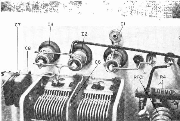
The three bulbs are press-fitted into ordinary rubber grommets. The crystal is mounted adjacent to I1. Note that I2 and I3 are connected in parallel.
