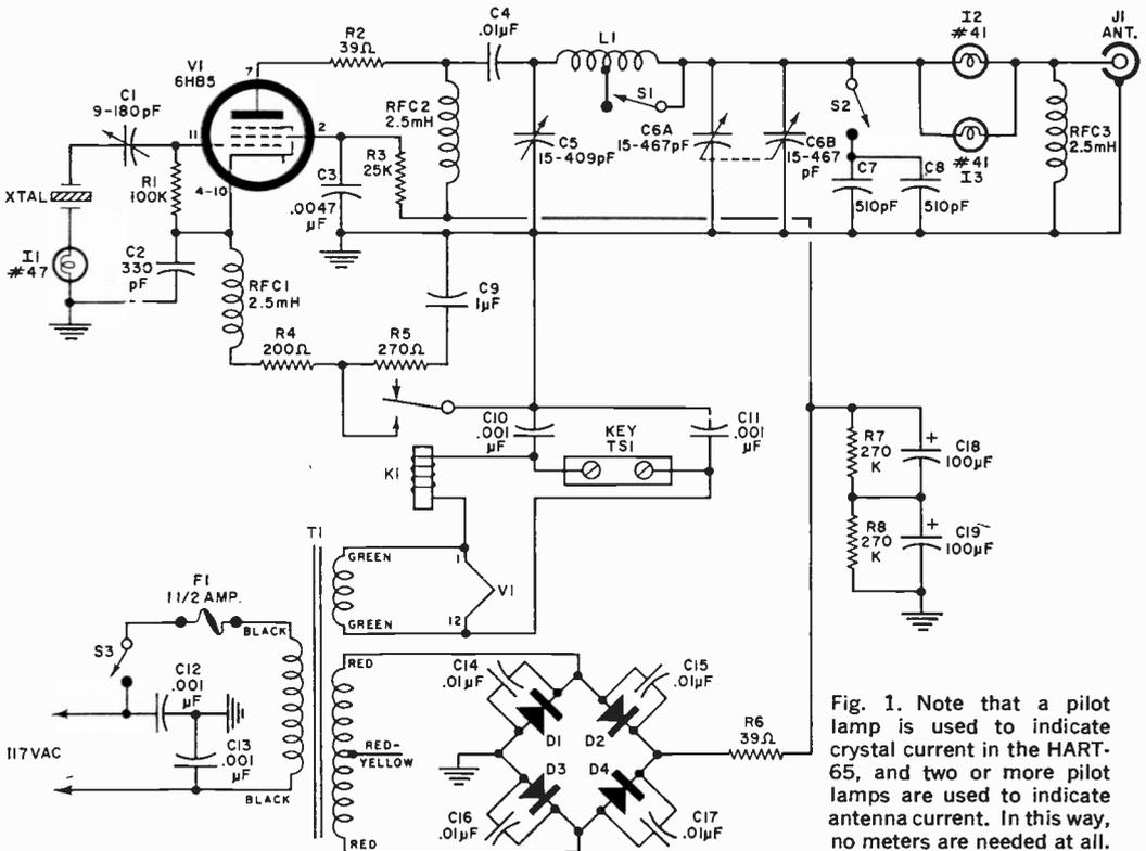
Fig. 1. Note that a pilot lamp is used to indicate crystal current in the HART-65, and two or more pilot lamps are used to indicate antenna current. In this way, no meters are needed at all.
