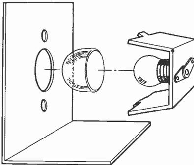
ceiver. Remove the #47 lamps, and replace them with #51 lamps. Then place colored dome-type lenses (for example, red for main tuning and green for bandspread) over the lamps, and replace the lamp holder on its bracket.
