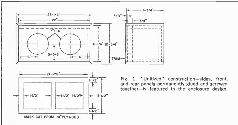
Fig. 1. "Unitized" construction—sides, front, and rear panels permanently glued and screwed together—is featured in the enclosure design.
