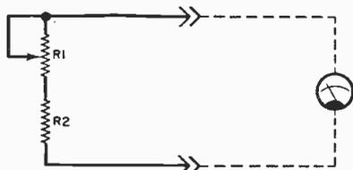
Values of potentiometer  $R1$  and resistor  $R2$  depend on the internal resistance of the meter movement.
