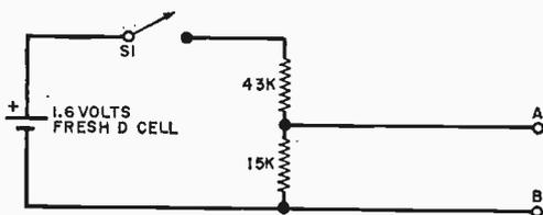
Fig. 6. The outboard calibration circuit for pH meter must be assembled around new, fresh D cell.
