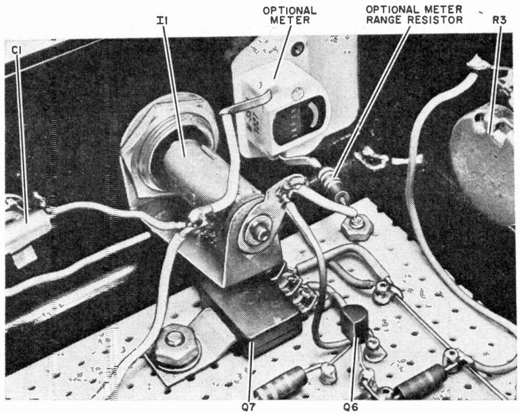
goes off. Now turn *R3* clockwise until the light comes on again. Then rotate *R3* slowly counterclockwise until the light just goes off. The detector is now set for maximum sensitivity. Potentiometer *R2* is used as the coarse control while *R3* is the fine adjustment. The settings of these controls determine at what level the Hotbox responds. If a particular device normally runs hot, set the controls
