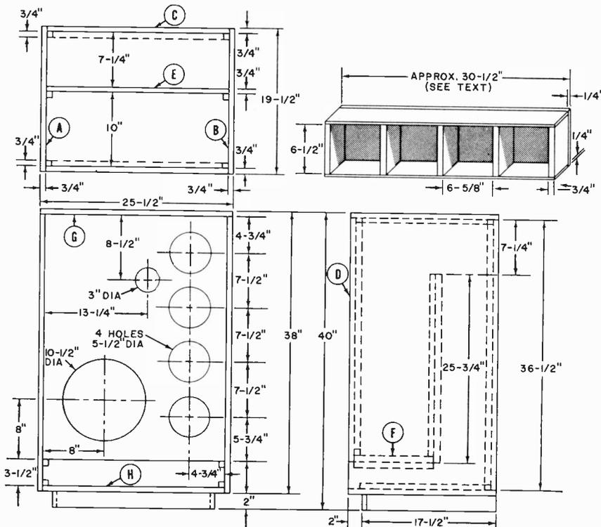
Fig. 1. To avoid confusion, all plates in basic enclosure are identified by letter symbols A through H. Cleats and corner blocks are referred to by lengths as they are used in text.
