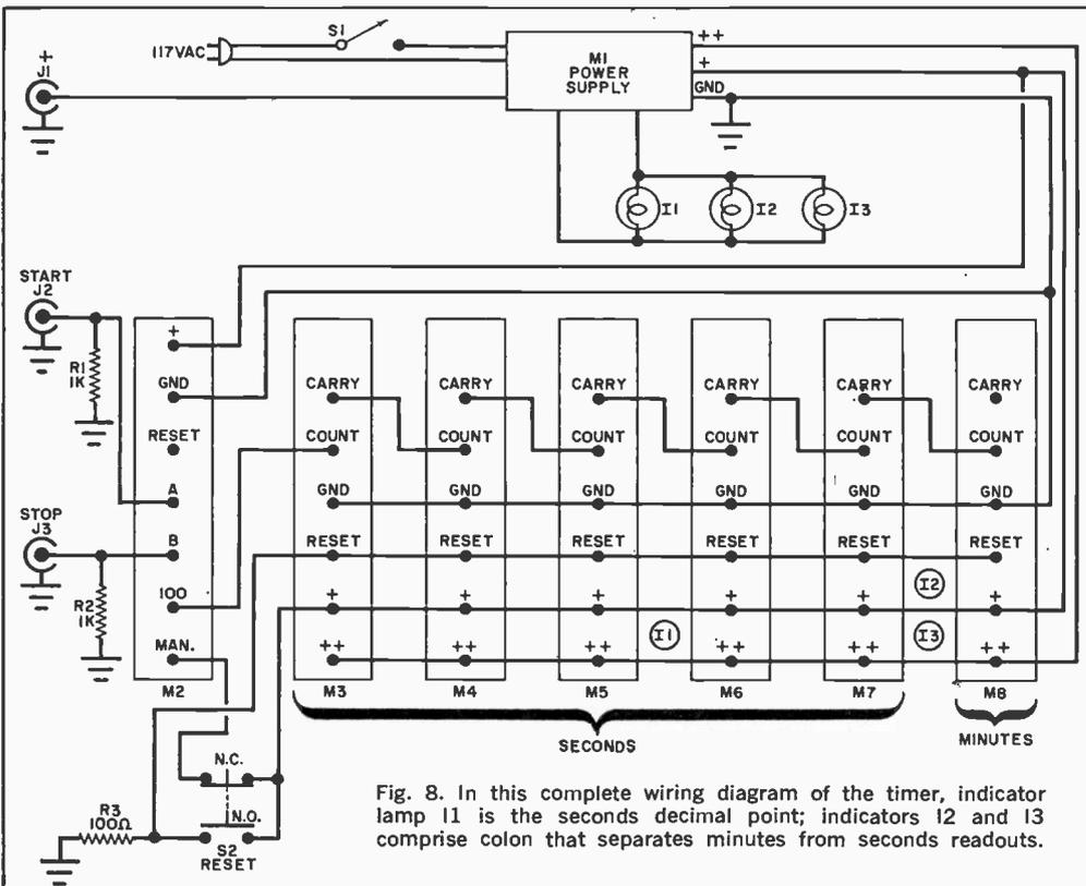
Fig. 8. In this complete wiring diagram of the timer, indicator lamp I1 is the seconds decimal point; indicators I2 and I3 comprise colon that separates minutes from seconds readouts.
