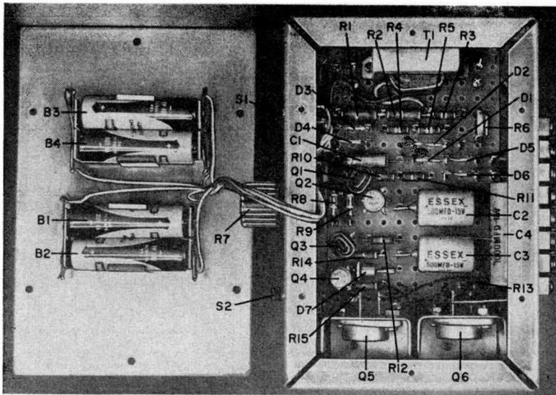
Fig. 2. In layout used by the author, much of the circuit is part of the audio amplifier. If a separate amplifier module is used, the blander assembly is made smaller. Arrangement of components is not critical. The four batteries are for the noise blander only. The amplifier requires a separate battery or a power-supply unit.
