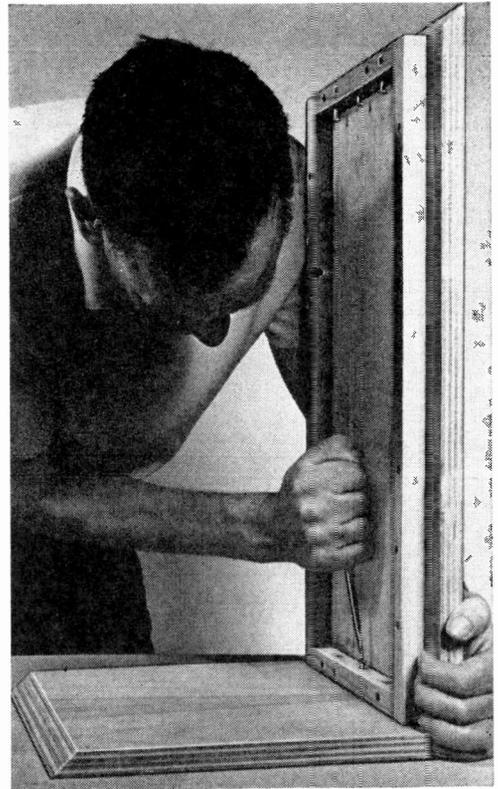
Fig. 2. Corner blocks, drilled in two directions, must be used to anchor sides to top and bottom.
