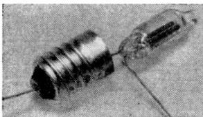
envelope of the incandescent lamp, and remove the elements and whatever glass remains in the screw base. Insert one of the wire leads on the NE-2 through the bottom contact of the lamp as shown in the photo; the other lead goes to the metal case. Insulate the leads from each other, solder both in place and, you'll have a screw-base NE-2 lamp.
