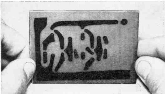
. . . the finished board will be an exact duplicate of the one in the magazine. The foil will be covered with black resist. Use steel wool to remove the dyed resist from the copper. Drill the required mounting holes and assemble components.
