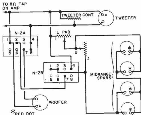
Fig. 2. To obtain proper phasing, be sure to wire all speakers together as shown here. Terminal numbers are stamped right on crossover networks. Tweeter control is supplied by the manufacturer.
