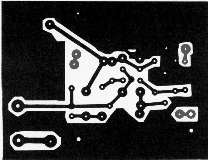
Fig. 2. Use this actual size layout for the PC board for the amplifier. Large amount of foil on the board acts as an extra heat sink for IC1.
