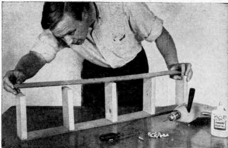
Attach 10" cleats to the bottom side edges of plate F and the 24" cleat to the front top edge. Anchor plates E and F together by letting E overlap F at the rear (see side view drawing in Fig. 1 for details).
