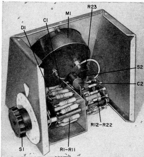
Mount the resistors, shield, C1, and D1 before installing the switch in the chassis. Grounding, through switch mounting hardware, must be tight!
