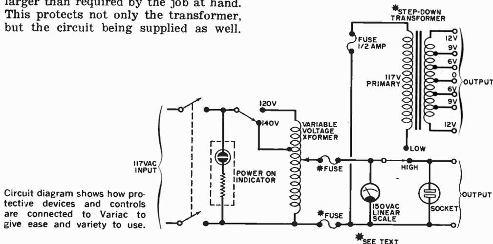
Circuit diagram shows how protective devices and controls are connected to Variac to give ease and variety to use.
