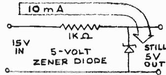
This shows that, while a resistor behaves according to Ohm's law, the zener diode disregards it, changing its effective resistance as needed to provide a constant output voltage.
