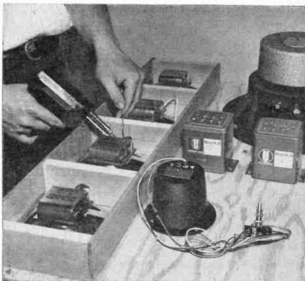
When properly mounted, the crossover networks should be located between woofer and tweeter.
