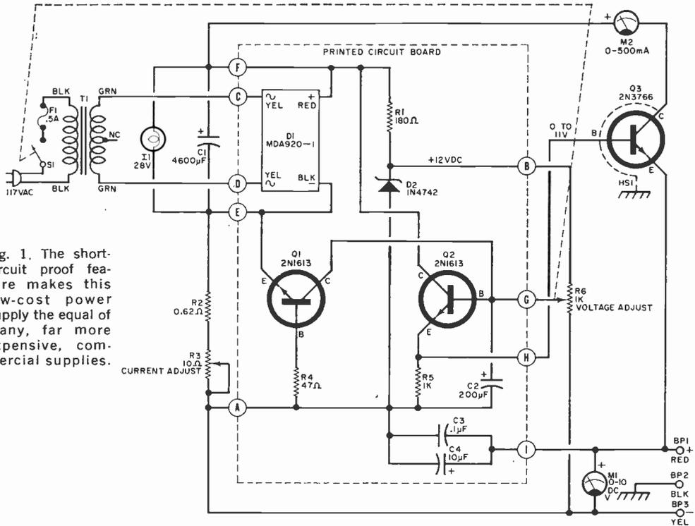
Fig. 1. The short-circuit proof feature makes this low-cost power supply the equal of many, far more expensive, commercial supplies.
