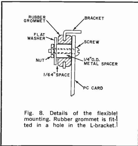
Fig. 8. Details of the flexible mounting. Rubber grommet is fitted in a hole in the L-bracket.
