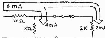
Using Ohm's law,  $E_{out} = 2000 \times 0.0002 = 4$  volts. What happens is that the load resistance shunts the output resistance, decreasing the total resistance "seen" by the source and reducing the voltage drop across the load.
