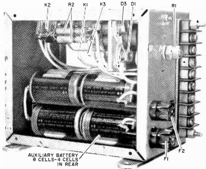
heater will stay on, keeping K2 and the siren off. If the door is closed, the K1 contacts open but K2 is locked in until the 60-second delay of K3 is completed. Then K2 is de-energized and the alarm is reset.
