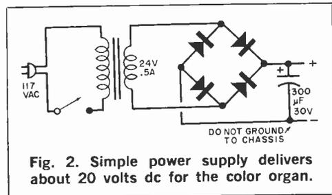
**Fig. 2. Simple power supply delivers about 20 volts dc for the color organ.**
