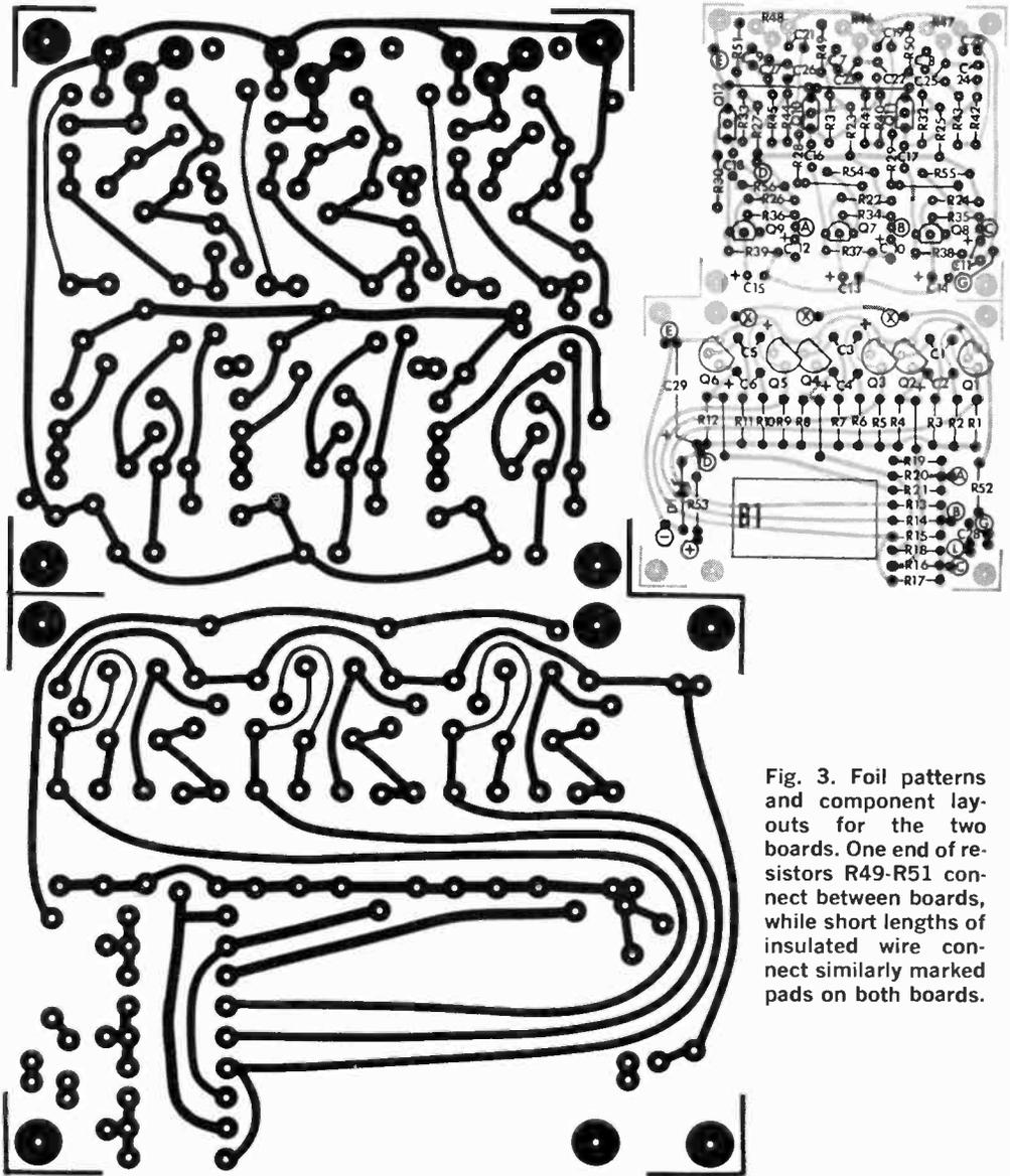
Fig. 3. Foil patterns and component layouts for the two boards. One end of resistors R49-R51 connect between boards, while short lengths of insulated wire connect similarly marked pads on both boards.
