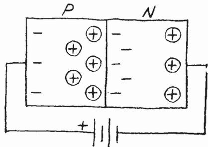
Fig. 2. Pn junction is shown forward-biased.
