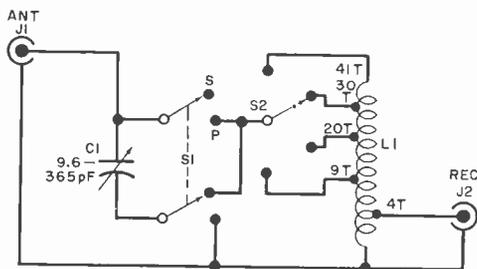
Circuit resonates at desired frequency and provides low-impedance output.
