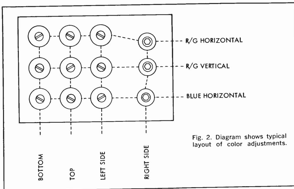
Fig. 2. Diagram shows typical layout of color adjustments.
