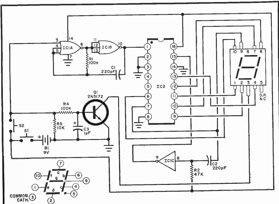
Fig. 2. Actual circuit for a single die. Two gates of IC1 form the 15-kHz oscillator. Its inverter provides a reset signal. IC2 drives the LED readout, turned on by Q1 biasing.
