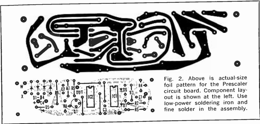
Fig. 2. Above is actual-size foil pattern for the Prescaler circuit board. Component layout is shown at the left. Use low-power soldering iron and fine solder in the assembly.
