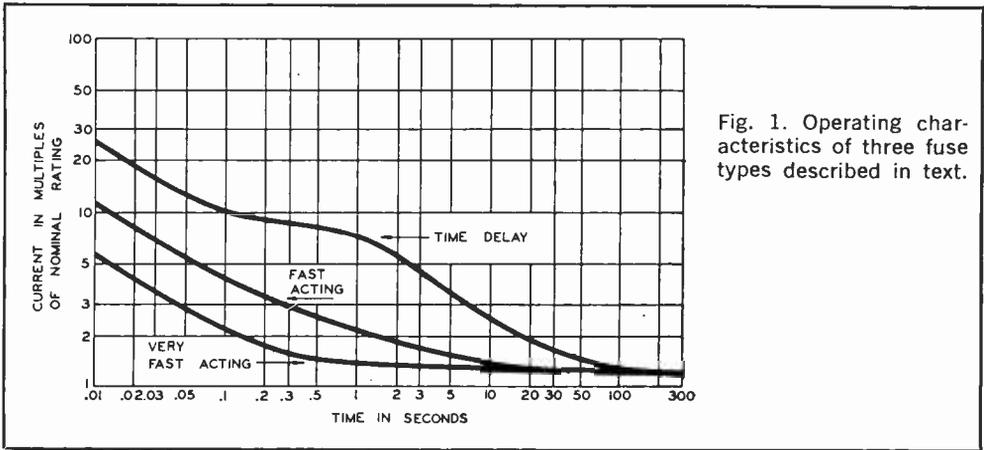
Fig. 1. Operating characteristics of three fuse types described in text.
