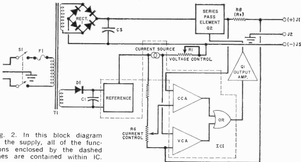
Fig. 2. In this block diagram of the supply, all of the functions enclosed by the dashed lines are contained within IC.
