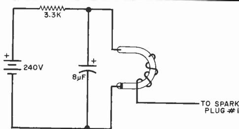
Fig. 8. In this simple engine timing light, the high-voltage pulse at the spark plug triggers the flash tube.
