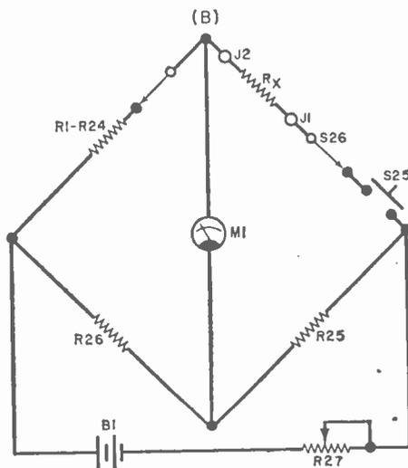
Fig. 2. The classical Wheatstone bridge is illustrated at A, while B shows how it is created in the bridge-substitution box project.
