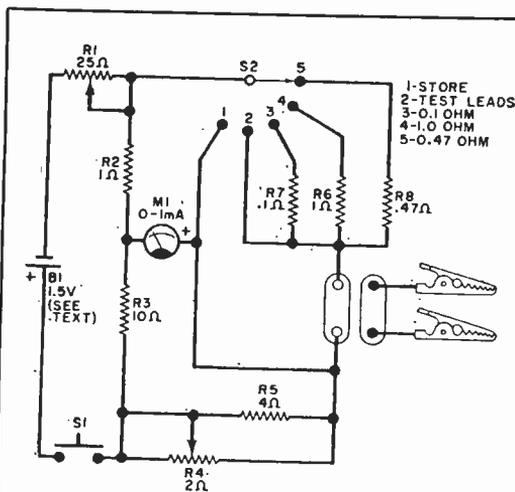
Fig. 1. Resistor R8 provides optional but very useful internal testing facility for checking calibration; S1 is momentary-action switch.
