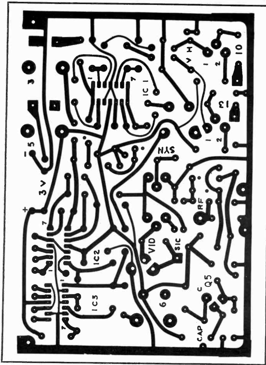
wire (close-wound, with one turn touching the other). Then carefully spread the coil until the ends are  $\frac{3}{8}$ -inch apart. Bend the end leads to the proper angle and remove the resistor before mounting the coil. Before the coil is soldered to the board, solder one lead of *C18* to the coil, four turns from the end connected to the collector of *Q5*. Note that this lead of *C18* does not go through the board, but directly to the coil.
