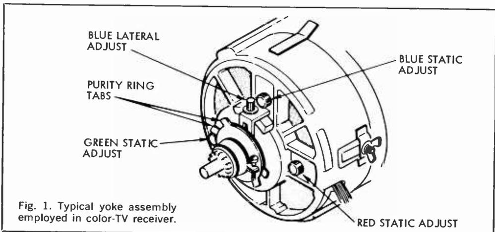
Fig. 1. Typical yoke assembly employed in color-TV receiver.
