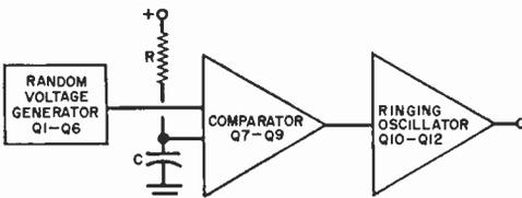
of the random voltage generator output directly to the ringing oscillators in such a way that, when the random voltage is high, the gain and sustain duration of the oscillators is increased. This squelching action allows the sustain on some of the strikes to be considerably longer than would otherwise be possible because of the danger of the circuit breaking into continuous oscillation.
