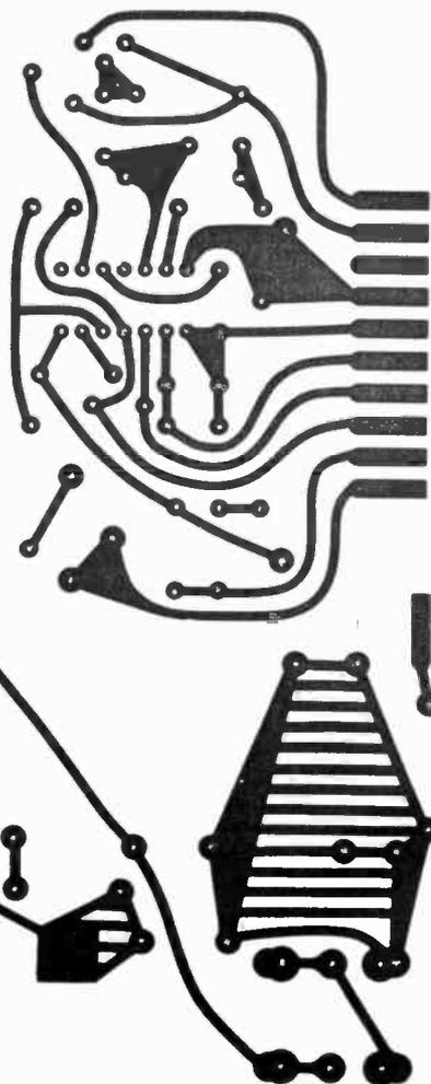
Fig. 3. These are actual-size foil patterns of the printed-circuit boards. They can be made of 2-oz. epoxy-glass.
