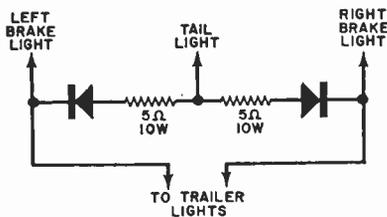
Only "hot" lead hookups are shown: circuit must be completed by connecting a cable between the trailer and car chassis.
