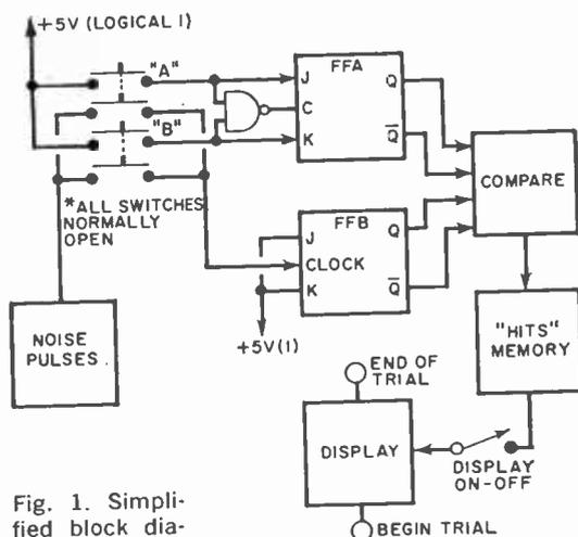
Fig. 1. Simplified block diagram of unit.
