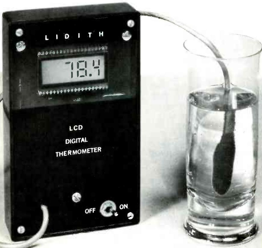
**H**ERE IS AN easy-to-build battery-operated 3½-digit thermometer, which we call "Lidith" for Liquid-crystal Digital THERmometer. It can accurately measure temperatures from  $-13^{\circ}$  F to  $+185^{\circ}$  F. Basic accuracy is better than  $\pm 1^{\circ}$  over this range and averages better than  $\pm 0.5^{\circ}$  from  $0^{\circ}$  to  $100^{\circ}$  F. Each degree is divided into 10 equal parts, giving Lidith a  $0.1^{\circ}$  F resolution. Read-out is on a ½" liquid-crystal display.
