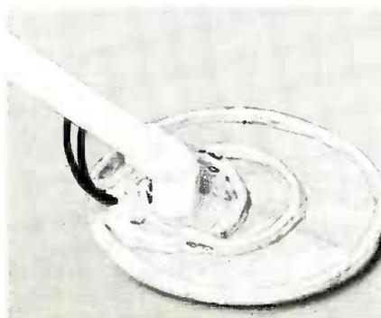
Fig. 5. The search-coil assembly with handle in place.
