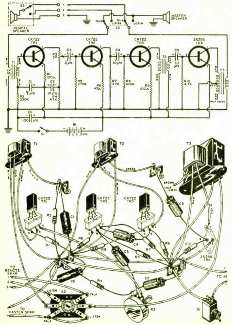
Pictorial and schematic diagrams of the transistorized intercom. ELECTRONIC EXPERIMENTER'S HANDBOOK
