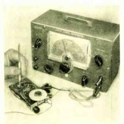
To align the superhet, you'll need a signal generator and an insulated alignment tool. ELECTRONIC EXPERIMENTER'S HANDBOOK
