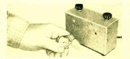
Above illustration shows the darkroom timer being calibrated with a watch. A clock with a sweep second hand may also be used for calibration. At the right, the timer is being used with a contact printer.
