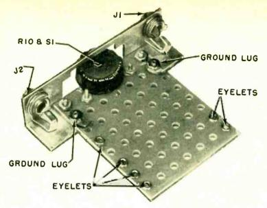
Preliminary assembly of the Bakelite mounting board, "frame" for input (JI) and output (J2) jacks, gain control (RIO) and the power switch (SI). Small evelets are installed in board as terminal connections. Use either or both ground lugs shown for grounding the circuit in accordance with Fig. I. The ground tie point in the pictorial diagram below should be connected to one of these points.
