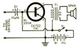
Note the simplicity of the phonograph amplifier circuit. The tap on the secondary of the output transformer should be selected for highest volume. parts list
