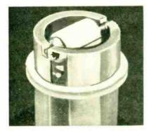
The photos above and at right show both ends of the Atomotron's charging belt. See exploded view of model for construction details. Ionic or corona discharge from the sharpened points of the support rod makes the model spaceship revolve rapidly around hollow aluminum sphere.
