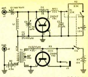
Although the receiver is very sensitive, you'll find it simple to construct if you follow the schematic diagram above.
