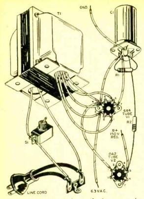
Pictorial and schematic diagrams for the power supply.
