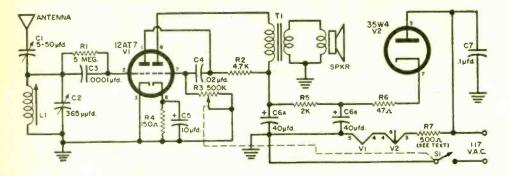
Schematic and pictorial diagrams for junk box receiver. A 12AU7 can be used in place of the 12AT7 if it is more easily obtained.
