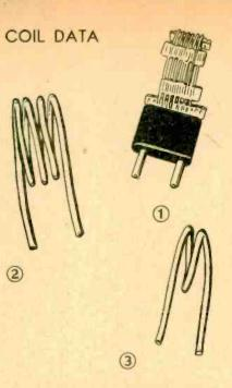
For the 28-50 mc. band: six turns of Barker & Williamson Miniductor No. 3015 coil stock (16 turns/inch), soldered into Millen No. 37412 plug.
