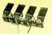
Multi-cell battery, as shown above, will provide greater voltages than a single cell, and can be easily assembled. Fig. I, at right, shows the schematic diagram for this hookup arrangement.
