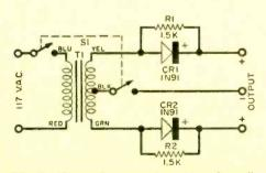
Fig. 2. Circuit for rejuvenating two dry cells of the same or different size and type simultaneously. It will also accommodate single cells. enator. The bottom of the zinc can is the negative terminal of the dry cell. It should always be connected to the negative (center) terminal of the rejuvenator.
