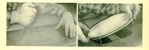
**CUT SHELF.** Using a sharp knife, carefully follow outline (above). Then lay moulding and baffle in place and drop mounting bolts through holes (above, right). Mount speaker from the trunk, using a weight to hold bolts in place (as shown below).
