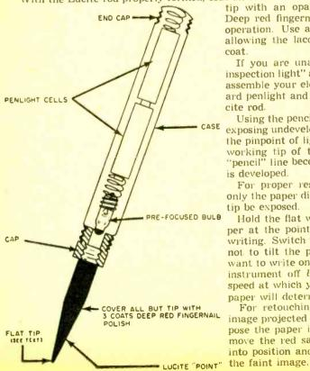
tip with an opaque or deep red lacquer. Deep red fingernail polish is good for this operation. Use at least three heavy coats, allowing the lacquer to dry between each coat.
