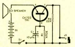
BI-15-volt miniature battery (Burgess No. Y104 C1-10-µfd., 15- or 25-volt electrolytic capacitor J1-Phono jack
