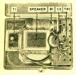
Layout of parts is not critical, but if you want to color the plastic case, don't mount the parts until after the paint has dried. Check all wiring before connecting the hand key or trying the unit.
