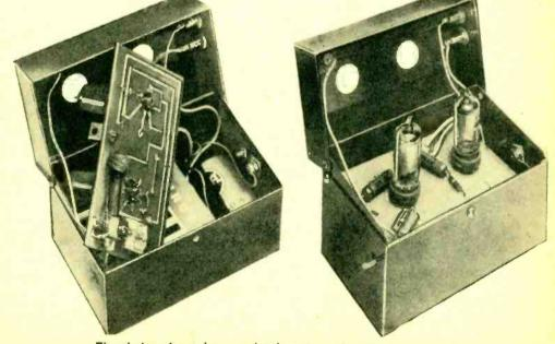
The photos above show completed receiver with cabinet open. At left is view of printed circuit board being put into place. Photo at right shows completed assembly. Note location of phone jacks, batteries, etc.
