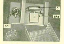
This power supply can be used to increase a motor's speed and prevent excessive heating. Very simple to construct, it is designed primarily for small high-speed motors used on a.c. or d.c., such as the carving motor shown at the top of this page.
