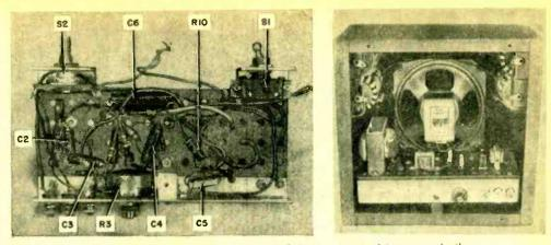
Views of the parts placement layout of the transistorized intercom. In the photo at left, the amplifier chassis is shown from below with major parts identified. Photo at right shows intercom cabinet with all parts installed.
