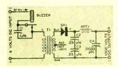
C1-0.1-µfd., 600-volt metalized paper capacitor C2, C3-0.25-µfd., 600-volt metalized paper capacitor C4-0.0033-µfd., 1000-volt mica capacitor RFC1-21/2-mh. r.f. choke (National R-100) SR1-High-voltage, cartridge-type selenium rectifier (International Rectifier U50HP) TI-Universal output transformer (Stancor A-3823) BUZZER-High-frequency buzzer (Johnson Type 114-400)
