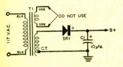
TI-TRANSFORMER, STANCOR #PS-8416 CI-ELEC. CAPACITOR, TUBULAR, 10,,/fd., 350V. SRI-SELENIUM RECTIFIER, 130 R.M.S. VOLTS, 20 MA. D.C. OUTPUT
