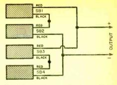
Fig. 1. Four-cell battery with series-parallel connection. The upper pair and lower pair are each connected in series and then in parallel. Color coding shown applies to B2M selenium cells.
