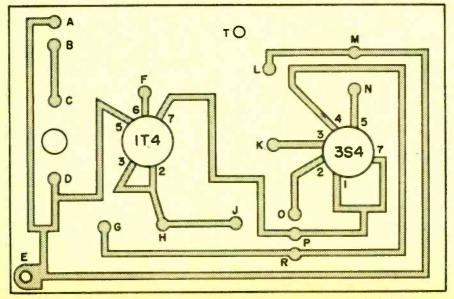
Full-scale layout of the printed circuit board. Tape resist goes on all shaded areas. ELECTRONIC EXPERIMENTER'S HANDBOOK
