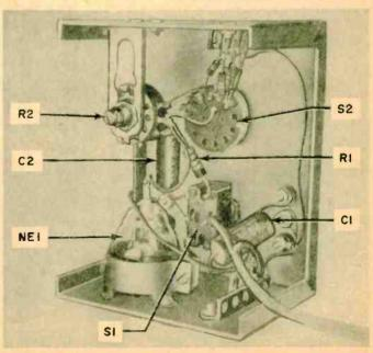
eter until a reading of Rear view of the unit in which the major components are identified.
