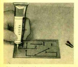
Using a ball-point ink tube to draw the circuit, 178 ponents are mounted in position, leads and connections are soldered, and all hardware —such as mounting brackets and tube sockets—is installed.
