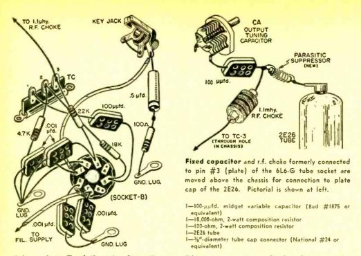
tube socket. Bend the wire from the parasitic suppressor towards the plate cap of the tube and solder a tube cap connector to it. Leave the lead just long enough to permit putting the connector on the tube cap without strain.
