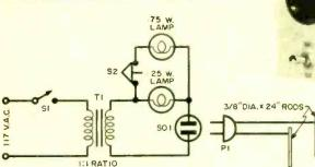
transformer. This current is permitted to be somewhat above the transformer rating since excessive loading will ordinarily be only momentary.
