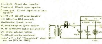
the 1-second and 5-second bulbs. For example, an 11-second interval calls for two blinks of the 5-second bulb, one of the 1-second bulb, and a 23-second interval calls for four blinks of the 5-second bulb, three of the 1-second bulb.
