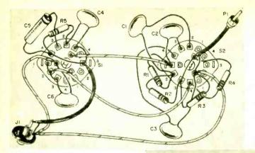
Wiring layout for the equalizer should closely follow the pictorial diagram at left. Switches SI and S2 are viewed from rear. The schematic diagram below shows how SI controls the bass turnover frequency while S2 regulates treble roll-off.
