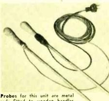
rods fitted to wooden handles and connected to chassis by cord and plug.
