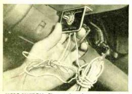
WIRE SWITCH. The switch, with I triple, 2 double contacts, taps line from transformer to front speaker, with extension line and ground for rear. Solder long "blue" line to triple "both" contact. Hook 2' "white" line to 2-contact "rear" position, "red" to 2-contact "front" post. Mount under dash.
