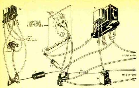
Pictorial and schematic diagrams for the amplifier circuit. Transistor pin connections are identified in the sketch at the left of the schematic. See parts list below.
