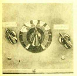
Front panel should be marked with proper identification for various bands and for identification of input (CI) and output (C2) capacitors. Frequencies which lie between these amateur bands can easily be tuned with capacitors C1 and C2. Generally, as the frequency increases, the tuning becomes more critical; and on the 20- and 10-meter positions, care must be taken not to tune the coupler to the image frequency.
