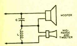
Fig. 2. Elementary crossover circuit for a system using a single woofer and a single tweeter. The inductive component, or coil, may be made at home (see text) from inexpensive materials that you will find at your local hardware store.
