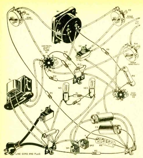
You'll find the pictorial and schematic diagrams helpful in putting the meter together. While VI is shown here as a 12AT7 tube, your particular needs might call for a 12AU7 or a 12AV7, either of which can be used without circuit modification (see text). Parts list is at right.
