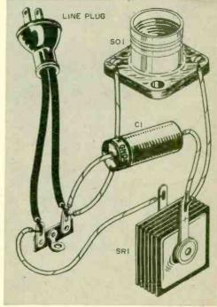
rectifier. It can only be employed with motors using d.c. or a.c./d.c.; motors using just a.c. will not work on the d.c. output of the rectifier.
