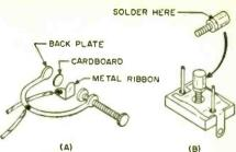
Two special components assure complete miniaturization: on-off switch (A) made from an earring, and (B) extension to capacitor C1.
