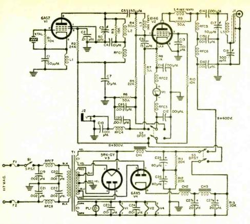
the 6146 beam tetrode (V2) using components  $R_4$ ,  $L_3$  and  $R_9$ ,  $L_4$ .
