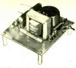
Smoll enough to be mounted in the same case with a Geiger counter, the power supply weighs one pound.
