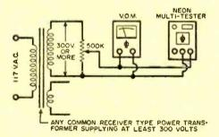
Voltage calibrating setup for the multitester.
