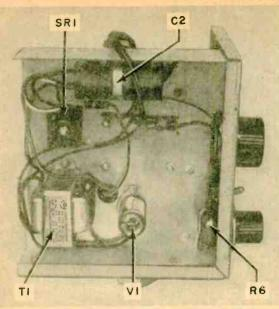
Interior view of left side of the receiver showing location of power supply components and the combination r.f. and audio amplifier tube, mounted herizontally.
