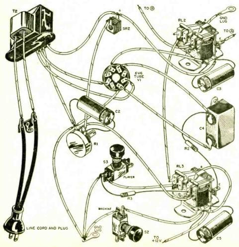
Pictorial wiring diagram for auto-response panel. ELECTRONIC EXPERIMENTER'S HANDBOOK
