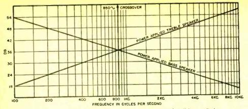
Fig. 1. Assuming 72 db of available sound energy, half of it (36 db) is applied to each speaker at the crossover point. At other frequencies the proportion varies, one speaker getting less while the other gets more, but the sum of 72 db is constant.
