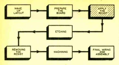
Basic steps in the preparation of an etched circuit. It is in the step labeled "APPLY THE RE-SIST" that simplified techniques can be used and time saved.
