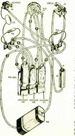
Pictorial diagram shows how printed-circuit is hooked up to other components.
