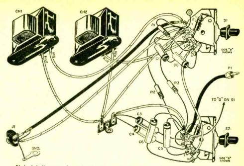
Pictorial diagram above details relationship of parts used in the filter. Note that leads on chokes CHI and CH2 are colored, and must be wired according to instructions. Below are the schematic diagram, table of frequency cutoff action for different switch settings, and parts list. Switches are shown at 100-cps and 4000-cps cutoff positions. All ground points, including shield of output cable, should be returned to connection at ground on JI.
