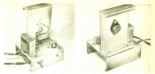
Above are two views showing the mounting details for the heat sink for the 2N255, the power transistor. Four flat fiber washers should insulate the chassis for the heat sink from the amplifier chassis.
