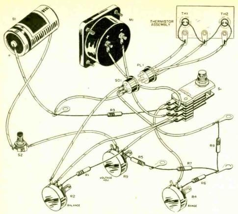
Pictorial wiring diagram of the anemometer.
