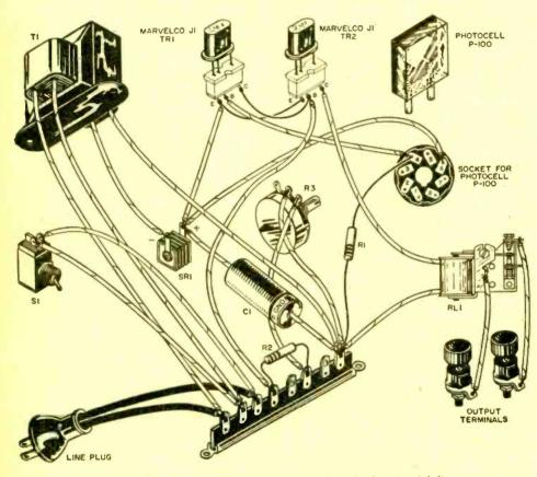
Parts of the photo-relay are interconnected as shown in this pictorial diagram.
