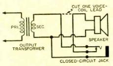
How the pillow speaker jack is wired into the voice-coil circuit of the bedside radio.
