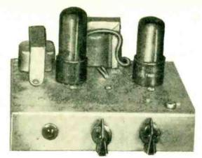
On the front of the amplifier are located the pilot light, the tone control, and the volume control. As shown on the preceding page, amplifier is used in hi-fi system that has been chosen to provide good performance at low cost.
