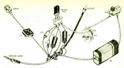
Hook up the "bargain basement" signal tracer's components as shown in the pictorial diagram above; schematic and complete parts list for this simple test unit are given below and at right.
