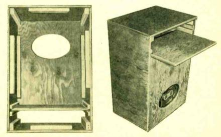
**Rear view of enclosure** before speaker is installed (above, left) shows position of bracing blocks. Note how ducted port is installed. The back should be put on with screws for tightest fit. Photo above, right, shows how to tune ducted port—it's best to turn the enclosure upside down.
