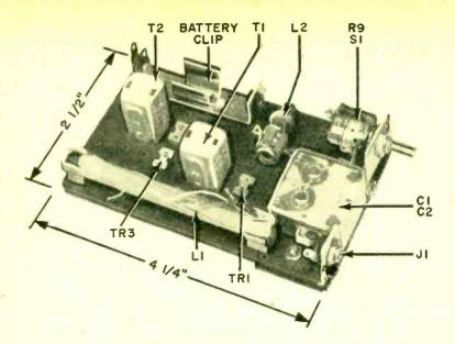
Top view of the receiver chassis shows location of all major components. The transistors are not in their respective sockets. Screw adjustments of CIb and C2b are visible on the top of CI/C2. Antenna coil LI is held in place with a pair of fuse clips.
