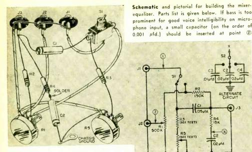
boost. A 0.03-µfd. capacitor will provide essentially flat response, while an 0.01-µfd. unit will increase the bass. If you don't want to bother with the switch, simply experiment with different values until you find one that is pleasing to your ear.
