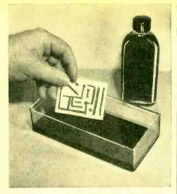
Placing prepared circuit board in the etchant.
