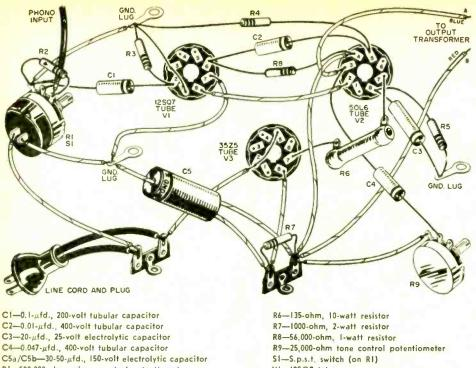
R1—500,000-ohm volume control potentiometer R2, R4-220,000-ohm, 1/2-watt resistor
