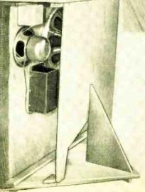
The baffle is shown above without grille to illustrate location of the five speakers. Side view shows construction details; note that the crossover network is mounted where it interferes least with the cross-sectional area of the labyrinth. See the illustration on the opposite page for details on providing acoustical isolation for the tweeter.
