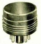
Four plug-in coils, such as the one shown here, cover the basic frequency range. Data for each coil is given in the box above. You can salvage the coil forms from defective octal tubes as described in the text.
