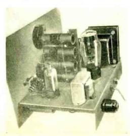
Now make a "parasitic suppressor" by winding six turns of No. 16 or No. 14 wire around a pencil, spacing the turns, so that the coil is about ¾" long. Slip the winding off the pencil and insert a 100-ohm, 2-watt resistor through it. Solder the ends of the coil to the leads of the resistor close to the resistor body.
