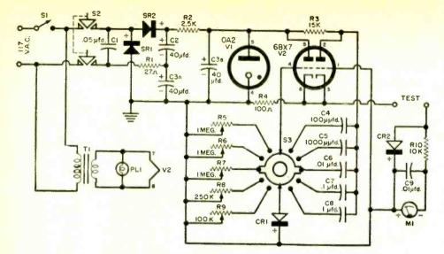
Schematic and parts list for the "Capaci-Meter".
