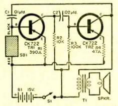
You can use a similar scheme, or provide separate transistor sockets. Make the connections to the battery by soldering leads directly to its terminals. Avoid overheating the battery.
