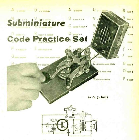
Simple single transistor circuit provides enough output to drive loudspeaker. Entire circuit can be mounted in small plastic box.
