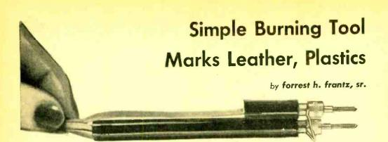
Mere's a burning tool you can make in half an hour. You can probably find all the materials in your junk box, or at most, they would cost you \$3 to \$4 at any parts store. The transformer is a 6.3-volt filament transformer capable of delivering 3 or more amps. The 100-ohm, 5-watt rheostat is the temperature control. A short length of Nichrome wire makes up the burning tip, which you can attach to the ends of an ordinary pair of test prods.
