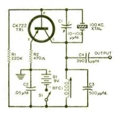
which you can still obtain beats depends primarily on the sensitivity of your receiver. Used on a low-sensitivity a.c.-d.c. "communications type" receiver, the model supplied beats up to 7 mc. On a better receiver, you should obtain beats at 100-kc. intervals up to 20 or 30 mc.
