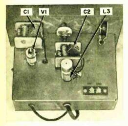
**Top view** of the "5:15" (above), assembled on a 7" x 5" x 2" aluminum chassis. Variable capacitors C1 and C2, coil L3 and the 12BE6 tube are identified. Erequency changing is accomplished by adjusting the oscillator frequency by means of capacitor C2, which is driven by the main dial of the converter. late enough calibration points that way, such a method is just as valid as either of the two following methods requiring more complex equipment.
