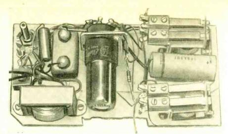
Recommended placement of parts in auto-response panel.
