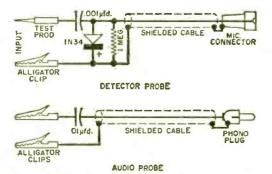
These special probes should have all elements well shielded. The detector probe components can be built into a small tube shield. All capacitors should be 600 volt miniatures. Thin lapel microphone cable can be used for utmost flexibility.
