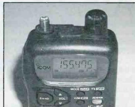
*The R2 provides a clear and easy-to-read display (with the slight exception of the "bank" indicators which are small, and very few controls to clutter the front). It takes a bit of getting used to, but it's easy to maneuver once you've spent some time with this receiver.*
