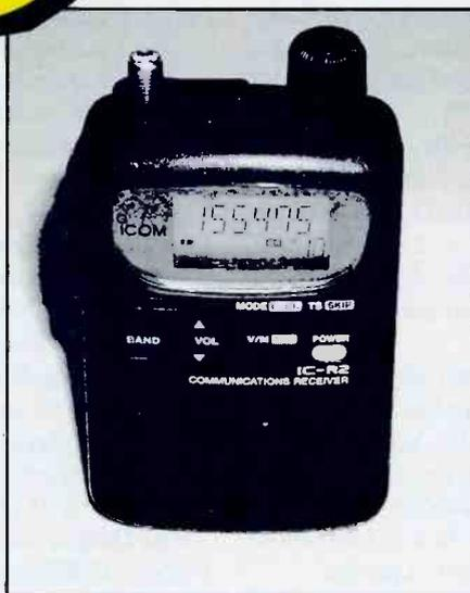
*Barely larger than the average pager, the R2 makes a highly portable package. Note the SMA antenna connector on top. These are quickly becoming standard equipment on many portable ham radios and probably won't be too far behind on many scanners, particularly small ones.*
