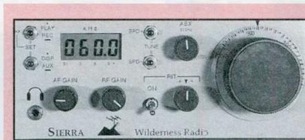
*The only compact, low-current, multiband transceiver kit available, the Wilderness Radio Sierra, uses plug-in band modules for reliability and simplicity. Designed by N6KR and extensively field tested by the NorCal QRP club, the Sierra represents the high end of today's QRP kit radios. Check out the whole line of radios and accessories at [www.fix.net/~jparker/wild.html](http://www.fix.net/~jparker/wild.html).*
