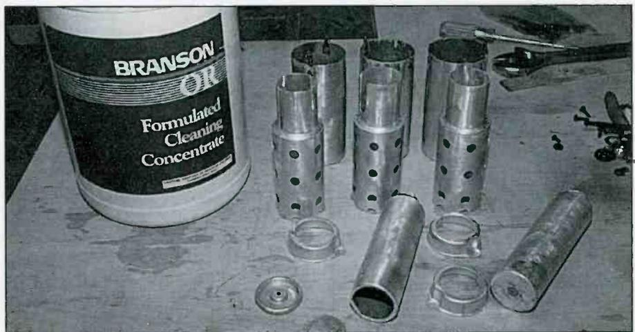
*The aluminum tube shields and IF coil covers sport a renewed luster. Weaker areas of the aluminum are beginning to show signs of erosive etching from the action of the organic cleaning agent, however.*
