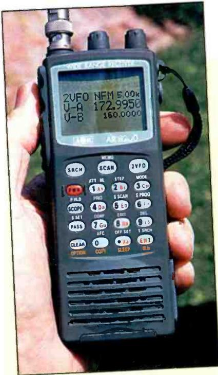
The Arrow antenna coax terminates to a BNC connector for use on your handheld scanner.
