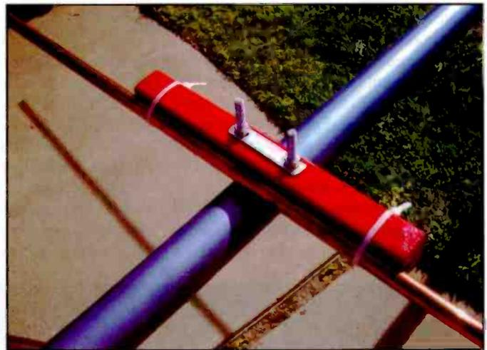
*Photo C. A typical reflector or director element, mounted on the boom during initial testing of the antenna.*
