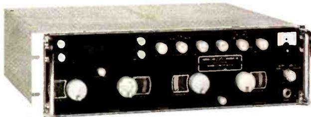
For complete coverage of the frequency range from 30 to 1000 MHz. AM, FM, CW reception. Displays RF signals with built-in signal monitor. Internal relays provide single AM or FM video output. System operated from single antenna input. Four IF bandwidths: 20 kHz, 75 kHz, 300 kHz and 2 MHz. Front panel tuning meter. AGC output available for remote monitoring.
