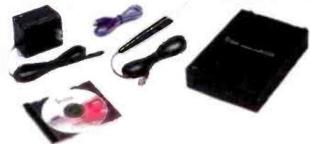
The Icom PCR1500 wideband computer receiver connects externally to your PC via a USB cable. This provides compatibility with many computer models, even laptops. Incredible coverage is yours with reception from 10 kHz to 3300 MHz (less cellular gaps). Modes of reception include AM, FM-Wide, FM-Narrow, SSB and CW. (CW and SSB up to 1300 MHz only). The PCR1500 comes with an AC adapter, whip antenna, USB cable and Windows™ CD. #1501 \$479.95
