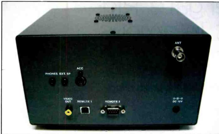
Computer interface jacks are provided both with USB and RS-232 serial. An external speaker, video out, and the standard AOR power and accessory jacks are also available. Note the separate headphone jack, which disables the internal speaker audio.
