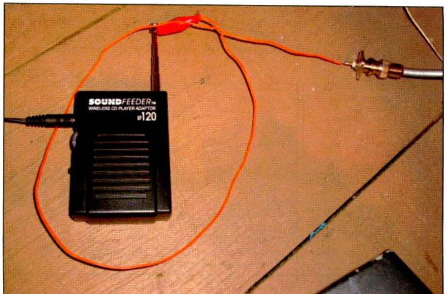
Photo A. The small Arkon SoundFeeder FM transmitter shown hooked up to a longwire antenna. →
