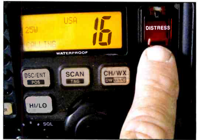
When a mariner transmits an automated DSC (digital selective call) distress call, the data burst changes all DSC receive radios to VHF Channel 16, 156.800 MHz, automatically.
