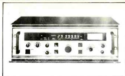
The SR-501 synthesized frequencies are selected by direct access push-buttons in 100 Hz decade switched steps, with up to six channels programmable by diode matrix.
