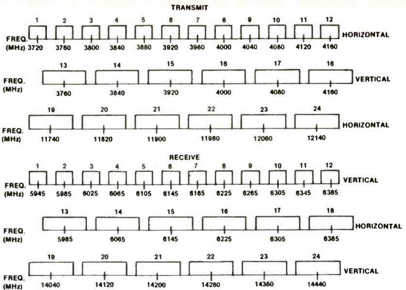
Figure 2. SpaceNet Transponder Center frequencies.
