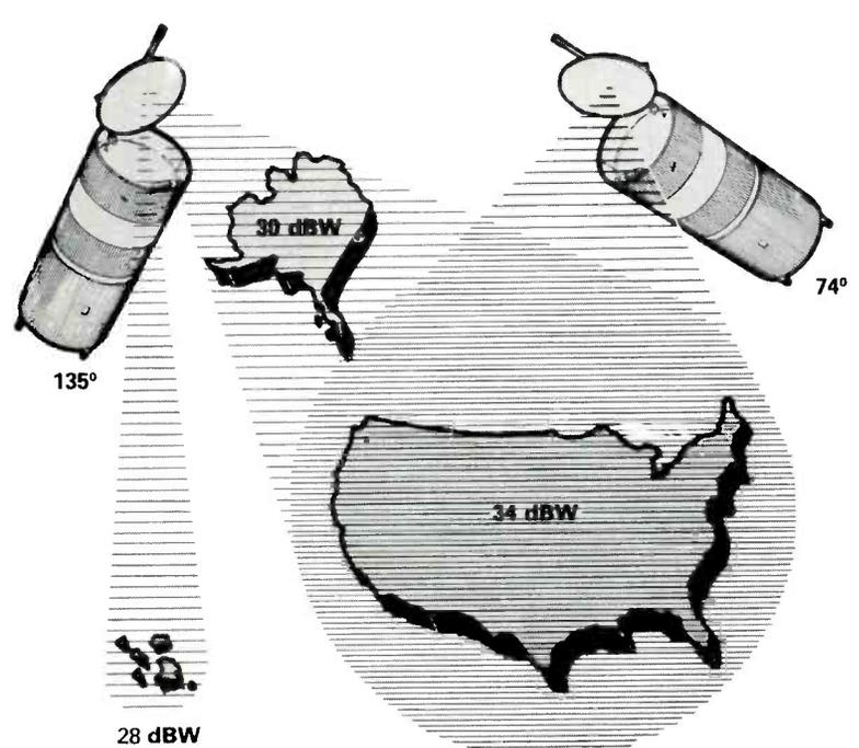
The Satellite located 135°W longitude provides 24 operational channels of at least 34 dBW, 30 dBW, and 28 dBW to the continental United States, Alaska, and Hawaii, respectively. The satellite located at 74° provides 24 channels at a minimum of 34 dBW to the continental United States; Alaska and Hawaii are not visible from this easterly location.
