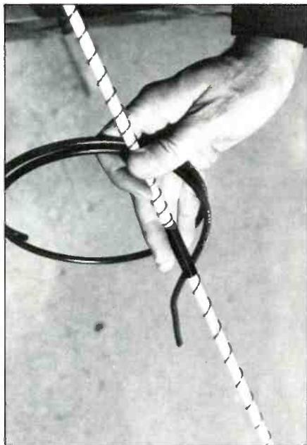
Helical windings on cordless base antenna.
