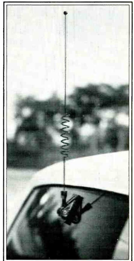
*This coiled 800 MHz "On-Glass" antenna is made by Antenna Specialists and can be used with trunked radio systems.*
