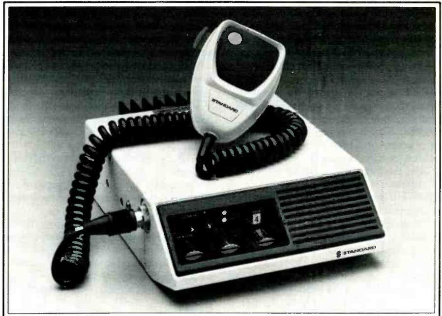
*This 800-MHz trunking radio is made by Standard Communications and is compatible with E.F. Johnson trunked systems. The radio is 35 watts and can operate on up to 40 channels.*
