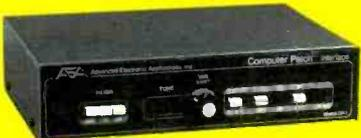
SWL-TEXT is the software and CP-1 is the interface that when combined with your Commodore C64™ and communications receiver, will give you everything you could ask for in a CW/RTTY intercept station!
