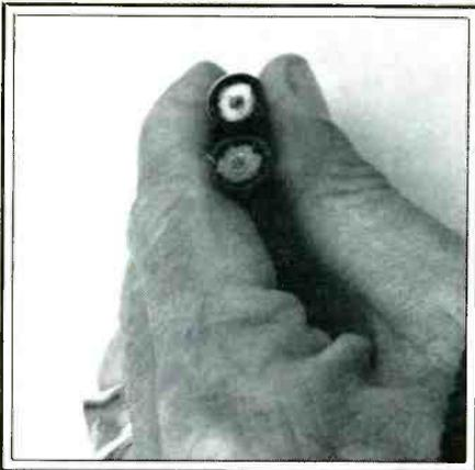
The difference between good and bad—the bottom coax is water damaged and cannot be used.
