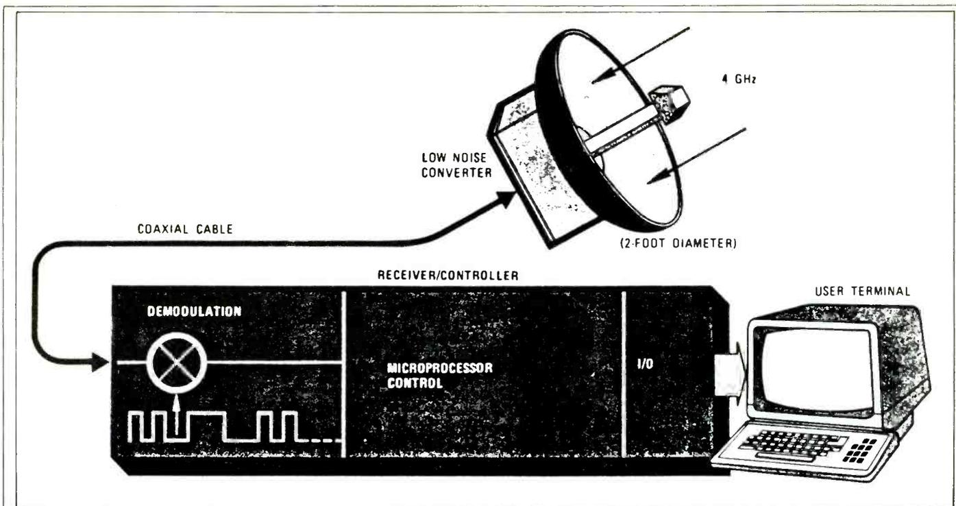
**Downlink:** The satellite signal is transmitted at 4 GHz to the subscriber's 2-foot antenna, amplified, and converted to an intermediate frequency for transmission by coaxial cable to the controller. The signal is then demodulated and sent as a standard digital signal under microprocessor control to user terminals.
