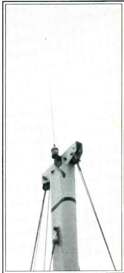
transmission and reception range on 27 MHz CB, plus long distance scanner reception on low band, high band, and at UHF frequencies, too. All that is necessary is a two-position coaxial cable switch that will either select your CB set or your scanner to be fed into the CB/scanner antenna.
