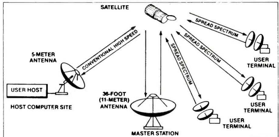
Figure 2: Terminal-to-Host Computer Data Communication Network using spread spectrum satellite link and local terrestrial line.
