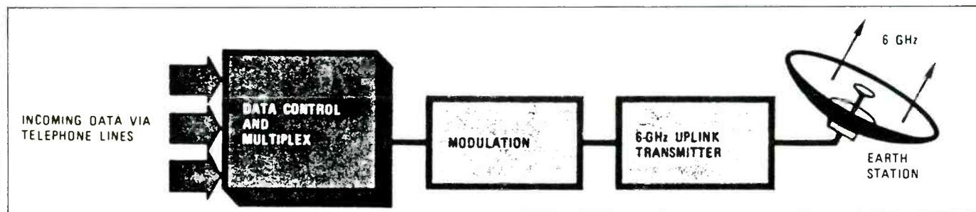
**Uplink:** The transmitting earth station at the broadcast site has the primary antenna — approximately 16 feet in diameter — and fully redundant electronics. The data to be transmitted is multiplexed into packet format, modulated for radio transmission, converted to 6 GHz frequency, and transmitted through the primary antenna.
