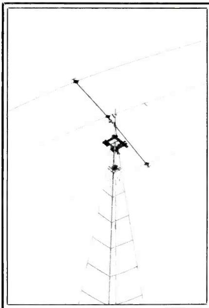
*HF antennas for long range communication can be either vertically or horizontally polarized. The beam shown here is for horizontal polarizations.*
