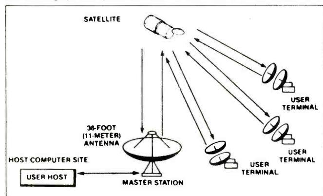
Figure 3: Terminal-to-Terminal Data Communication Network.
