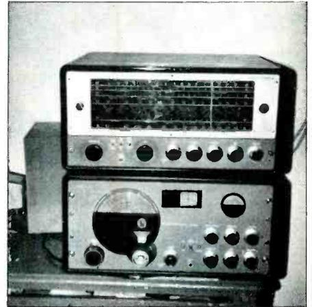
*Two of the finest receivers ever made grace the shack of George Tobin. The Hallicrafter SX42 (bottom) and the SX-62. Both models tune 540 kHz to 108 MHz AM/FM/CW.*
