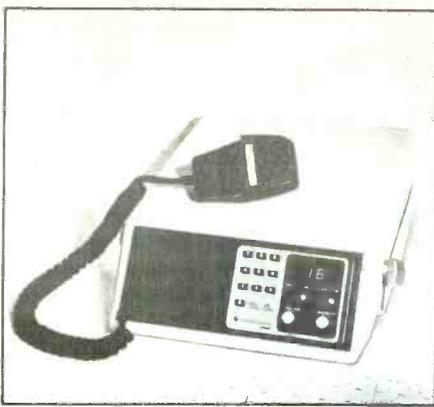
Keyboard channel selection, a fully-synthesized, 55-channel, 25-watt transmitter and a 76-channel receiver with extremely clear sound are features of the new TI-2000 VHF FM marine radio telephone.
