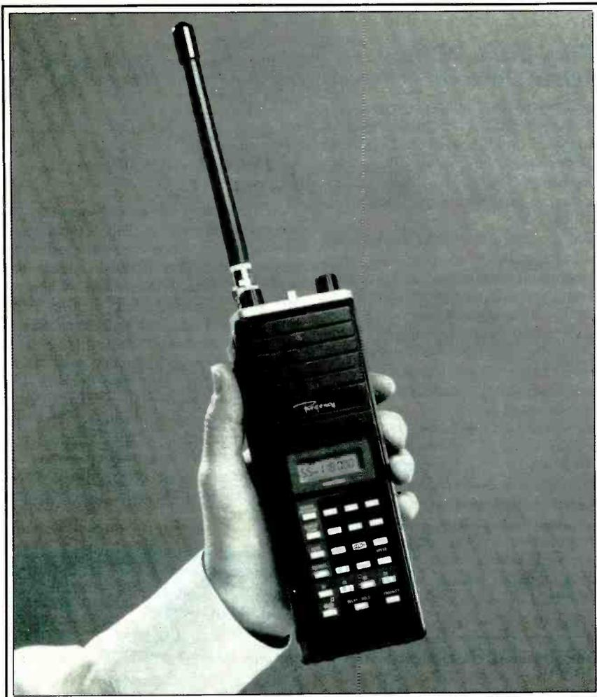
The Regency HX1500 handheld, programmable scanner offers 55 channel capacity, 11 of the most popular bands, plus selectable channel banks.
