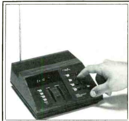
Other important features include channel lockout, for skipping channels not of current interest, plus sliding volume and squelch controls. In the event of a power failure, a built-in capacitor will save frequencies in memory for several hours, without requiring batteries. All electronics are housed in an attractive woodgrain case that features a top-mounted, built-in speaker.
