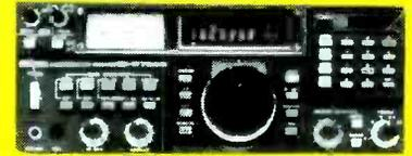
EEB introduces the new ICOM R7000 VHF/UHF receiver, which also is available as the R7000 HP (high performance) with EEB-designed modifications that remarkably improve the sensitivity, audio frequency response, selectivity, and more.
