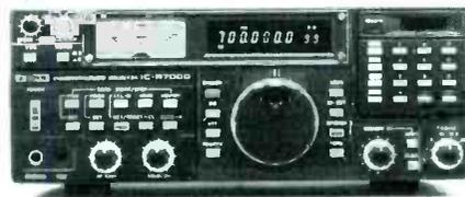
Commercial quality scanning receiver 25-1300 MHz plus, keyboard entry, 99 memories, 5 tuning speeds. Call for \$\$\$
