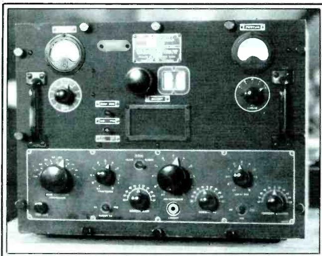
*Like to DX on those low frequencies? This WWII U.S. Navy RAL-7 TRF receiver tunes down to 15 kHz and really pulls 'em in from far away. It weighs a ton and is filled with cast aluminum and ceramics. Thanks to Fred Gwyer, M.D., W9BIU, of La Grange, IL for giving us a look at this great old veteran that still performs like a champ.*
