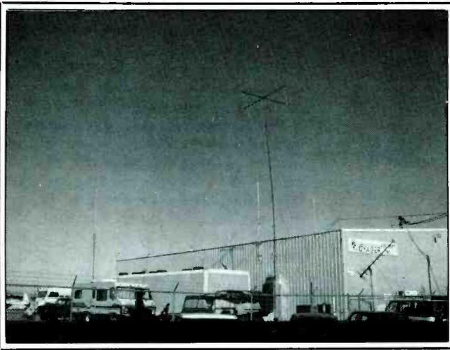
*Voyager Mission Control and antennas. The trailer shown adjacent to Hangar 77 at the Mojave, CA airport housed the Mission Control. The temporary towers at either end of the trailer held up a dipole HF antenna through which communication direct to the Voyager aircraft was often clear.*
