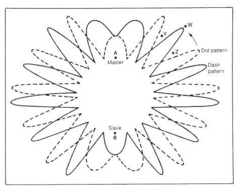
Fig. 1 - Consolan antenna radiation pattern. Observer at A would receive all dashes, at B all dots and at C a combination.
