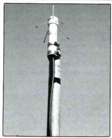
Maximum results are obtained with the MAX-800 mounted outdoors as high as possible, but you need low-loss UHF coax for this
