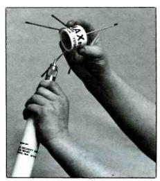
The MAX-800 accepts feedlines using popular PL-259 connectors, although you can order them with Type N connectors on request.
