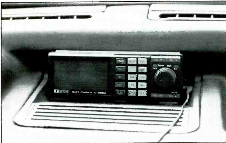
ICOM IC-900A remote controlled multi-band VHF/UHF transceiver.
