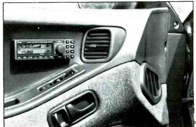
ICOM IC-901A remote head installed in a fire chief's vehicle door panel.
