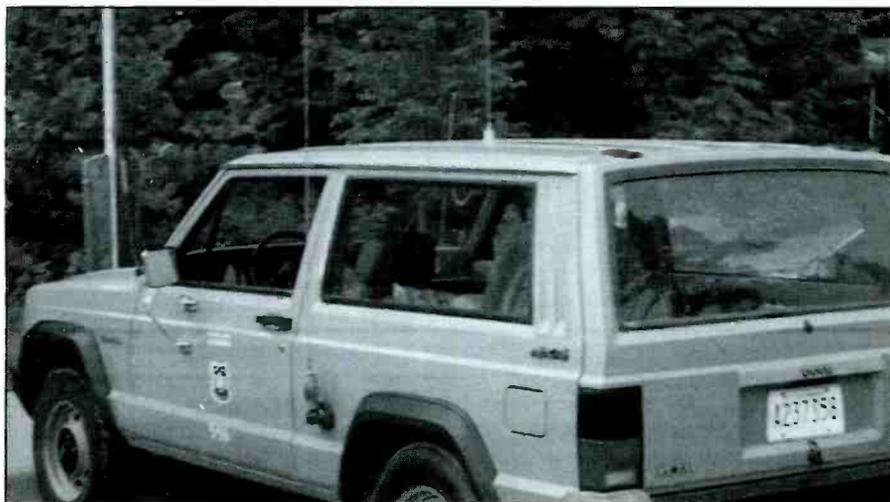
This Dept. of Agriculture vehicle is shown with a VHF high band antenna on the roof. There's also a low band antenna for comms with state and local police.
