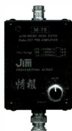
State of the art surface-mount technology coupled with features not found on other pre-amps makes the M75 simply the best. Wide band (24 to 2150 MHz), variable gain -10 dB (attenuation) to +20 dB gain. Bandwidth selector switch covers 3 bands:
