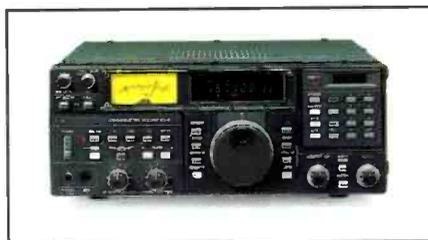
The IC-R71A is a shortwave listener's delight. Its **32 tunable memories** store frequency and mode information, and they are single-button programmable, **independent of VFO A or VFO B's operations!** Dual width, an adjustable noise blanker, selectable RF preamp, and selectable AGC combined with **four scan modes** and all-mode squelch further enhance the IC-R71A!
