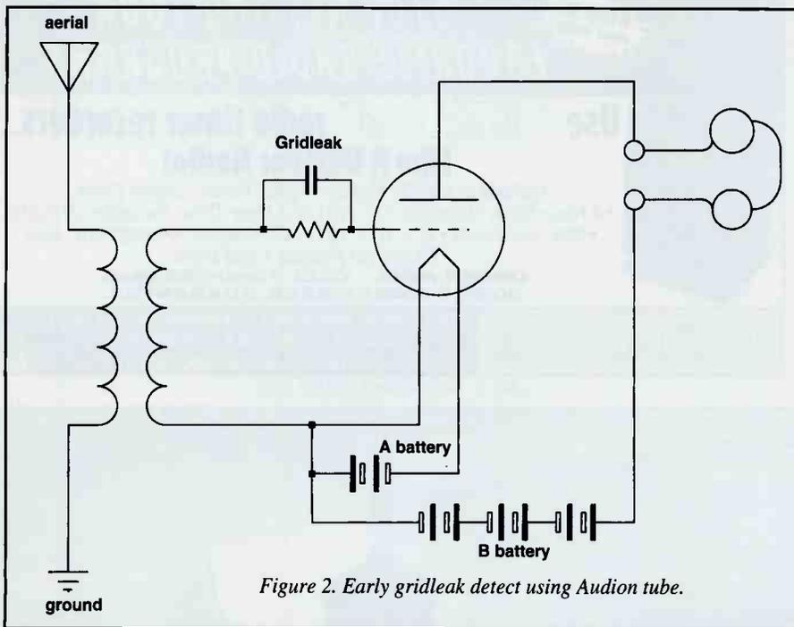
Figure 2. Early gridleak detect using Audion tube.
