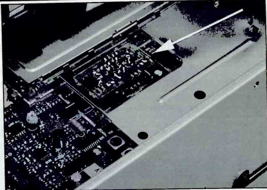
*Some scanners, like the popular BC-9000 from Uniden, need an optional CTCSS board installed before they can take advantage of tone squelch. Note that the 9000 only does CTCSS even with the board — DCS is not available.*
