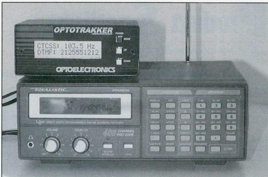
*Shown here decoding a CTCSS tone, the controls on the Optotrakker are simple, yet complete. The large display lights as a tone is received (if desired) making it easy to read even from several feet away.*
