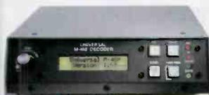
The **Universal M-450v1.5** reader copies: **Baudot, SITOR, FEC-A, ASCII, SWED-ARQ** and **Weather FAX** (to printer port) plus the **ACARS** aviation teletype mode. Features a big two-line, 20 character LCD and bidirectional parallel port. Operates from 12 VDC or supplied AC adapter. U.S.A. #0450 \$399.95 (+\$8)
