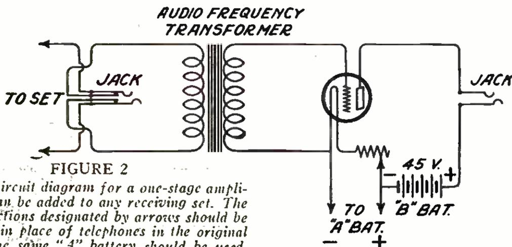
This is a circuit diagram for a one-stage amplifier that can be added to any receiving set. The two connections designated by arrows should be connected in place of telephones in the original set, and the same "A" battery should be used.
