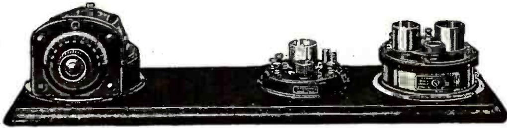
Complete Receiving Set—Coupled Circuit Tuner, Detector, and 2-stage Amplifier
