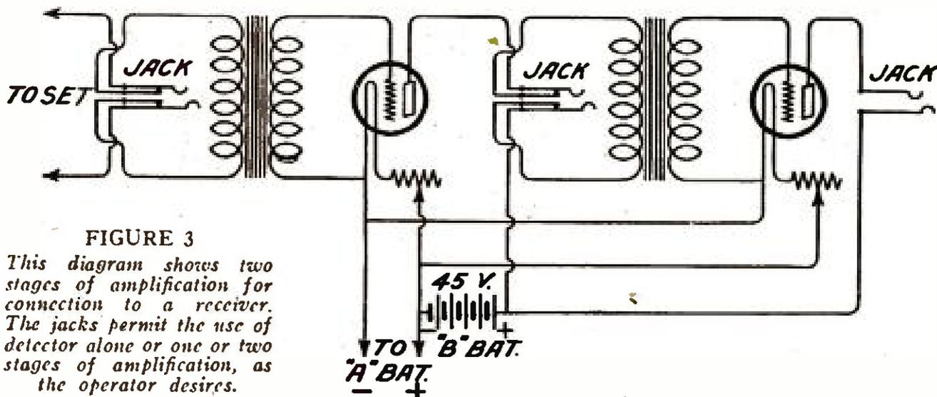
This diagram shows two stages of amplification for connection to a receiver. The jacks permit the use of detector alone or one or two stages of amplification, as the operator desires.
