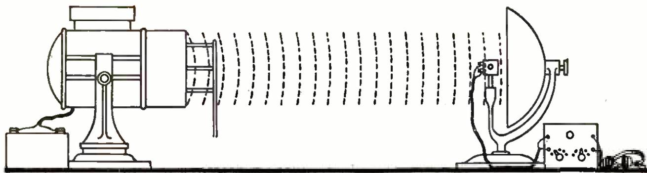
**Q** *A new system of communicating along a beam of light. A light wave is directed in a narrow path from a searchlight and picked up by a reflector which concentrates the waves on a light-sensitive cell which records the signals.*
