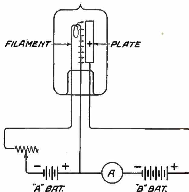
**HOW THE FLEMING VALVE WORKS**
