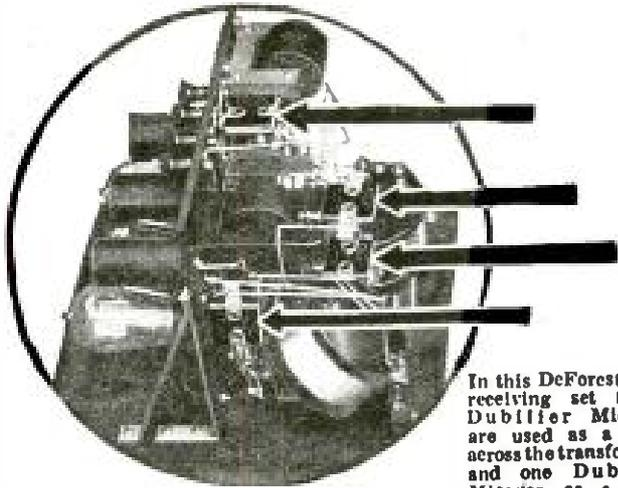
In this DeForest radio receiving set three Dubilier Micadons are used as a shunt across the transformers and one Dubilier Micadon as a grid-condenser. Dubilier Micadons are similarly used in other standard receiving sets.
