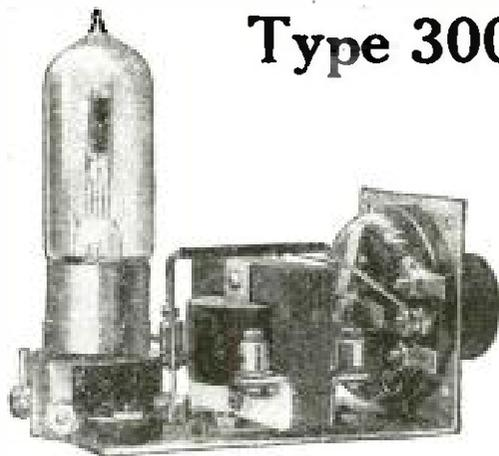
For those who desire a compact amplifier unit, we recommend the type 300. This unit consisting of our Type 231-A Amplifying Transformer, Type 255 Filament Rheostat, and Type 282 Tube Socket mounted on a nickel finished brass plate, is all ready for the external connections. It may be used as a table unit or mounted behind a panel, in which case only the rheostat knob projects. Connections are properly made so as to keep the unit from howling.
