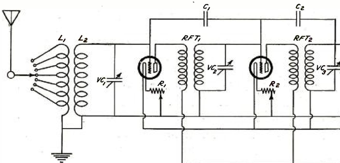
QUESTION: I would like to get a diagram of the hook-up of the "neutrodyne receiver." Will you give it to me, together with list of the instruments necessary? I want to use two stages of neutrodyne radio frequency amplification, vacuum tube detector, and two stages of audio frequency amplification. Also let me have enough information as to the sizes of the coils so that I can construct them.
