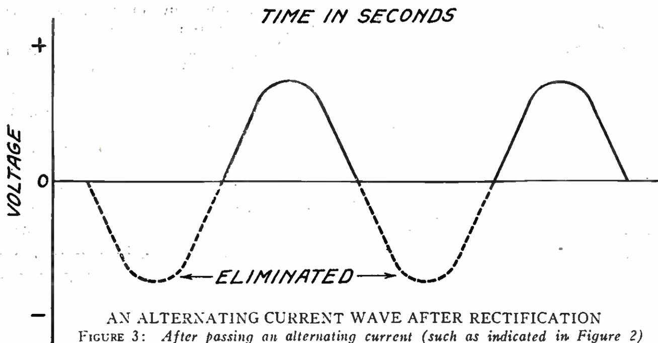
AN ALTERNATING CURRENT WAVE AFTER RECTIFICATION
