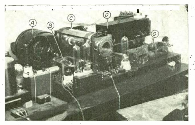
THE RADIO PHOTOGRAPHIC TRANSMITTER A is the synchronous motor and B is a gear that connects it with the cylinder C on which the photograph to be sent is fastened. D is the camera box that is shifted by the magnets G while the varying lights and shades of the photograph are being converted into electric impulses.
