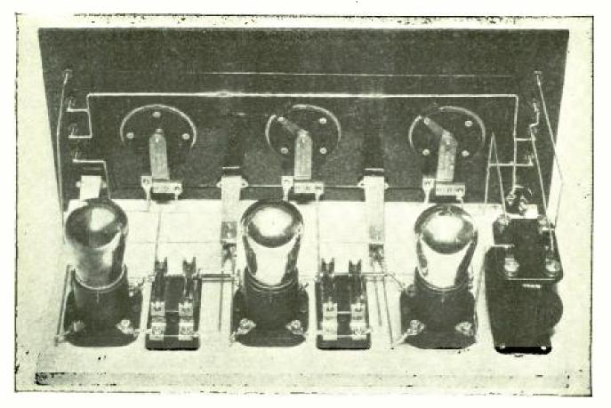
VIEW OF THE AMPLIFIER FROM THE REAR Compare this picture with the diagram on the next page when you mount the parts and when you connect up the instruments. The wiring is so simple that it can be done in a little less than an hour.
