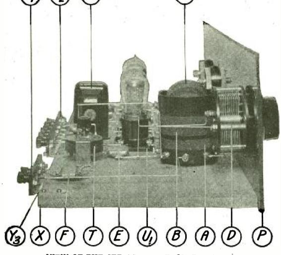
VIEW OF THE SET AS SEEN FROM THE LEFT FIGURE 6: This illustration shows the general manner of mounting the DX coupler, condenser and variable grid-leak.
