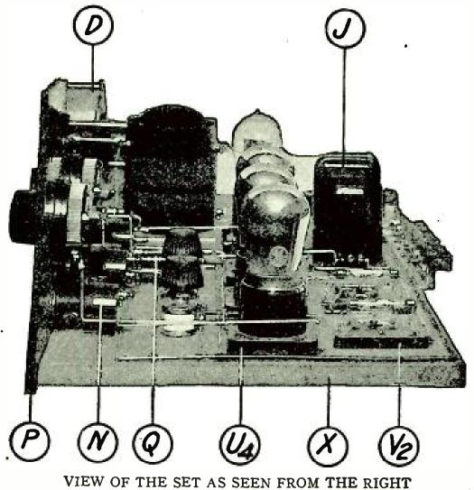
FIGURE 7: This end view indicates the manner of mounting the sockets, grid-leaks, Bradleyohms, rheostats and the jacks.
