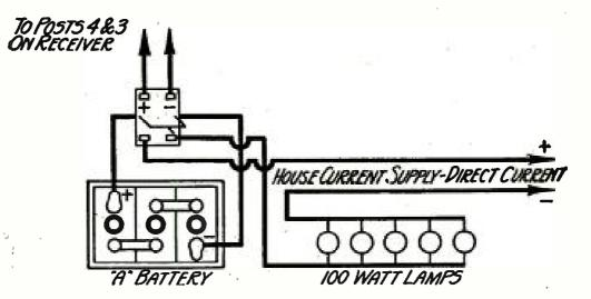
HOOK-UP FOR THE DIRECT CURRENT CHARGER FIGURE 6: When your house-lighting service is direct current, a different type of charger is needed, which is wired to the set as shown above. To determine the positive and negative terminals of your house current, dip leads from the supply line in a cup of salt water. Bubbles will form around the negative wire.
