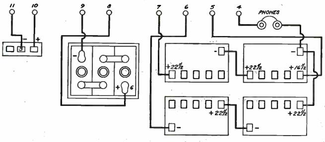
CORRECTED BATTERY HOOK-UP FOR THE SEVEN-TUBE SET FIGURE 2: The headphones are shown properly connected for the neutralizing process.
