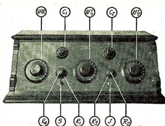
PANEL VIEW OF THE RECEIVER FIGURE 2: The three principal controls are VAR, variometer; RFT1 and RFT2, variotransformers; C1 and C2 are the compensating condensers; and R1, R2, R3 and R4 are the rheostat controls for the tubes. S is the jack switch and J is the filament control jack.
