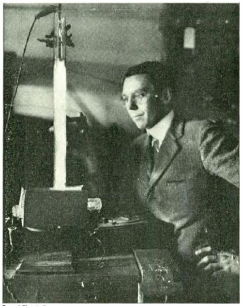
General Electric Co. HAS BALL LIGHTNING BEEN DUPLICATED IN THE LABORATORY? In this vacuum tube that contains a very small quantity of vaporized tungsten, Dr. C. G. Found has produced a "streamer discharge" that is said to be similar to the rare "ball lightning" that is observed in nature. An electric current acting upon the tungsten creates the atomic behavior that produces this phenomenon.
