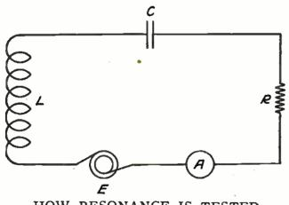
HOW RESONANCE IS TESTED FIGURE 6: In an electrical circuit, the frequency of oscillation depends on the inductance and the capacity. When generator E is run at varying speeds, some one speed will produce a frequency that will give the highest reading in ammeter A.
