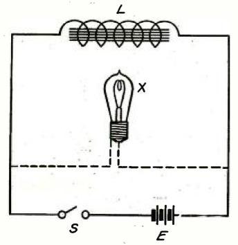
INDUCTION WILL LIGHT THE LAMP FIGURE 4: When key S is opened, the collapsing lines of magnetic force about the core of magnet L cut the wire of the magnet and induce a current that flashes the lamp.
