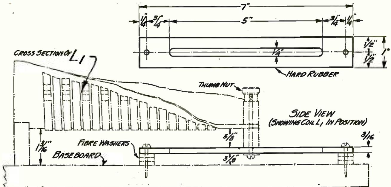
THE CONSTRUCTIONAL DETAILS OF COIL L1
