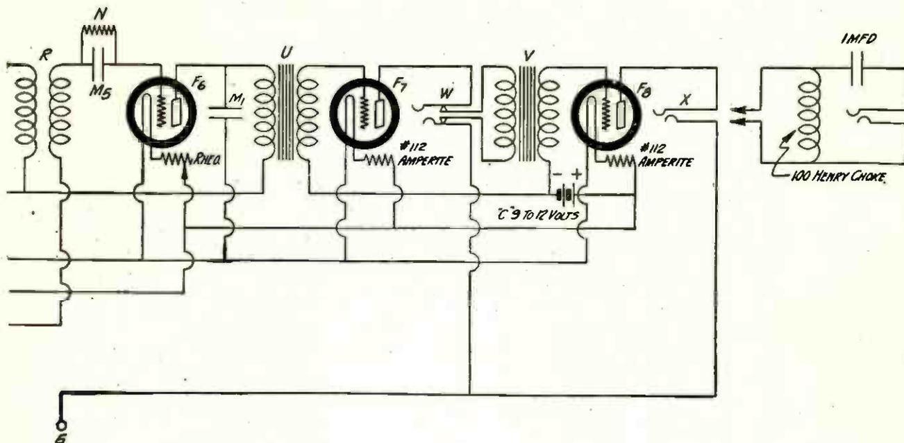
effected by connecting one side of a small midget condenser to the plate terminal of the detector tube, and the other side to the lower terminal of the loop.
