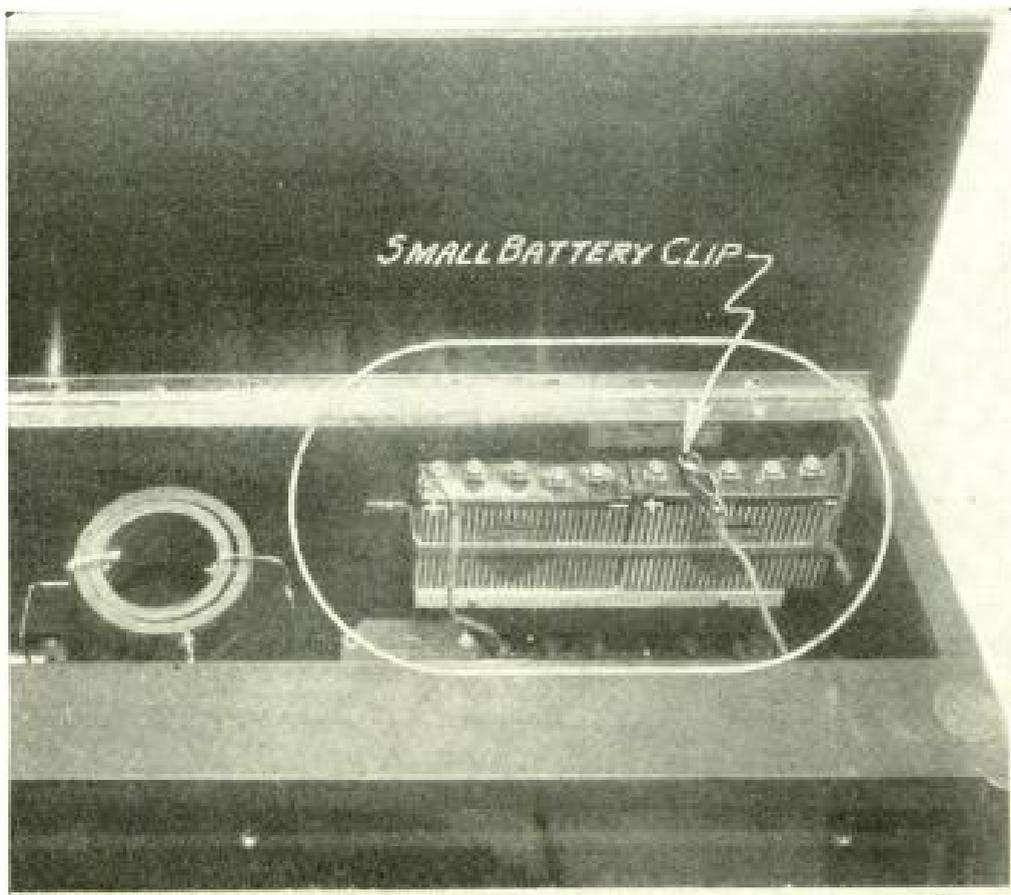
THE "C" BATTERIES INSTALLED IN THE CABINET
