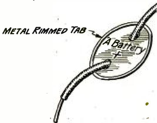
A MARKER FOR BATTERY WIRES
