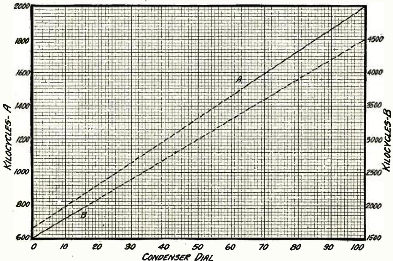
THE RESULT OF USING A 3:1 FREQUENCY RATIO CONDENSER ON A NARROW FREQUENCY BAND
