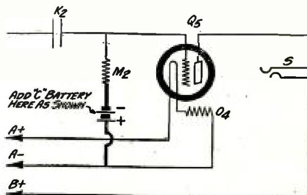
THE PROPER ELECTRICAL LOCATION OF THE "C" BATTERY
