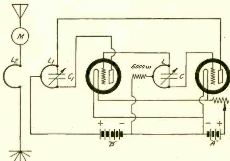
A DIAGRAM OF THE TRANSMITTER WIRING
