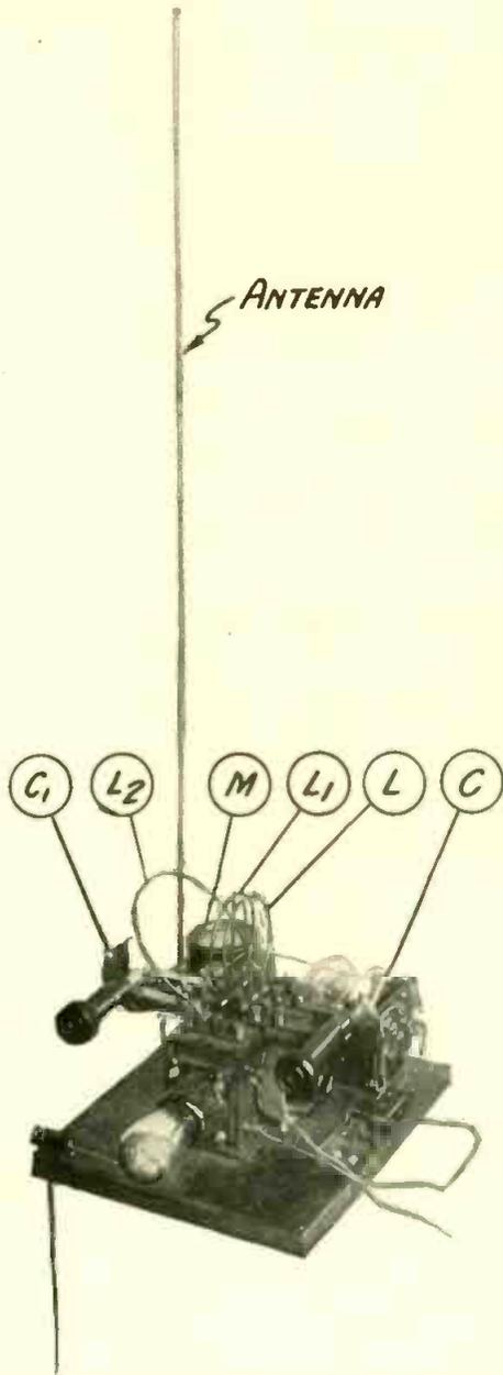
THE SHORT-WAVE TRANSMITTER USED IN THE EXPERIMENTS
