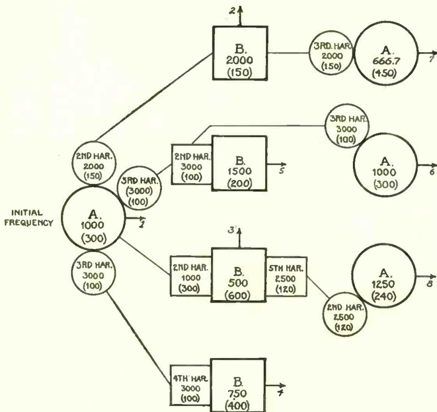
FIGURE 2: A general idea of how harmonic heterodyning is used to produce new frequencies should be easily obtained from this chart.
