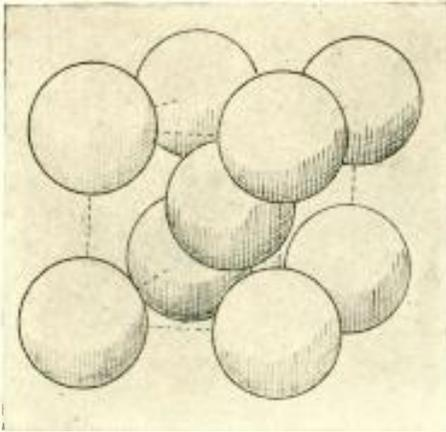
THE ARRANGEMENT OF ATOMS IN A PIECE OF IRON AT ORDINARY TEMPERATURES
