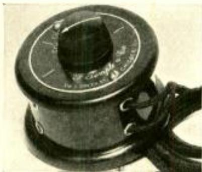
This small rotary switch is a quadruple-throw, double-pole rotary switch that contains pin jack terminals for loudspeakers. It will accommodate four sets of loudspeaker terminals at the same time and by rotating the small knob on the top of the instrument, any of the loudspeakers may be switched on instantaneously for direct comparison as to their tone qualities. Experimenters will find it a handy unit for connecting loudspeakers in circuit.
