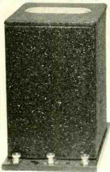
A SHIELDED RADIO-FREQUENCY COIL
