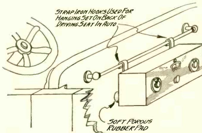
**ONE WAY TO MOUNT A RECEIVER IN AN AUTOMOBILE**
