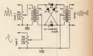
Fig. 5. Ring modulator. The output signal consists of  $f_1$  and  $f_2$  plus their sum and difference frequencies. The resulting sound is an unusual chord
