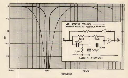
Fig. 1. Frequency response of parallel-T network
