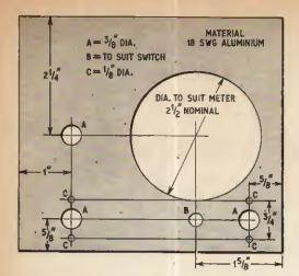
Fig. 10a. Front panel drilling details
