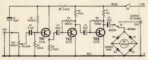
Fig. 9. Detector unit circuit
