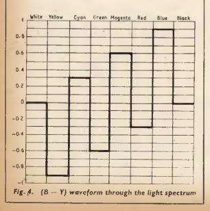
0.3r + 0.6g + 0.1b, the (R - Y) and (B - Y) is at zero level. Therefore, in the absence of the chrominance signals it is evident that the picture will be received in monochrome.
