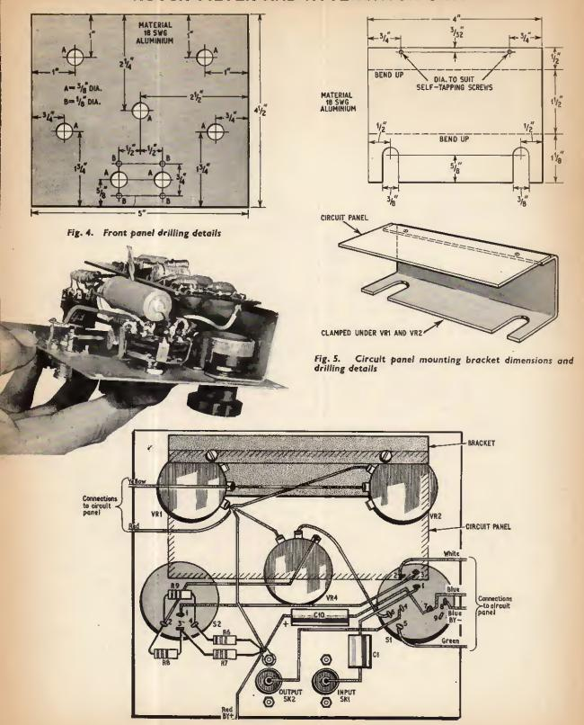
Fig. 6. Front panel controls and wiring
