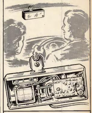
Overcome the irritating dazzle of night driving with this easy-to-build device. Mirror tilts upward immediately any bright light falls on a light-sensitive resistor.
