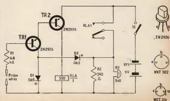
Fig. 3. Simple latching to overcome wave action
