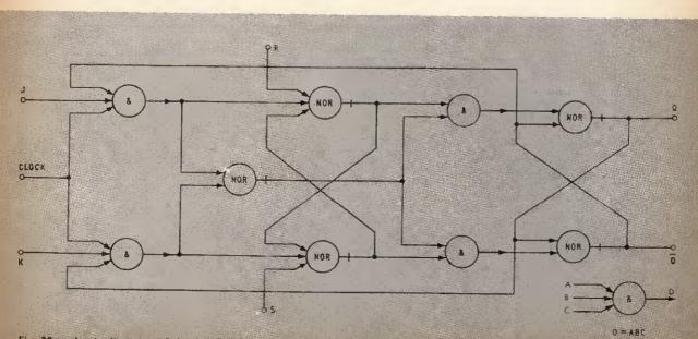
Fig. 20b. Logic symbol of an AND gate
