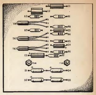
Fig. 11a. Circuit panel, component layout
