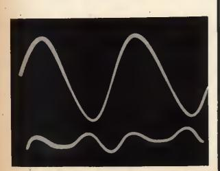
Fig. 13. Oscillograph of sine wave containing I per cent distortion. Lower trace shows distortion signal
