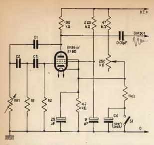
Fig. 3. Decay applied directly to a phase shift oscillator. The values of C1, C2, C3, VR1, R1, and R2 will depend on the frequency required. VR1 gives a fine adjustment of the nominal frequency
