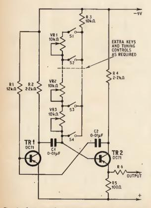
Fig. 4. A suggested transistor square wave generator tuned by adjustment of VRI, 2, and 3. Pitch can be selected by SI, 2, 3, 4
