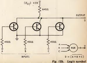
Fig. 15a. A typical RTL NOR gate
