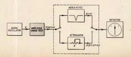
Fig. 2. Block diagram showing method of measuring distortion
