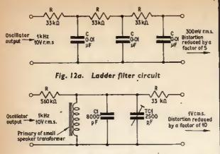
Fig. 12b. Inductive filter circuit
