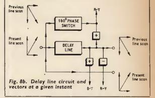
it is necessary to reintroduce the carrier component for demodulation, and this is the function of a crystal oscillator circuit, operating at 4.43MHz, and called the colour reference oscillator. Having reinserted the carrier the separated colour information is then demodulated and amplified as a video output signal. The (G - Y) content is determined from a proportion of the sum of (R - Y) and (B - Y), resulting in three colour difference video references which are fed to the c.r.t. grids.
