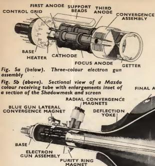
**CONVERGENCE ASSEMBLY**—Three pairs of plates act as internal extensions to external pole pieces of "Radial Convergence Magnets". Controls relative position of each electron beam.
