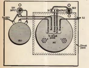
Fig. 10b. Front panel controls and wiring
