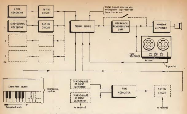
Fig. 8. Typical set-up for recording various tones and sound effects
