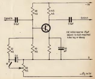
Fig. 2b. A suggested transistor decay circuit; prone to generating clicks when key SI is closed
