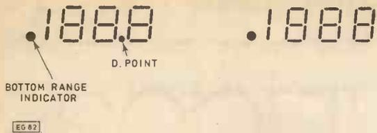
Fig. 1.14. Driver number 1 is an exception since the lowest range cannot be displayed as above left, so it is shown as above right bottom range indicator
