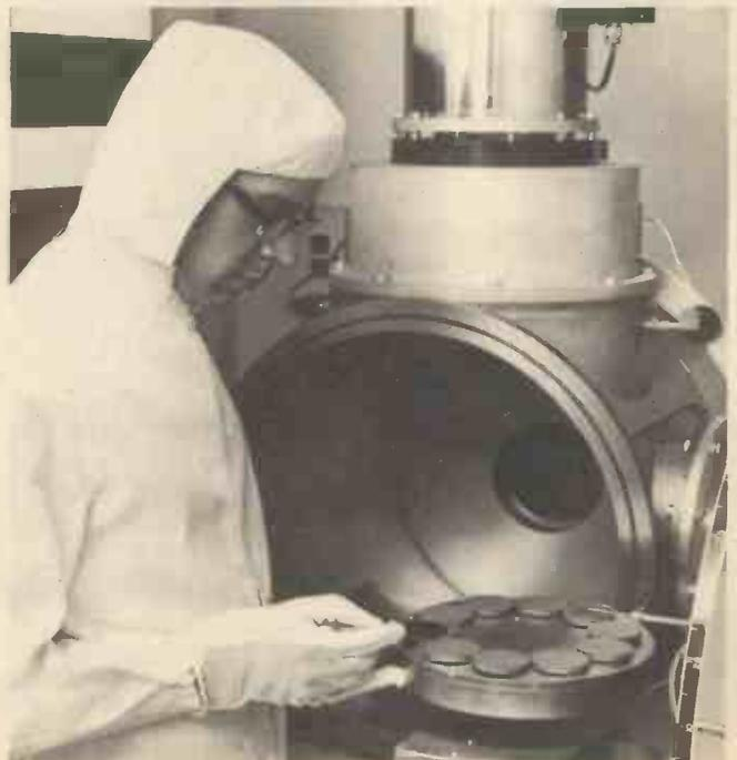
Fig. 10. Ion-milling equipment used to etch conductor and propagation patterns
