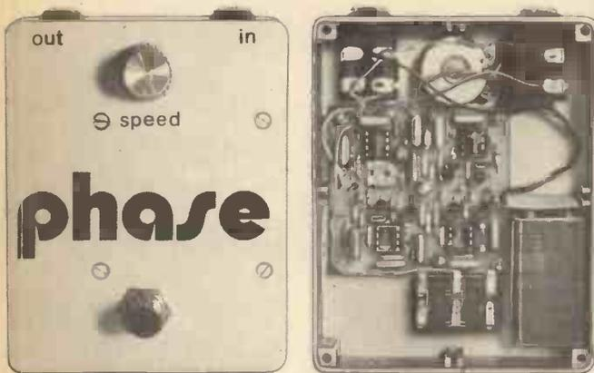
Front panel annotation and Internal layout of the Phaser unit
