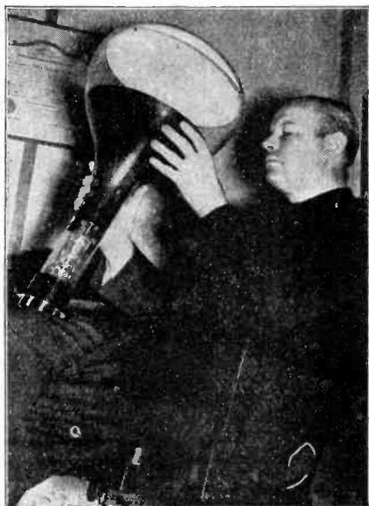
**T**HE more critical requirements of television reception are being met by two cathode-ray tubes recently developed and now made available by Allen B. DuMont Laboratories, Inc., of Upper Montclair, N. J. The Type 54-10-T has a 5-inch diameter screen and a maximum third anode voltage rating of 3000. The Type 144-10-T has a 6000-volt rating and a twelve-inch diameter screen.
