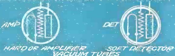
HARD OR AMPLIFIER VACUUM TUBES SOFT DETECTOR VACUUM TUBES
