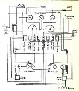
Fig. 7-Circuit Diagram of Power Equipment
