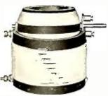
Tube of hard fibre, rotor in moulded hard rubber. Wound with green covered wire. Nickel plated hardware. Special binding posts. No soldering of connections.
