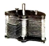
Variable condensers to be efficient must be well made. Loose joints or faulty construction soon allow the plates to get out of alignment and decrease their efficiency.
