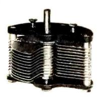
Variable condensers to be efficient must be well made. Loose joints or faulty construction soon allow the plates to get out of alignment and decrease their efficiency.
