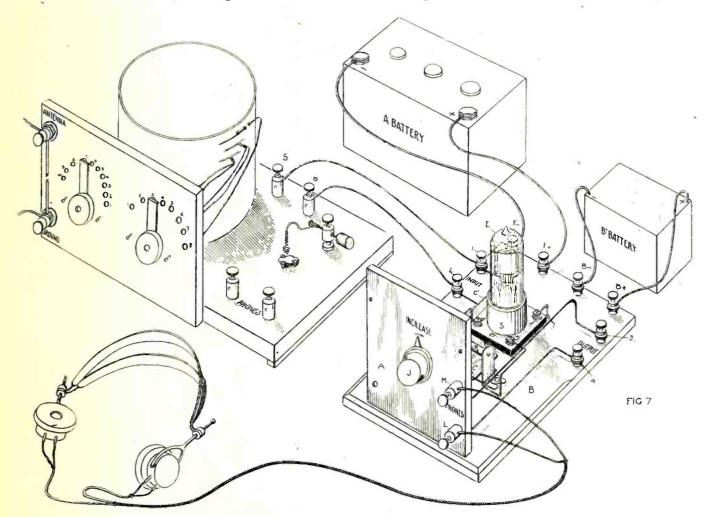
off two round wood blocks just long enough to raise the socket terminals clear of the base, and mounting them so that the screws which hold the socket to the baseboard will pass through holes in the centers of the blocks. After the socket, S, grid condenser C, grid leak R and by-pass condenser C' are mounted the parts are wired up.
