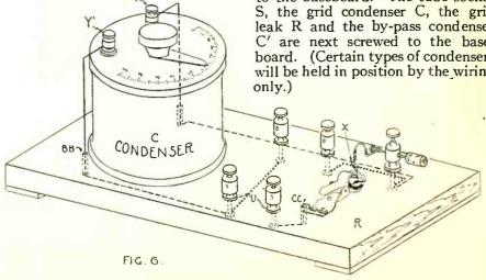
The exact location of these parts can not be stated because the several types of parts commercially available will vary somewhat in dimensions. One can get a very good idea of the relative positions of the several parts from Figs. 1, 2 and 7. The tube socket S is mounted so that the two terminals marked G and P (Fig. 1) are nearest the upright panel. Blocks Y and Y' are put under the socket S so that the four terminals of the socket do not touch the wood baseboard. This is done by cutting
