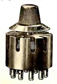
The amplitrol not only adjusts the filament to its maximum efficiency, but it also automatically switches on and off the plate circuit. Unlike automatic filament control, the amplitrol does not put a sudden strain on the filament. It provides a gradual current increase for the filament, prolonging the life of the vacuum tube at least one-third.
