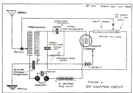
tinue to "stumble" onto more of inductance consists of the ordinary primary winding of the vario-coupler with its usual contact taps for the switch, with no change excepting that it will be noticed that a 43 plate variable condenser is conplicity of the arrangement, will at nected between this aerial inductance and the rotor. This gives a combination inductive and capacitative coupling between the two coils of the coupler.
