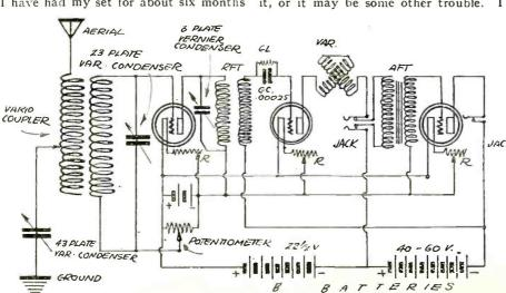
Figure 4. In the Three Circuit Regenerative set, the grid variometer is omitted when radio frequency amplification is added, and the tuning is accomplished with a 23 plate vernier condenser across the secondary of the variocoupler.
