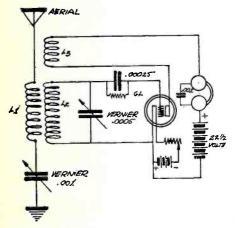
Figure 7. Many of our readers are asking for an easily constructed inexpensive one tube set. Here's one using two condensers and homemade inductances.
