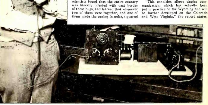
Radio station 9-CEX, with a range of from fifty to seventy-five miles. It was made by E. W. Applebaum, of the Illinois Fixture & Electric Supply Co., Chicago, and is said to be the smallest licensed and registered radio station. (U&U Foto).
