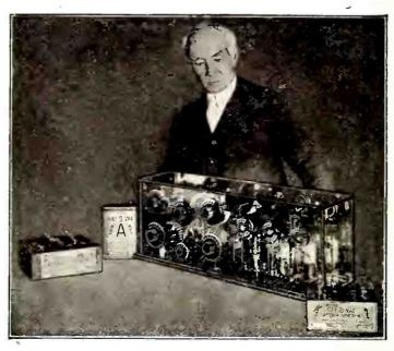
THE French Battery and Carbon Company has the distinction of having in its employ Chief Designer John Graves, who has conceived and built a radio receiving set of glass with two steps of audio frequency. The set operates with 3 WD-11 tubes on a Number 1261B Ray-O-Vac "A" Battery and 3 No. 2151 Ray-O-Vac "B" Batteries on the plate circuit.
