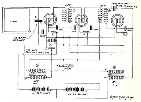
Figure 2. The finished hookup of the Grimes Circuit.
