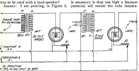
Figure 3. A two stage audio frequency amplifier, constructed with binding posts as in the circuit, can easily be connected to any set, as shown.
