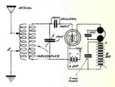
drawing will help considerably. As the condenser used for this purpose has too much capacity to be used across the phones, it will not do to employ the one condenser for both, but two separate condensers of the proper capacities should be used as shown.
