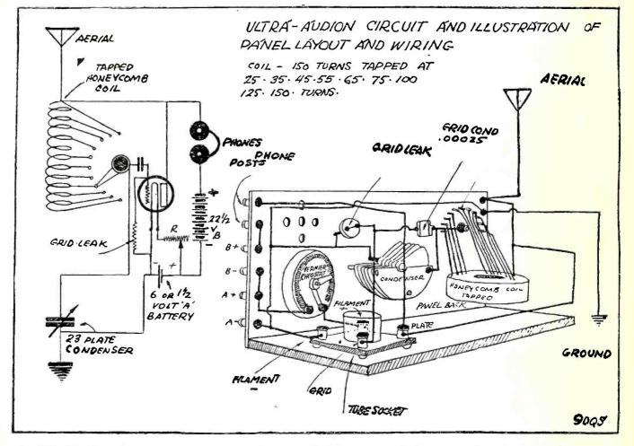
O NE OF the oldest and most efficient tube circuits evolved in the course of vacuum tube experimentation is the Ultra Audion circuit, which during the years of its use has not changed appreciably, and which remains one of the most efficient single circuit systems now in use.
