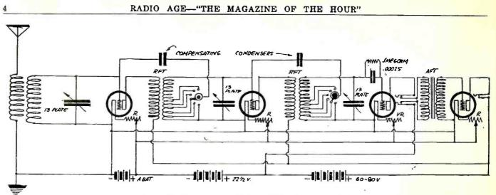
Figure 3. Complete circuit diagram of the Neutrodyne set.
