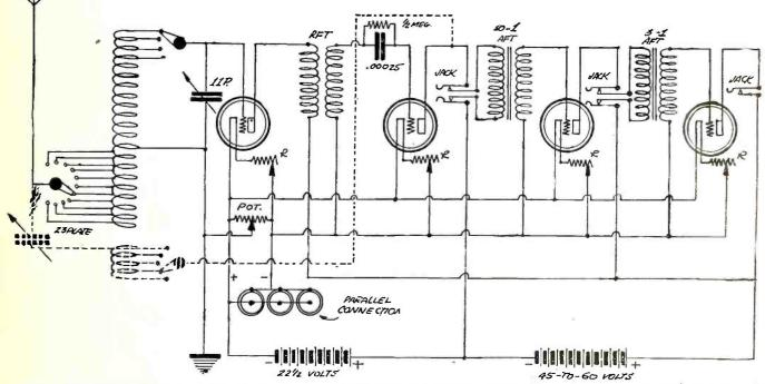
Figure 1. This is the Reinartz circuit, showing how Mr. Tuck changed the circuit by taking out the plate coil. This is indicated by the dotted lines.
