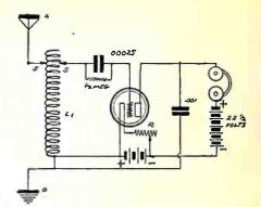
Figure 4—The two-slide tuning coil is connected to a tube much in the same way as a crystal is used.
