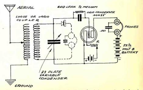
Figure 6—The dotted lines in the above circuit show the relative connections of tube and crystal in the two-circuit set.
