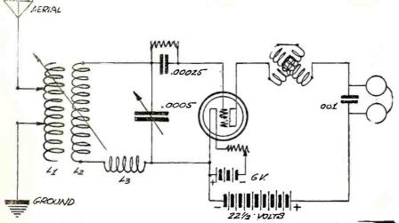
Figure 5-This is circuit used when the long distance crystal set is changed to a tube set.
