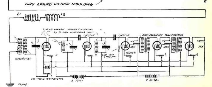
Figure 2. This composite sketch shows Mr. Leland's arrangement of using the picture moulding oatmeal box antenna. Ll is a coil wound on an oatmeal box, having 25 turns and L2 is a coil of the same number of turns, wound on the same box in the opposite direction from L1. The circuit shown, while not of the type used by Mr. Leland, is a type of circuit particularly admitted to the experiment
