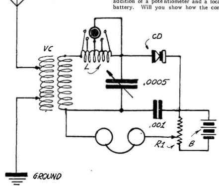
Figure 5. This shows the electrical connections of a sharp tuning crystal set, making use of a potentiometer and local battery to increase the efficiency of the crystal. VC is the variocoupler, L is a coil of 25 turns, tapped every fifth turn, CD is the crystal rectifier, and RI is a potentiometer of the graphile type, having a maximum resistance of 10,000 ohms. The battery marked B should have a voltage of from two to four volts.
