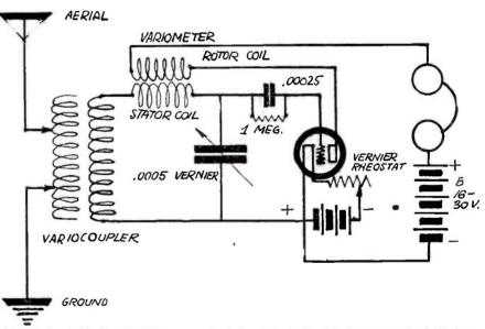
Figure 1. This is another arrangement possible, using the instruments of the longdistance crystal set in a one-tube hookup. The variometer is split and used in the circuit as shown. The set is highly regenerative and gives unusually loud signals.
