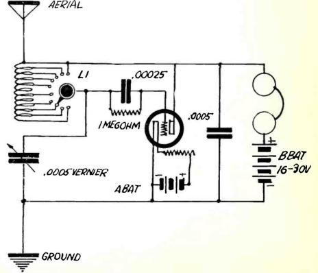
Figure 1. This shows the circuit constructed by one of our readers, which is giving unusual results. L1 is a spider web coil, having 10 taps, with taps at every seventh turn, making the coil 70 turns in all.
