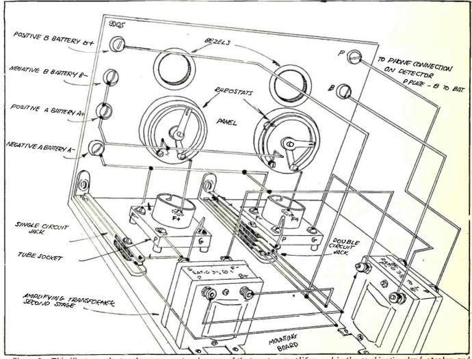
Figure 5. This illustrates the panel arrangement and wiring of the two-stage amplifier used in the combination loud speaker and amplifier described on page [3. Full instructions concerning the construction of this unit appeared in the August issue of RADIO AGE.
