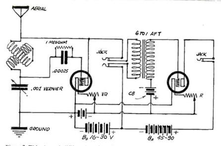
Figure 2. This shows the "First Tube Outfit" connections with the addition of a one-stage audio frequency amplifier. CB is a small flashlight ballery, or dry cell, of one and one-half volts used as a grid bias, to assure the highest amplification factor when WD 11 tubes are used. L is the variometer. Full details concerning this set were given in the October issue of RADIO AGE.
