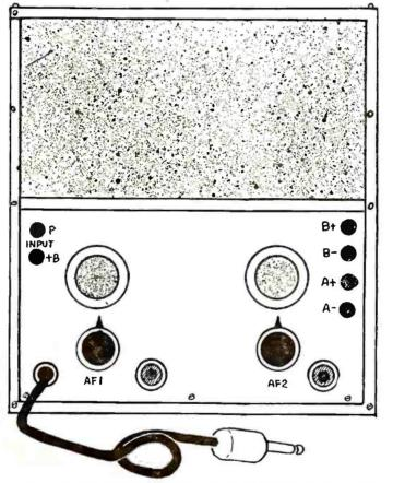
Figure 1. This is the front panel view of the neat-appearing, loud speaker and two-stage amplifier, described by Mr. Masson.
