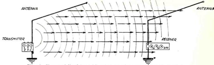
The magnetic lines being at right angles to the electrical wave travel in a horizontal plane.
