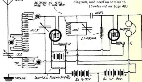
Figure 3. The Reinartz circuit in connection with the tuned impedance radio frequency method of low frequency amplification. This method is highly efficient in tuning over a broad hand of waves.
