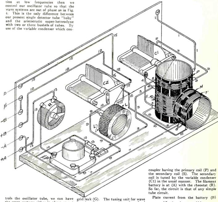
the wave systems either in phase or out of phase at pleasure, hence we can use the circuit as a plain heterodyne or superheterodyne at will.
