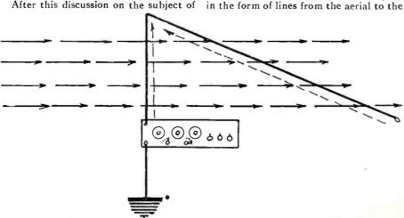
Figure 7. Wrong construction of antenna. The lines cut in such a manner as to set up opposing currents.
