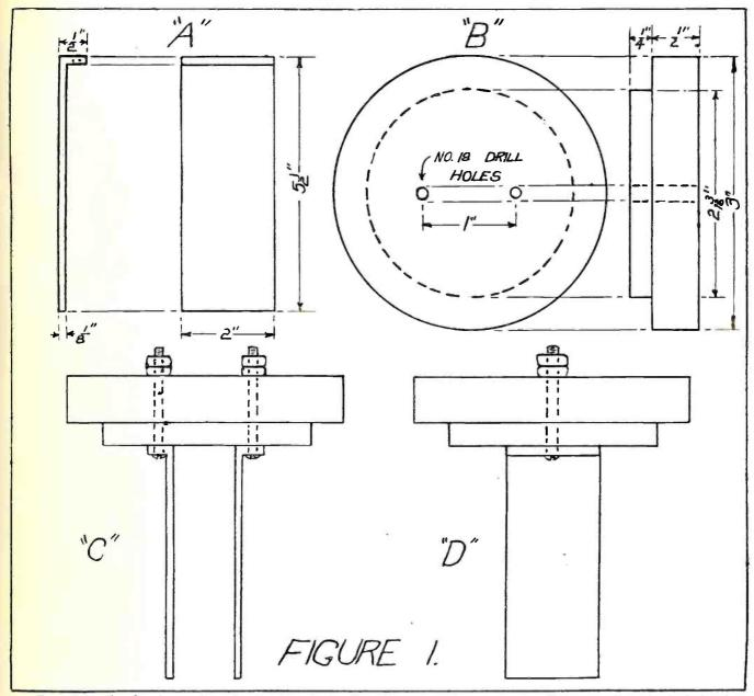
The constructional and assembling details of the Noden Valve Electrolytic Battery charger. This type of rectifier is designed for use in homes where the 110 volt house lighting current of the alternating type is available.
