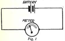
arises as to how an electric current can flow in an open circuit. It is true (in the case of direct or continuous currents) a complete conducting circuit must be supplied before a current will flow and when such a curciut is established, the amount of current flowing will depend upon the electrical pressure applied and the electrical resistance of the circuit.
