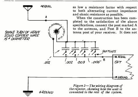
sandpapered, and soldered rigidly to the copper strips which are cut from the ten inch piece of copper. The illustration shows how this is accomplished. The slider, constructed from the brass strip, should next be drilled and mounted so as to run smoothly over the entire arc. Drill for the mounting of the switch levers, and switch points and make allowance for the two binding posts. Two switchpoints must be used, one to throw the condenser into the circuit and the other out.
