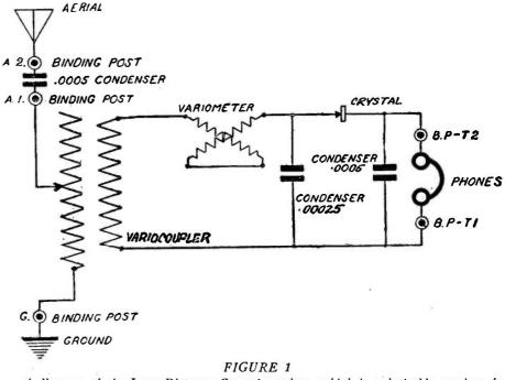
A diagram of the Long Distance Crystal receiver, which is a desirable receiver for the new beginner in the radio pastime. The set is easily constructed, requires little or no knowledge of radio, and gives surprising results. The binding posts, A-1 and A-2, are used as part of the tuning system, the A-2 post being used for the lower waves and the A-1 for the higher. This applies especially where the antenna used is a long one.
