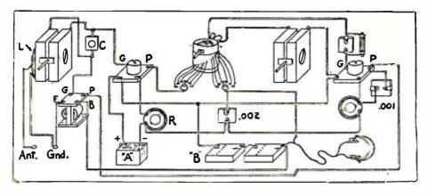
stituted instead. Many reflex circuits show a large fixed condenser across the "G" and "F" posts of the transformer, but the experience of the writer is that this is poor practice in a single reflexed tube. It acts as a shunt condenser and lowers the voltage of the energy released from the secondary winding, thereby reducing the volume very noticeably.
