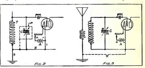
trouble with body capacity if a sufficient potential is established on the grid by regeneration. If the grid line is connected to the stationary plates or stator (S), then all parts at grid potential will be located well back of the panel and the tendency toward body capacity on the controls will be reduced by this amount. Again, connecting the stator to the grid allows us to connect the rotor to the ground or to (-A), which still further protects against trouble.
